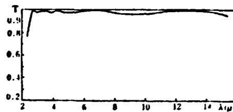
Fig. 2. The calculated transparency curve of a three-layer broad-band antireflection coating system.
