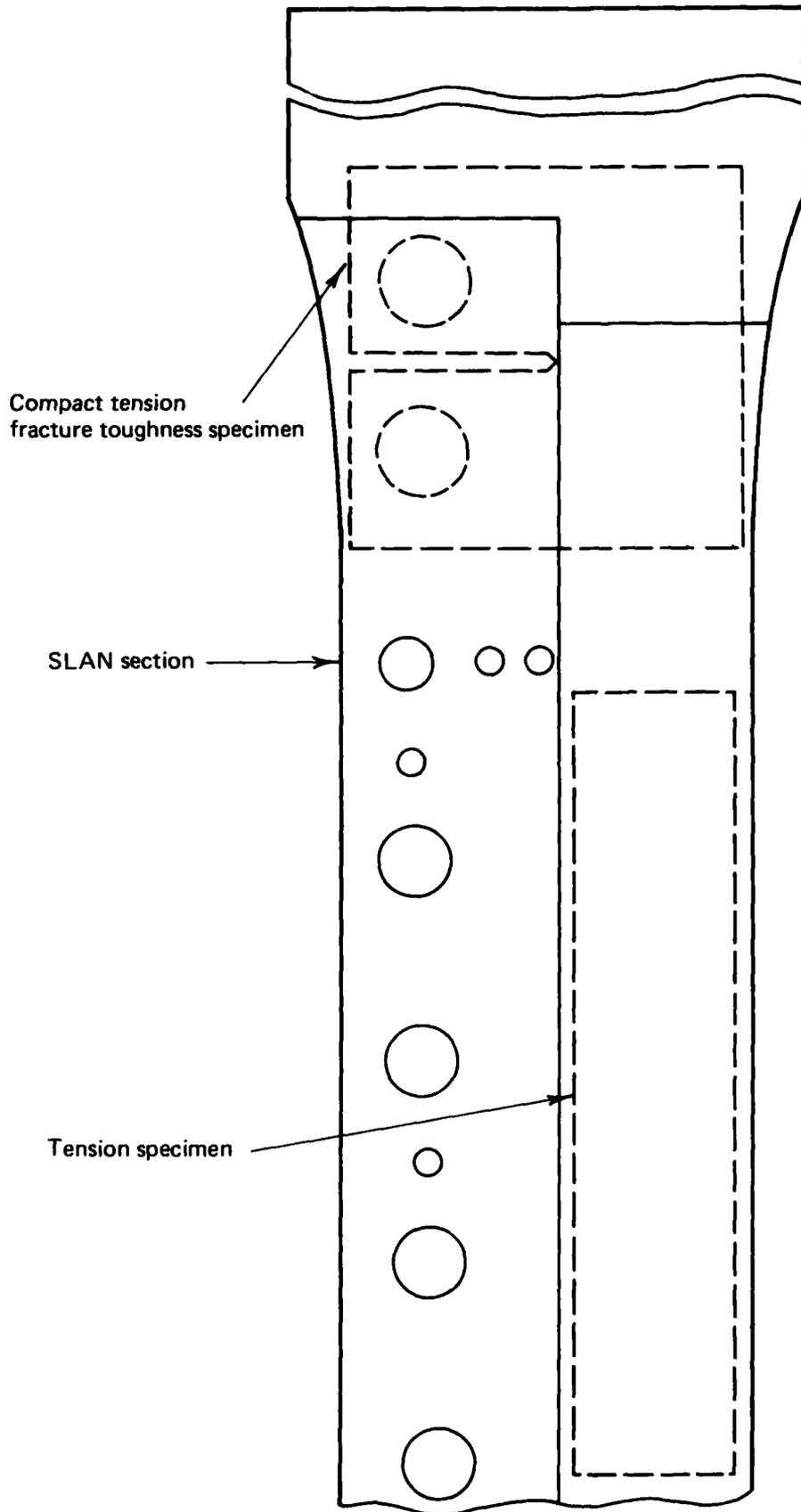
FIG. 11 LOCATIONS OF TENSION AND FRACTURE TOUGHNESS SPECIMENS
