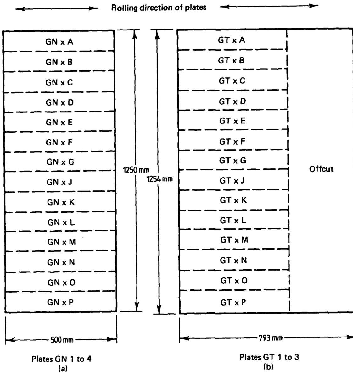
FIG. 9 FATIGUE SPECIMEN POSITIONS IN A7- U4SG PLATE
