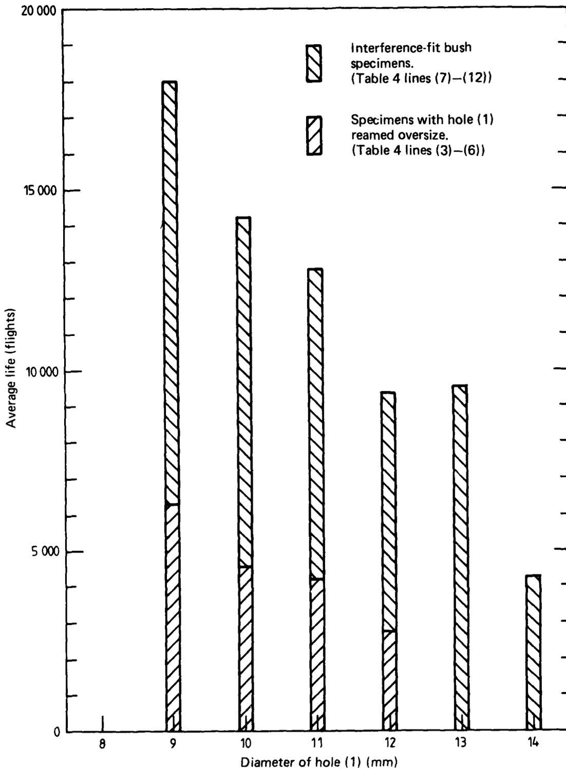
FIG. 22 COMPARISON OF LIVES OF SPECIMENS WITH INTERFERENCE-FIT BUSHES TO LIVES OF SPECIMENS WITH HOLE (1) REAMED OVERSIZE
