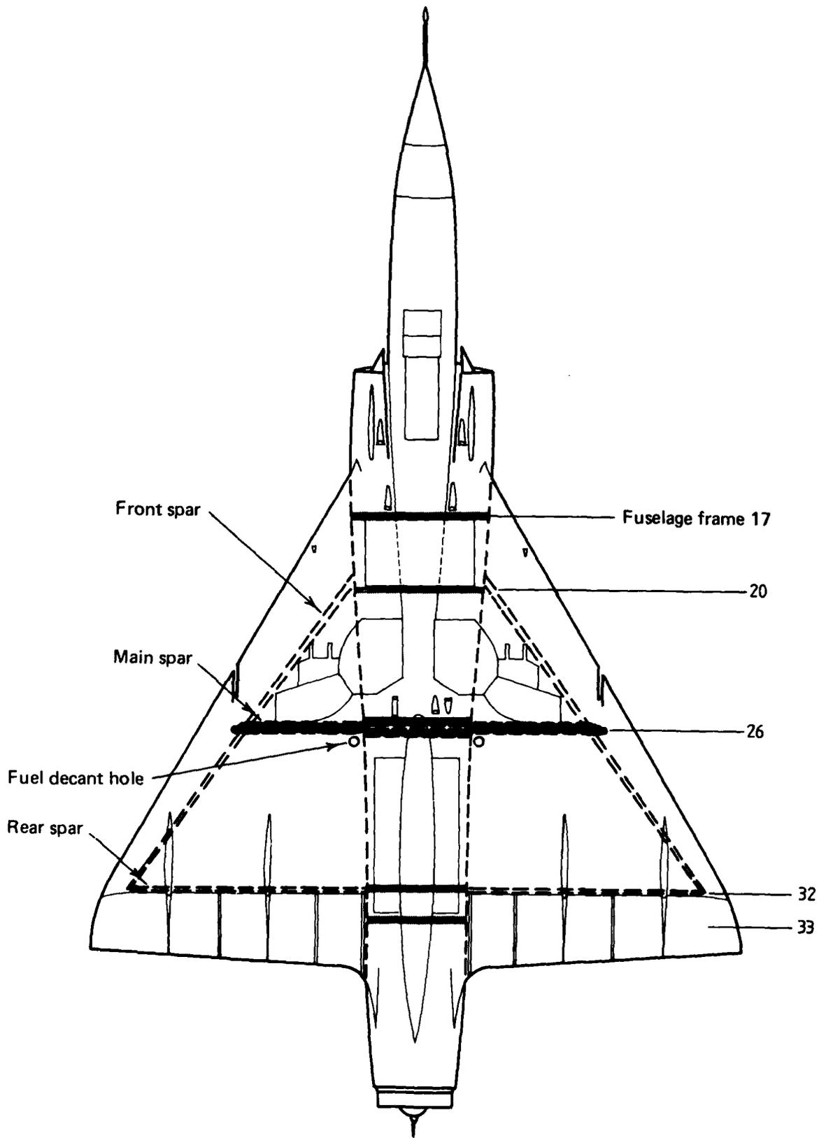
FIG. 1 MIRAGE III LOWER SURFACE SHOWING POSITIONS OF WING SPARS
