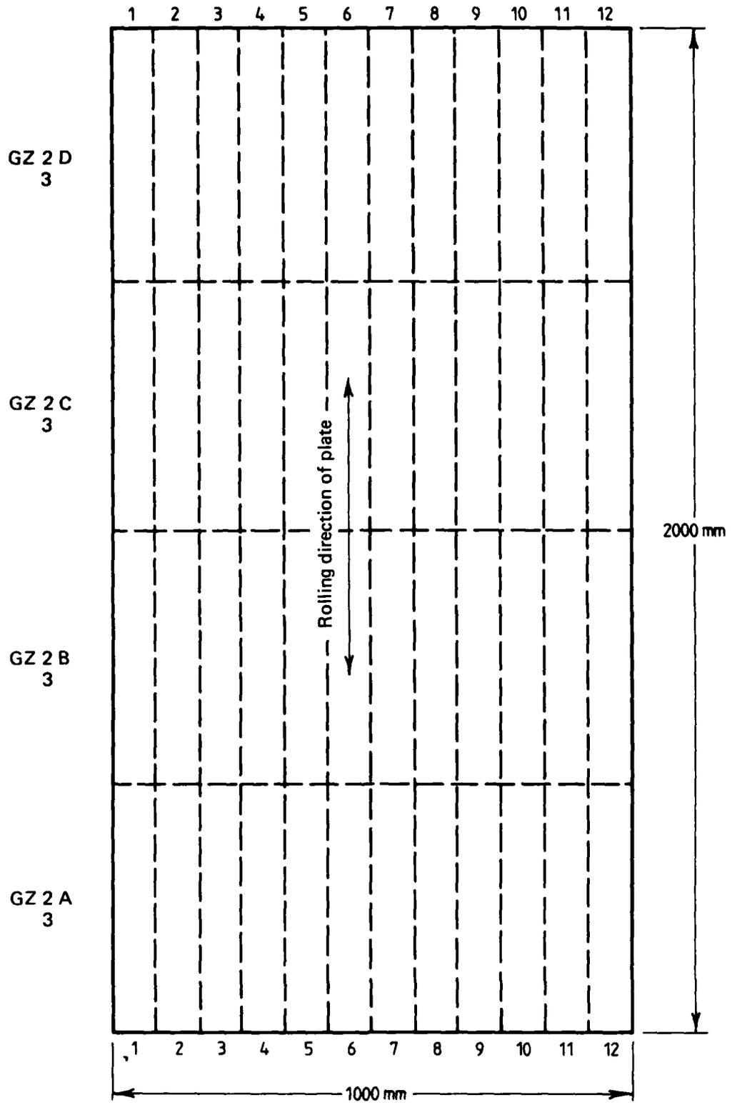
FIG. 10 FATIGUE SPECIMEN POSITIONS IN A7- U4SG PLATES
