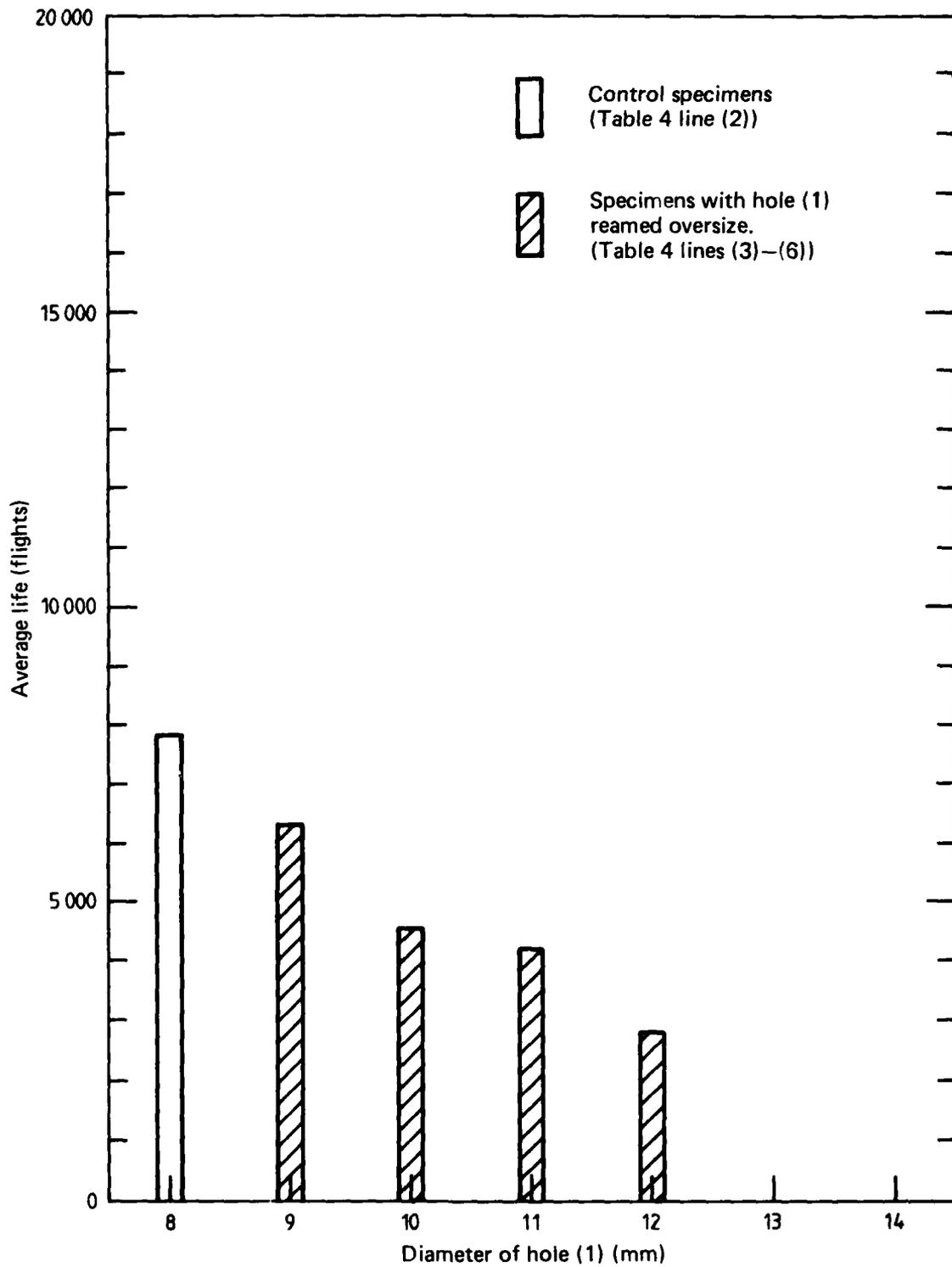
FIG. 15 COMPARISON OF LIVES OF CONTROL SPECIMENS TO LIVES OF SPECIMENS WITH HOLE (1) REAMED OVERSIZE.
