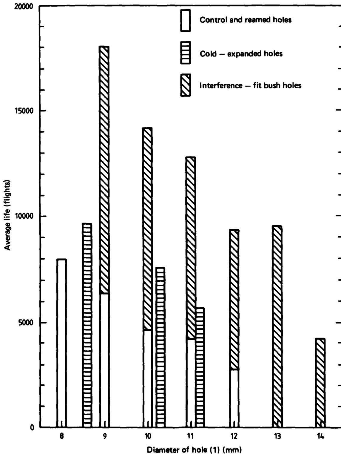
FIG. 36 EFFECTIVENESS OF BOLT HOLE REFURBISHMENT TECHNIQUES
