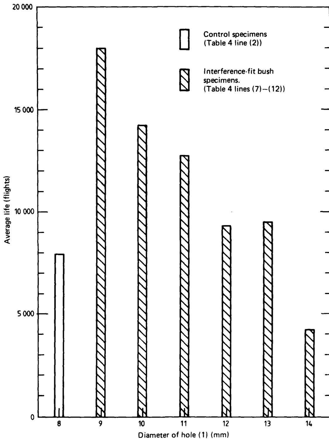
FIG. 21 COMPARISON OF LIVES OF CONTROL SPECIMENS TO LIVES OF SPECIMENS WITH INTERFERENCE-FIT BUSHES
