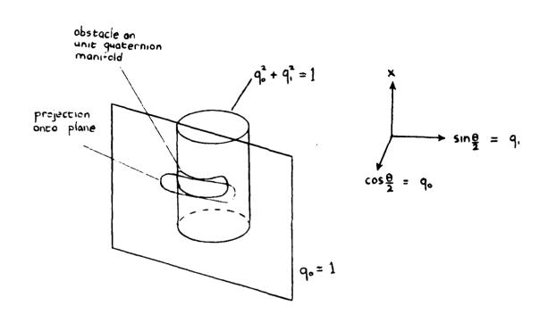
Figure 1. Projection of a configuration space constraint from the cylinder of normalized quaternions onto a hyperplane.
