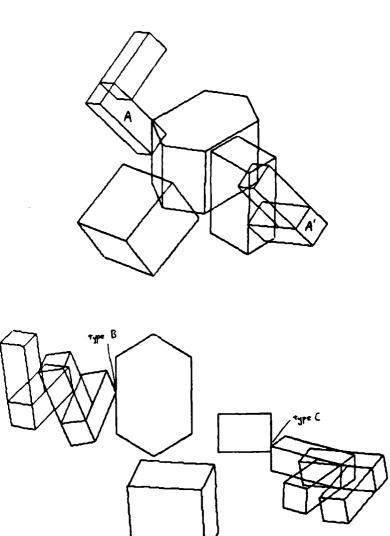
Figure 2. Collision Detection Example, (i) Object starts at A, moves uniformly to A', (ii) collisions points along the path
