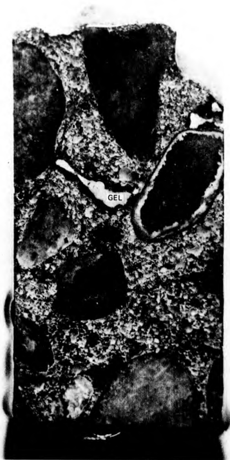
Figure 12. Photograph shows evidence of alkali-silica reaction, i. e. gel pockets and cracks traced in reaction products. Thin section blank, core 5-1, 7.5- to 9.0-ft section, Tuscaloosa Lock (after McDonald and Campbell 1977)
