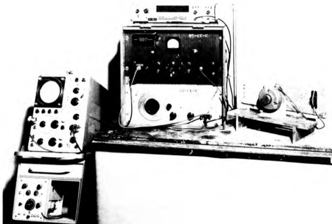
Figure 22. Laboratory resonant frequency vibration apparatus
