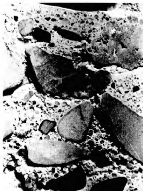
Fig. A.3.1—Bleeding channels and water pockets of concrete in a caisson; note laitance below particles of coarse aggregate
