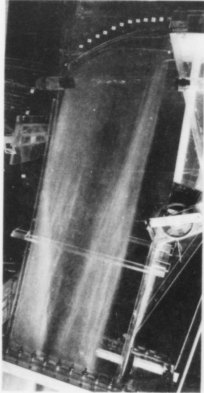
Valve open 12.5 ft; discharge 13,900 cfs. emergency gate slot vent open.
