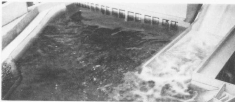
River discharge 45,000 cfs, spillway flow 40,000 cfs.
