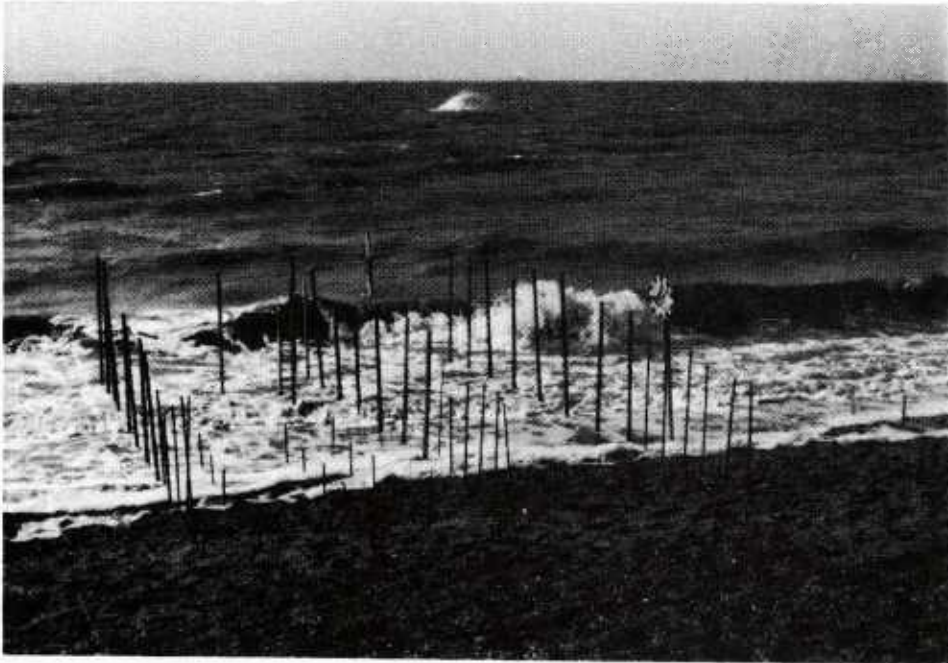
FIGURE 5 PHOTOGRAPHS TAKEN BEFORE HIGH TIDE SHOWING COYOTE POINT FIELD SITE AND SURVEYED ARRAY OF REFERENCE STAKES
