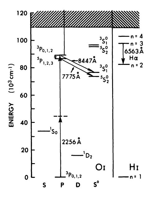
Figure 1. Partial Energy Level Diagram for O and H Atoms
