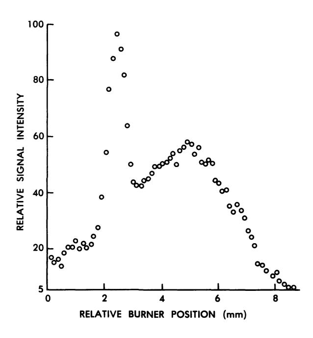
Figure 3. O Atom Emission Profile at 777.5 nm in a Curved Knife-Edge Burner Supporting a Fuel-Rich  $\text{CH}_4/\text{N}_2\text{O}/\text{N}_2$  Flame
