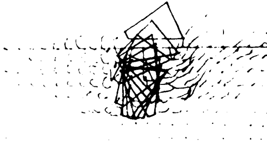
Fig. 4 Movement of the paddy soil particles under the action of a single lug with slippage 25%
