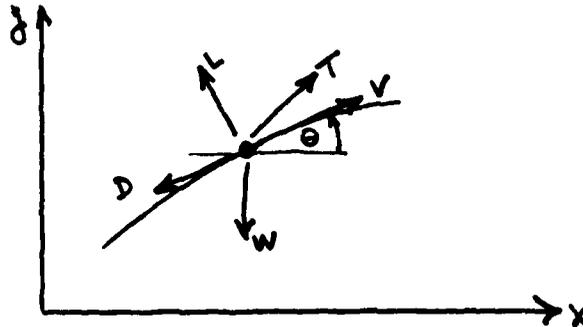
The forces acting are the Thrust ( $T$ ), Lift ( $L$ ), Drag ( $D$ ) and Weight ( $W$ ). The thrust is at an angle  $\alpha_e$  above the fuselage reference line; the fuselage reference line is at an angle  $\alpha$  above the velocity vector ( $V$ ); and the velocity is at an angle  $\theta$  above the horizontal x axis. The pitch attitude ( $\psi$ ) is given by
