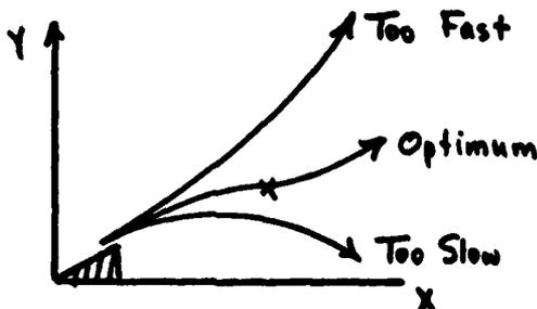
Generally, larger ramp angles also provide the desirable smaller launch speeds. However, there is a complicated interplay that must be considered among logistics, launch speed, ski-jump angle and aircraft loads. Also one must consider the sensitivity of the results to small errors in thrust and speed to provide adequate margins of safety.
