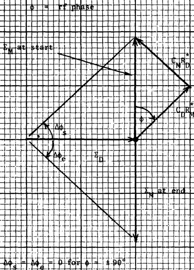
Fig. C-10. Relation of various phasors for simultaneous two source commutation at separation angle = 0.5 beamwidths.
