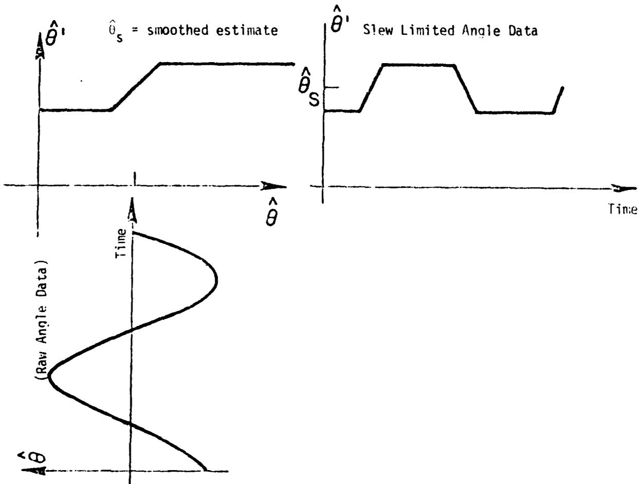
Fig. 5-3. Input-output time waveforms with TRSB Phase II receiver slew limiter.
