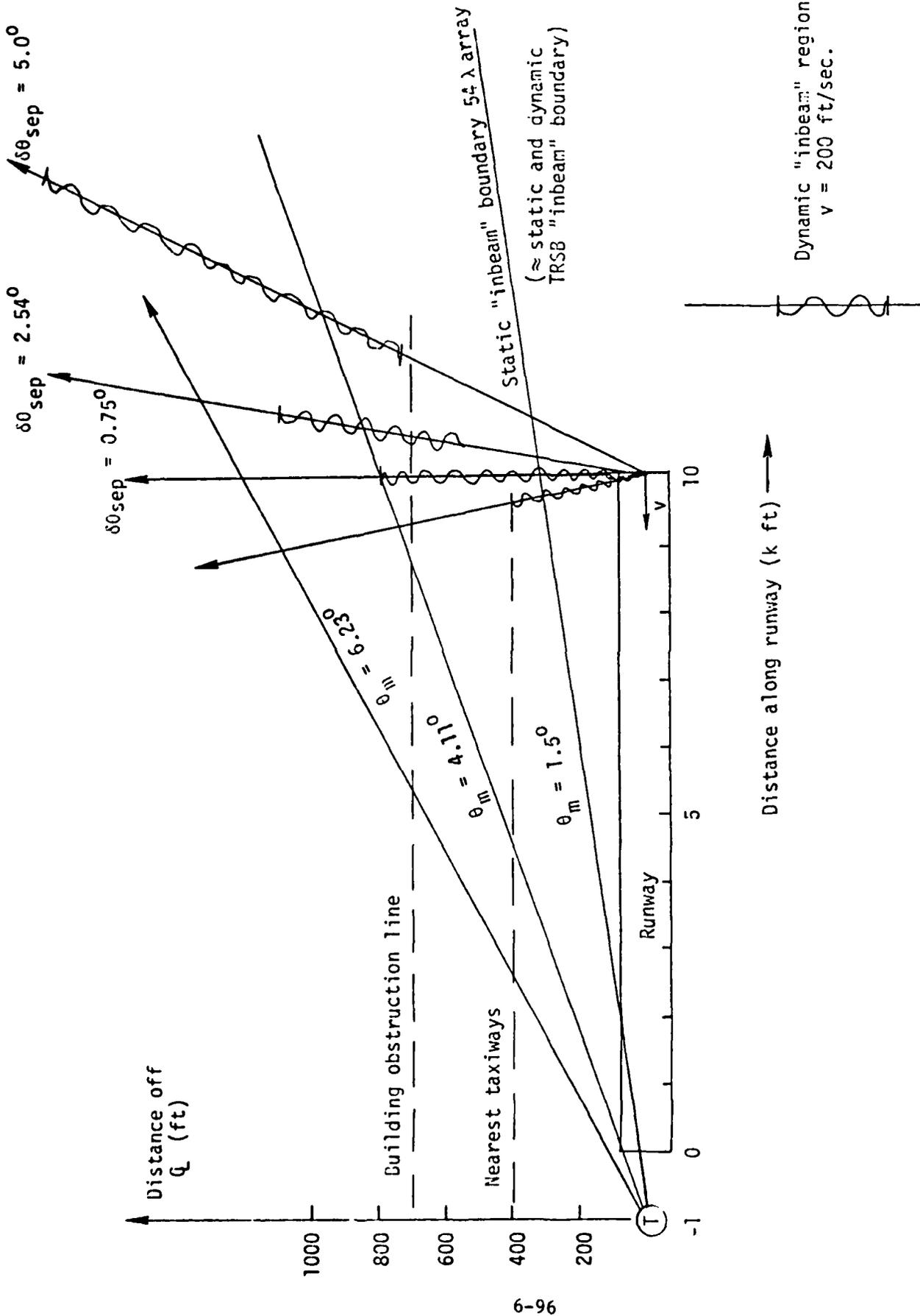
Fig. 6-31. Dynamic DMLS "inbeam" multipath region for reflected array x direct reference component.
