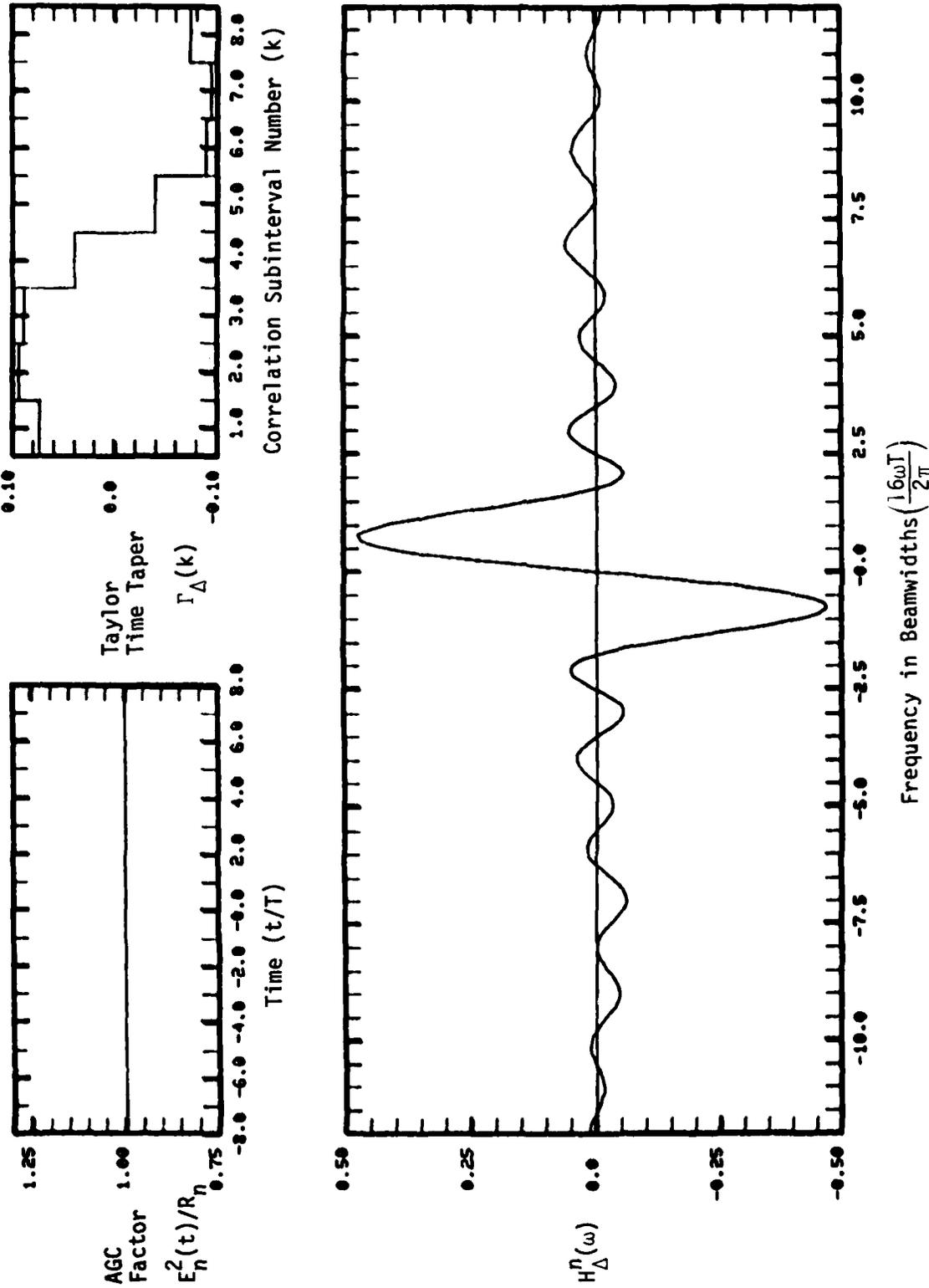
Fig. 6-2. Difference filter frequency response for zero scalloping frequency (uniform AGC factors).
