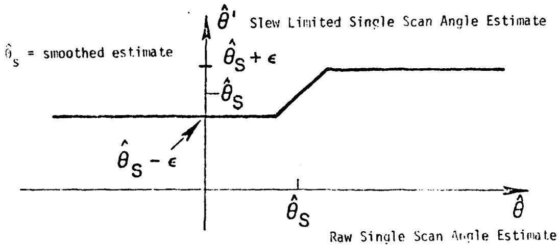
Fig. 5-2. Input-output characteristic for slew limiter.
