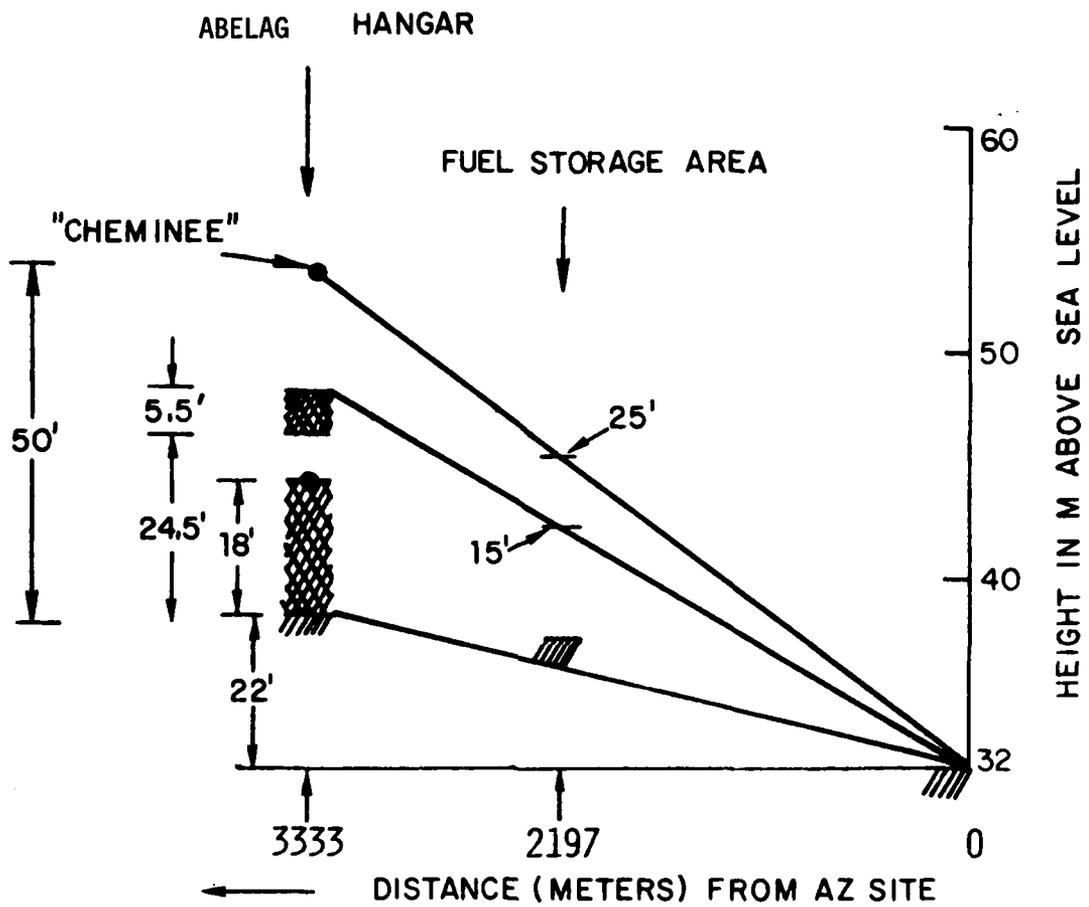
Fig. 6-52. Vertical plan view of Abelag hangar shadowing by fuel storage area structures.
