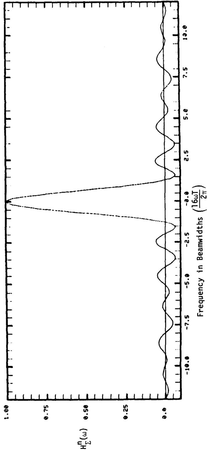
Fig. 6-3. Sum filter frequency response for scalloping frequency of  $\frac{1}{2} \frac{2\pi}{16T}$  (210 Hz) and midscan phase of  $0^\circ$ .
