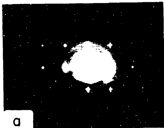
TED Pattern After Annealing at 250°C for 15 Minutes
