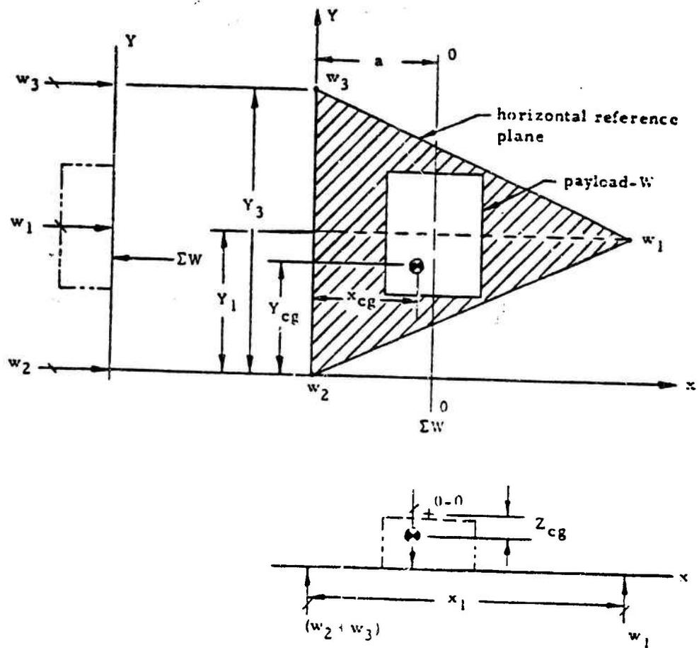
Figure 3.2 Horizontal Reference Plane Projection to Illustrate Method of Locating Center of Gravity by Weighing Test Object in a Single Plane
