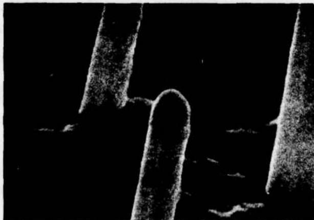
Figure IV-10. Scanning Electron Micrograph of Ion Milled Exposed Fibers.
