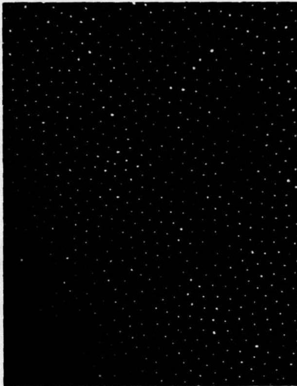
Figure III-10. Photomicrograph of Transverse Section of Sample LBH-20 Showing Tungsten Fiber Array, X542.
