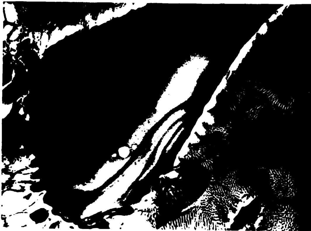
Fig. 11 TEM micrograph of an unmelted Al<sub>3</sub>Ni intermetallic particle surrounded by the microeutectic mixture corresponding to zone A.
