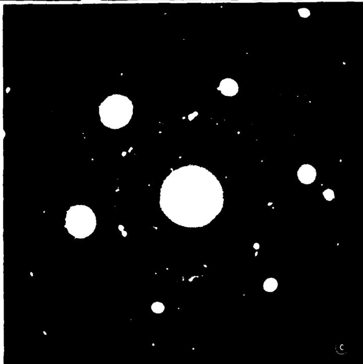
Fig. 36 a) Transmission electron micrograph of the top surface of ribbon of Al-8Fe-2Mo made in vacuum. b) SAD pattern of the above structure.
