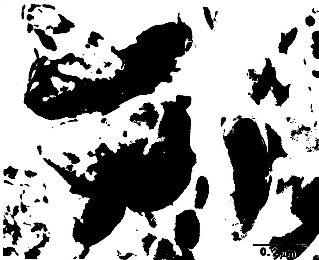
Fig. 7 TEM micrograph of Al-3.5at.%Co melt spun ribbon spun in vacuum showing zone B microstructure.
