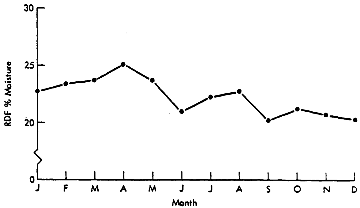
Figure 4-3. Monthly Average RDF Moisture and Heating Values at Ames Municipal Power Plant - 1976 4 .
