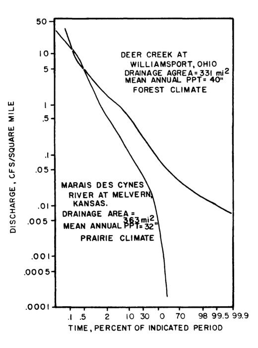
Figure 2.8. Flow-duration curve of mean daily flows for each of two rivers: Deer Creek at Williamsport, Ohio, and Marais des Cygnes River at Melvern, Kansas (from Leopold *et al.* 1964: Fig. 3-18).
