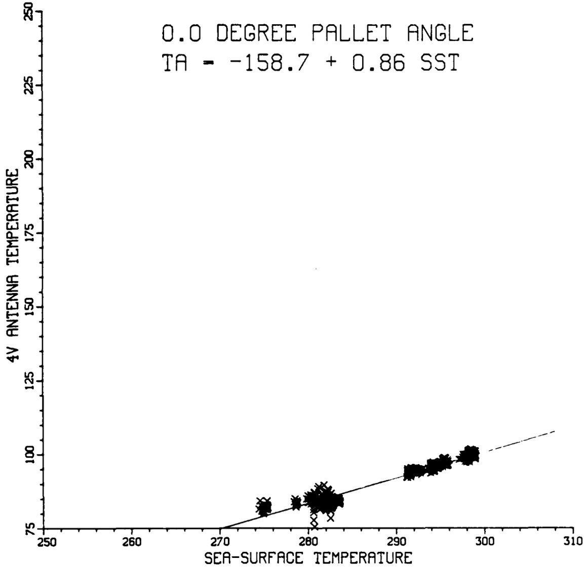
Figure 5 SFMR 4.5 GHz antenna temperature vs SST at 0° pallet angle
