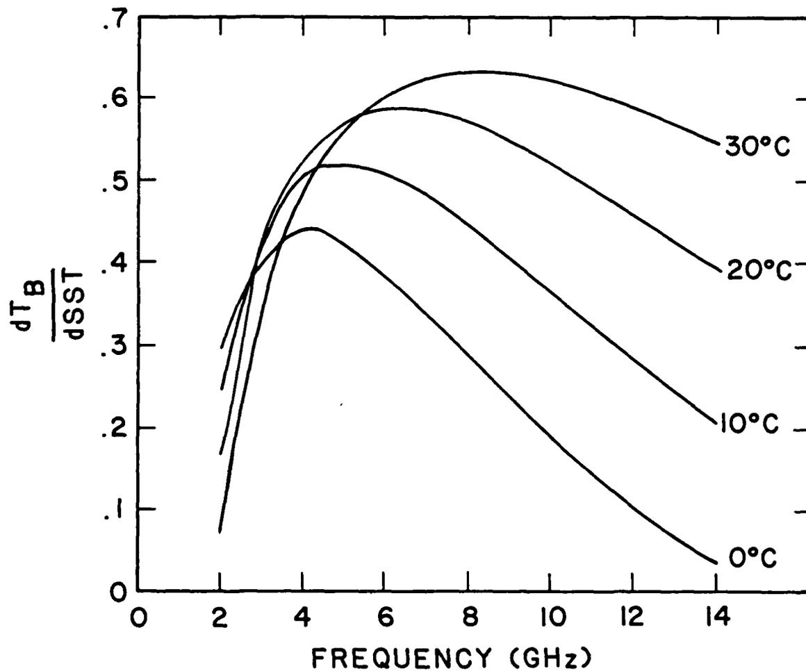
Figure 1 Sensitivity of brightness temperature to SST as function of frequency
