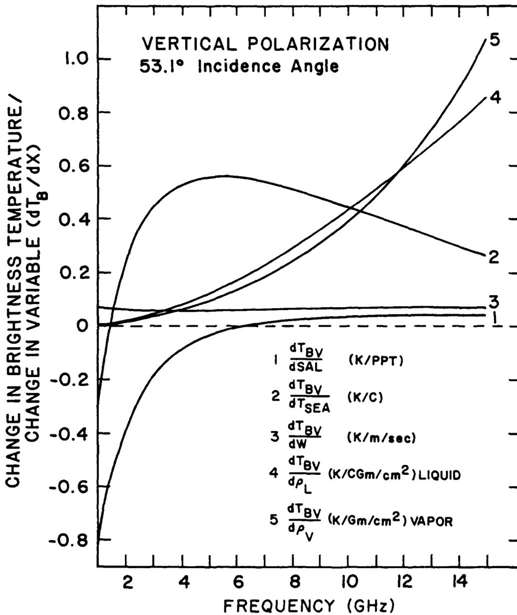
Figure 2 Change in brightness temperature w.r.t. change in environmental parameters
