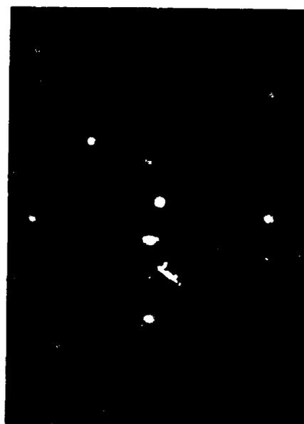
FIG. 2. LEED photograph of the  $c(6 \times 2)$  structure of the ( $\bar{2}01$ ) layered face of the GeAs crystal used in this study for 100 eV primary electrons.
