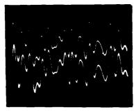
Figure 20. Two Broadband Waveforms on Electrodynamic Shaker
