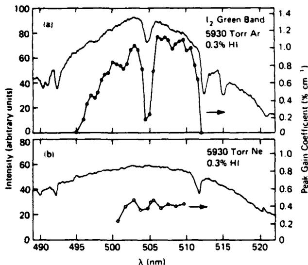
FIG. 4. Spontaneous emission and gain spectra for electron beam excited mixtures of HI and (a) argon or (b) neon. The minimum detectable gain coefficient is  $\sim 0.1\% \text{ cm}^{-1}$  and the maximum concentrations of Ar in Ne and Ne in Ar are both less than 1 ppm. The top traces in (a) and (b) are the fluorescence spectra as recorded with an OMA.
