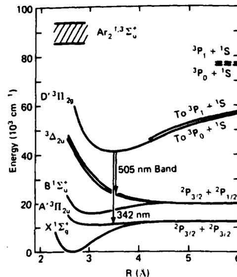
FIG. 1. Partial energy-level diagram for molecular iodine showing the well known  $D' \rightarrow A'$  UV band and the green excimer transition (after Refs. 1 and 14). The position of the argon molecular excited states is also indicated. The upper level for the green band appears to be an ion pair state lying above but close to  $D'$ .
