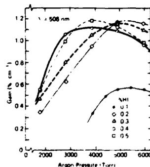
FIG. 5. Dependence of the green gain coefficient on the composition and total pressure of the Ar/HI mixture. The dye laser probe wavelength is 506 nm.
