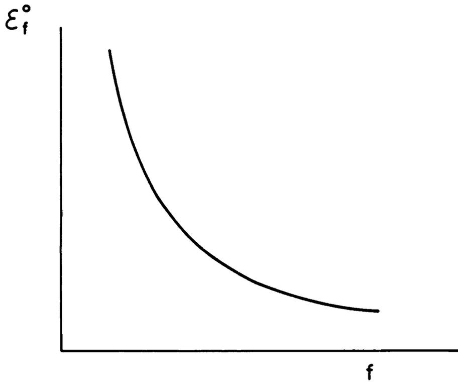
Figure 1. Ductility as a function of volume fraction of void nucleating inclusions, assuming voids nucleate at zero strain.
