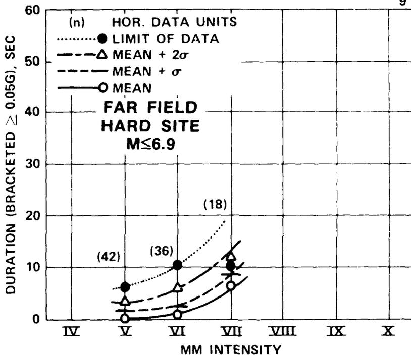
Figure 21. Krinitzsky-Chang curves for bracketed duration ( $\geq 0.05$  g) versus MM Intensity: far field, hard site,  $M \leq 6.9$
