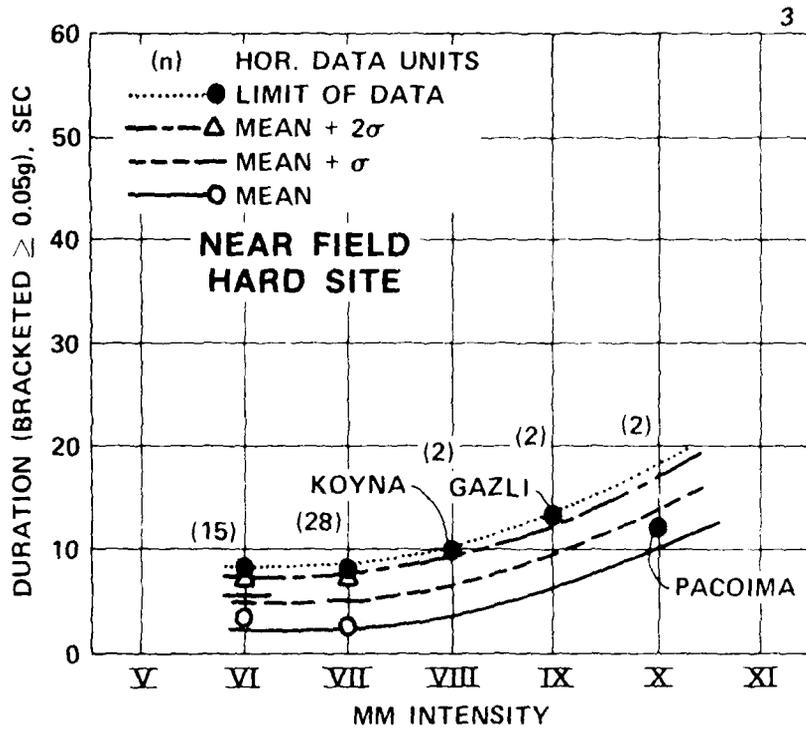
Figure 18. Krinitzsky-Chang curves for bracketed duration ( $\Delta$  0.05 g) versus MM Intensity: near field, hard site
