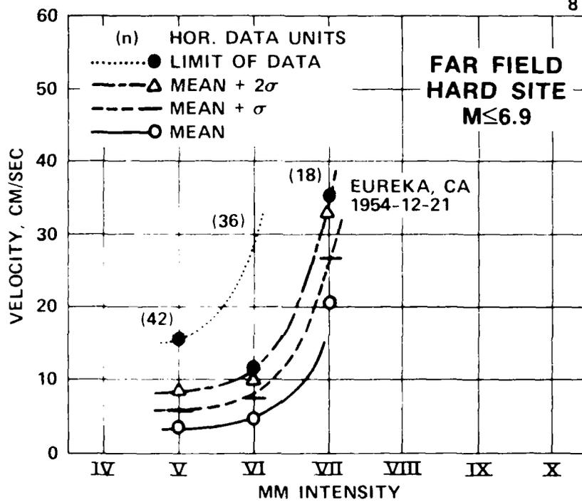
Figure 20. Krinitzsky-Chang curves for velocity versus MM Intensity: far field, hard site, M ≤ 6.9
