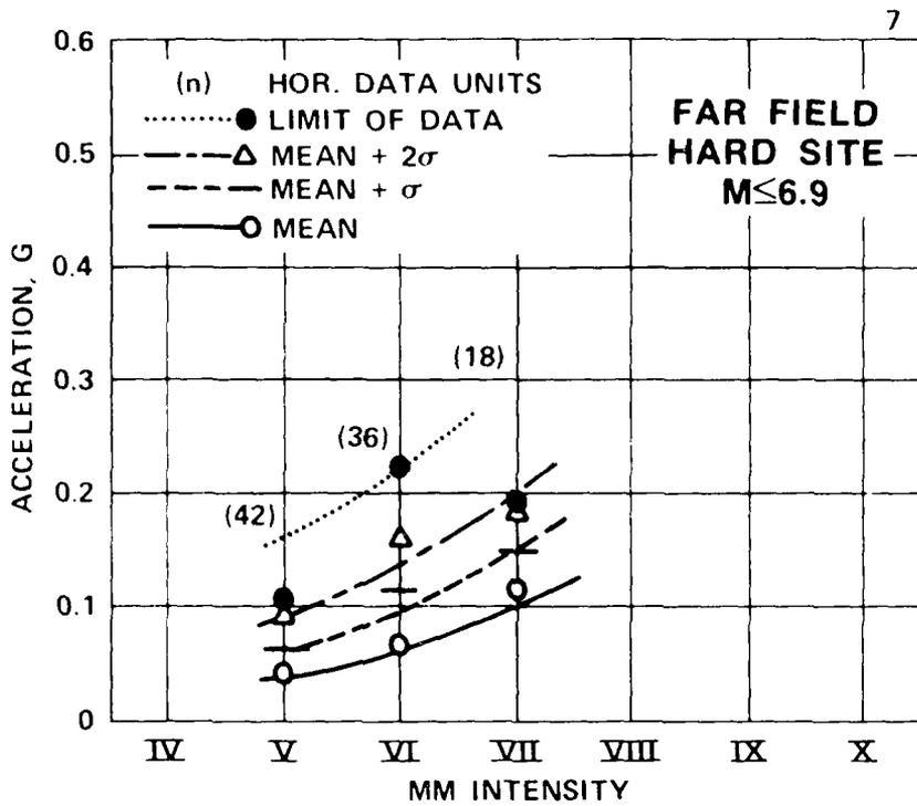
Figure 19. Krinitzsky-Chang curves for acceleration versus MM Intensity: far field, hard site,  $M \leq 6.9$
