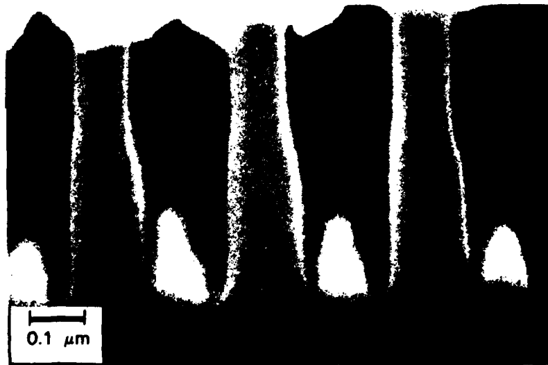
Figure 4-14. SEM of the base region of a Si PBT, where the W base metal is separated from the Si sidewall. In the corresponding I-V characteristics shown above, V_{BE} = +0.4 for the top curve.
