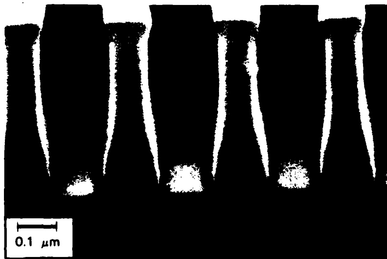
Figure 4-15. SEM of the base region of a Si PBT in which the base metal appears to be in partial contact with the Si sidewall. In the corresponding I-V characteristics shown above, V_{BE} = +0.4 for the top curve.
