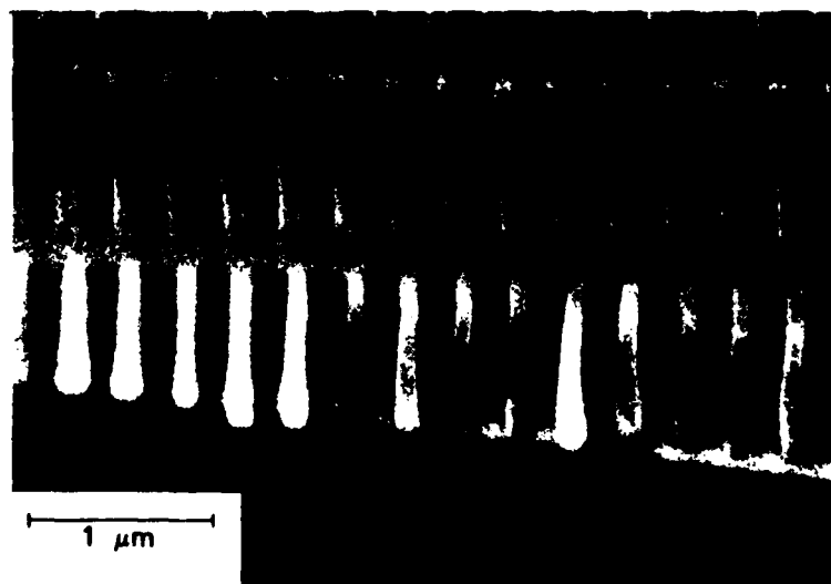
Figure 4-7. SEM of a grating pattern in a 0.6\text{-}\mu\text{m} -thick nitrocellulose film on a silicon wafer. The sample was exposed to a beam of 500\text{-eV Ar}^+ at a current density of 0.25 \text{ mA cm}^{-2} for 40 s. The \text{SiN}_x stencil mask used for this exposure consisted of a 320-nm grating with a crossmember every 3.8 \mu\text{m} to strengthen the mask. Two shadows of the crossmembers can be seen in the nitrocellulose.
