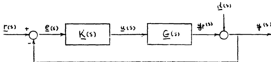
Figure 4.1. Block Diagram of a MIMO Compensated Plant
