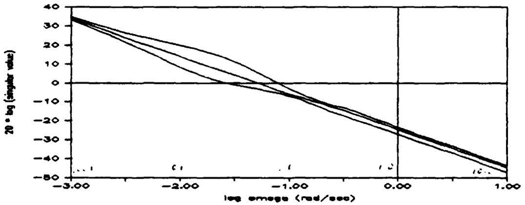
(b) Kalman filter open loop  $G(kf)$
