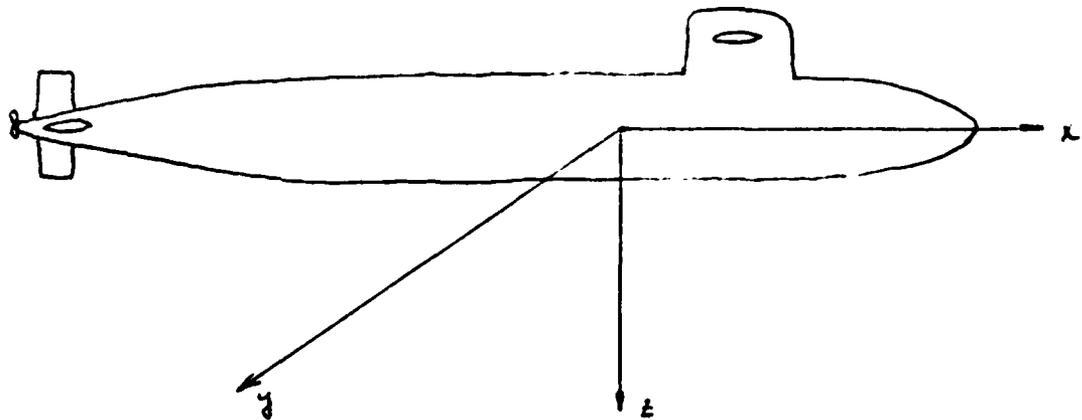
Figure 2.1 - Submarine Body Reference Frame Axes
