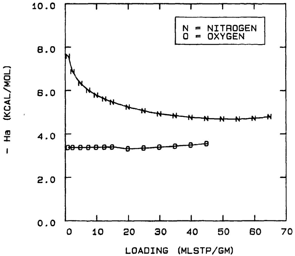
FIG 5-24. ISOSTERIC HEAT OF ADSORPTION FOR NITROGEN AND OXYGEN ON MOLECULAR SIEVE 5A.
