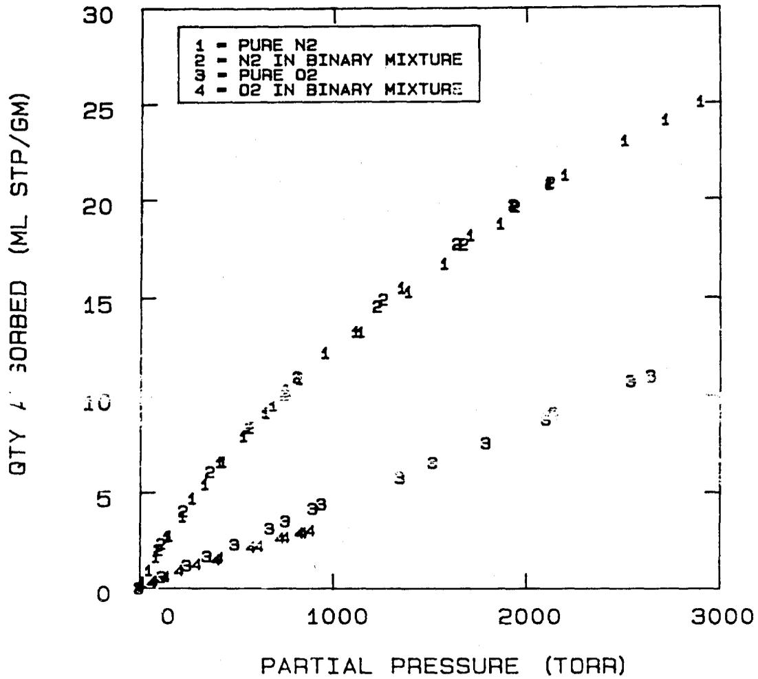
FIG 5-48. PURE AND MULTICOMPONENT DATA OF NITROGEN AND OXYGEN ON MOLECULAR SIEVE 5A AT 24°C.
