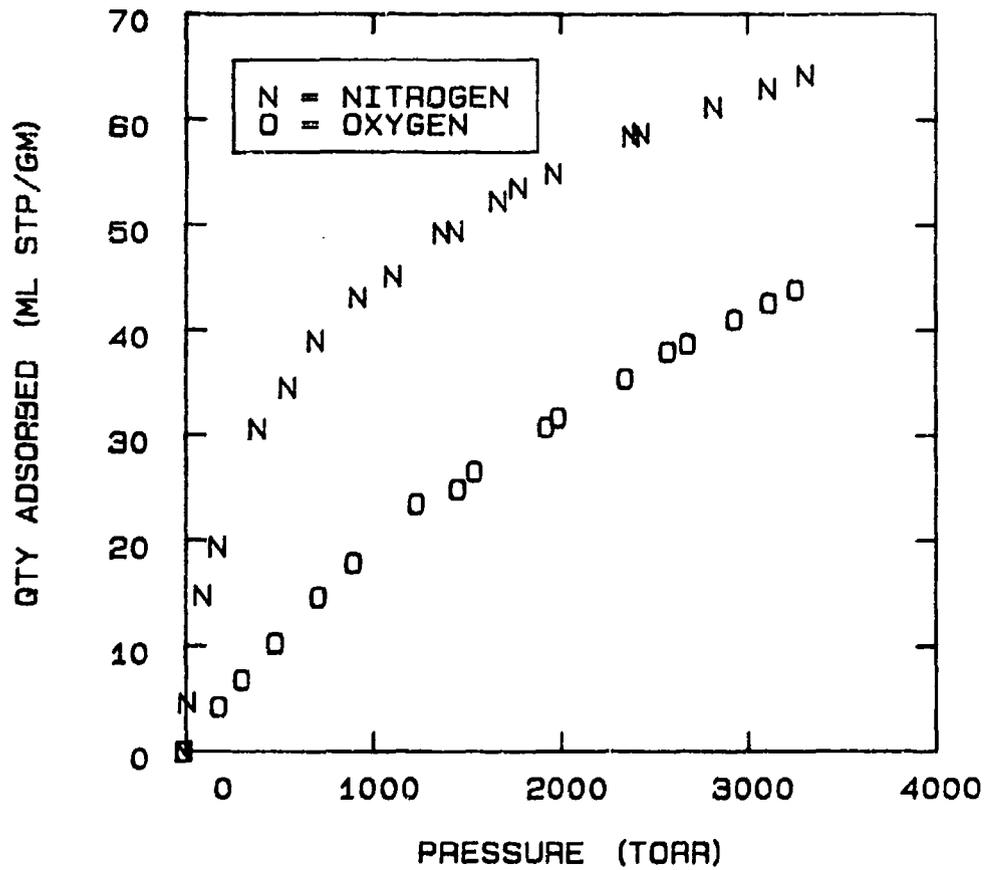
FIG 5-8. PURE NITROGEN AND OXYGEN ON MOLECULAR SIEVE 5A AT -40°C.
