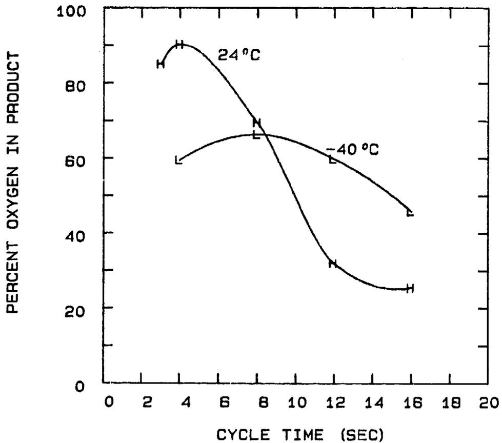
FIG 5-91. EFFECT OF CYCLE TIME AND TEMPERATURE ON THE PSA UNIT CONFIGURED FOR 2 STEPS/CYCLE, 0.029" PURGE ORIFICE, AND 100 SCCM PRODUCT FLOW.
