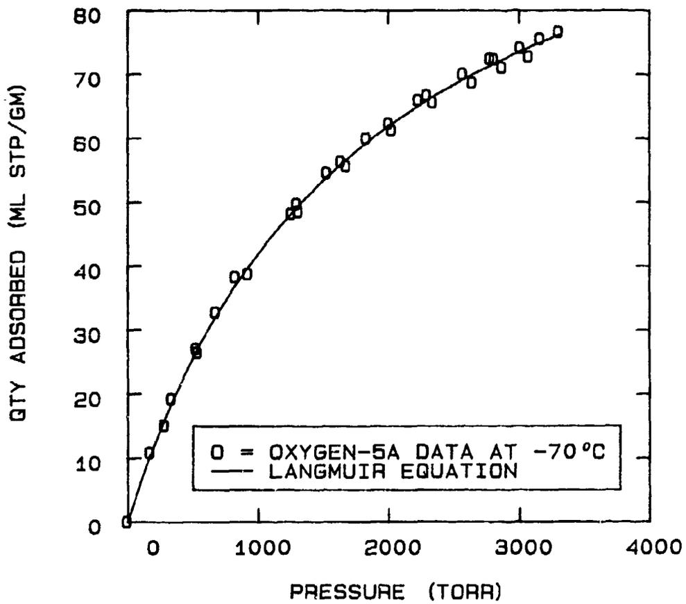
FIG 5-18. FITTING A LANGMUIR EQUATION TO THE OXYGEN-5A DATA AT -70°C.
