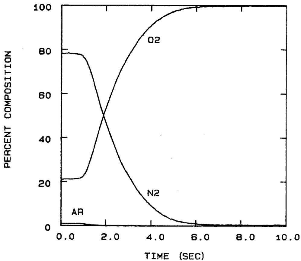
FIG 5-64. RUN 102714 : COLUMN OXYGEN BREAKTHROUGH AT 24°C, 25 SLPM, AND BED PRESSURE OF APPROXIMATELY 18.5 PSIA.
