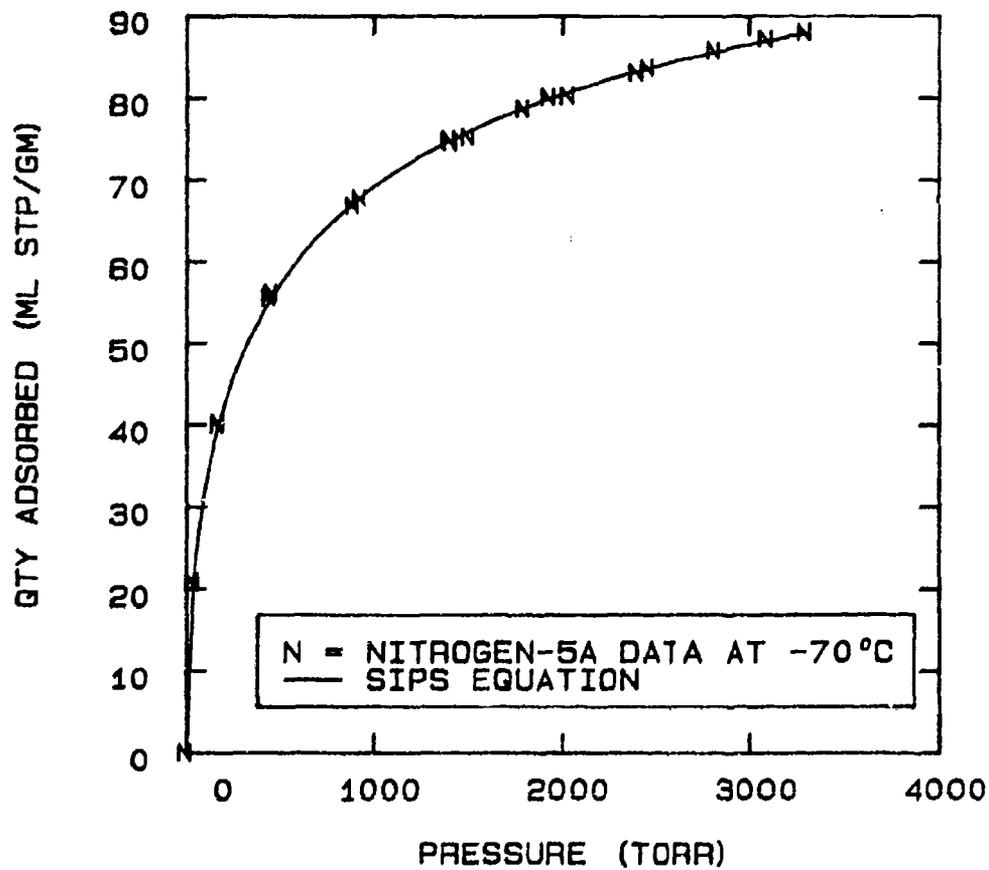
FIG 5-21. FITTING A SIPS EQUATION TO THE NITROGEN-5A DATA AT -70 °C.
