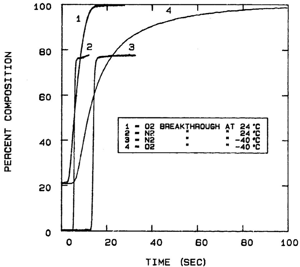
FIG 5-75. EFFECT OF TEMPERATURE ON NITROGEN AND OXYGEN BREAKTHROUGH FOR A FLOWRATE OF 13 SLPM AND BED PRESSURE OF 25 PSIA.
