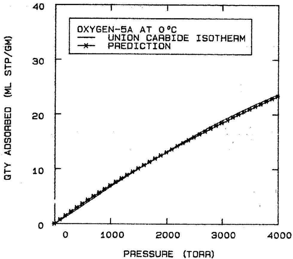
FIG 5-34. PREDICTION OF UNION CARBIDE DATA FOR OXYGEN-5A SORPTION AT 0°C USING A STATISTICAL THERMODYNAMIC MODEL WHERE:  $K=0.0006969$ ,  $B=38.8$ ,  $m=20$ .
