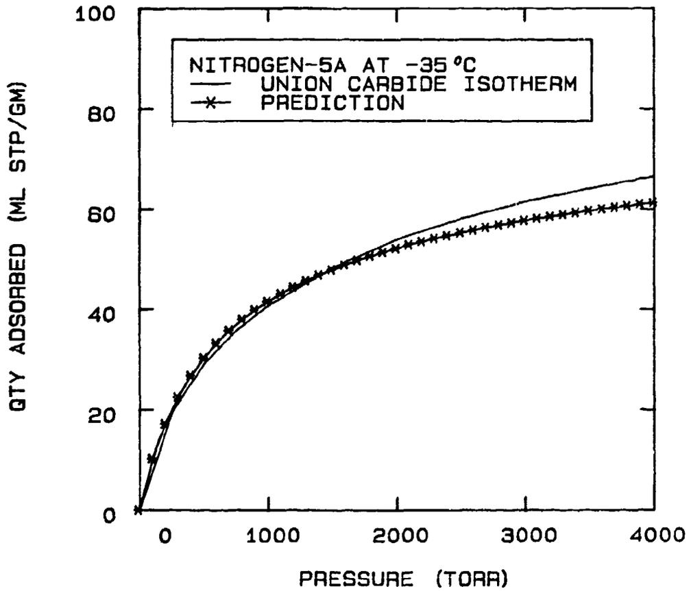
FIG 5-38. PREDICTION OF UNION CARBIDE DATA FOR NITROGEN-5A SORPTION AT -35 °C USING A STATISTICAL THERMODYNAMIC MODEL WHERE:  $K=0.01261$ ,  $B=77.6$ ,  $m=10$ .
