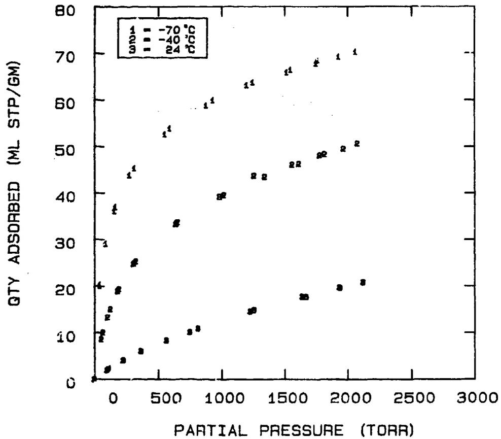
FIG 5-45. NITROGEN LOADING AT 24, -40, AND -70°C FOR THE AIR-5A SYSTEM.
