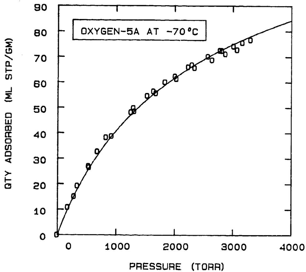
FIG 5-29. CORRELATION OF OXYGEN SORPTION ON MOLECULAR SIEVE 5A AT -70°C USING A STATISTICAL THERMODYNAMIC MODEL WHERE:  $K = 0.005952$ ,  $B = 38.8$ ,  $m = 20$ .
