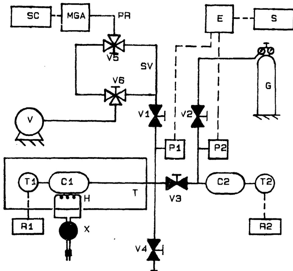
FIG 4-8. MULTICOMPONENT EQUILIBRIUM APPARATUS. C1. SAMPLE CHAMBER, C2. CHARGE CHAMBER, E. PRESSURE TRANSDUCER ELECTRONICS BOX, G. BOTTLED GAS, H. HEATER, P1 AND P2. PRESSURE TRANSDUCERS, R1 AND R2. DIGITAL READOUTS, S. STRIP CHART RECORDER, T. ENVIRONMENTAL TEST CHAMBER, T1 AND T2 THERMOCOUPLES, V. VACUUM PUMP, V1-4. MANUAL VALVES, X. VARIAC, MGA. MEDICAL GAS ANALYZER, SC. MGA STRIP CHART RECORDER, PR. MGA GAS SAMPLING PROBE, SV. MGA SAMPLING VOLUME, AND V5-6. THREE-WAY VALVES.
