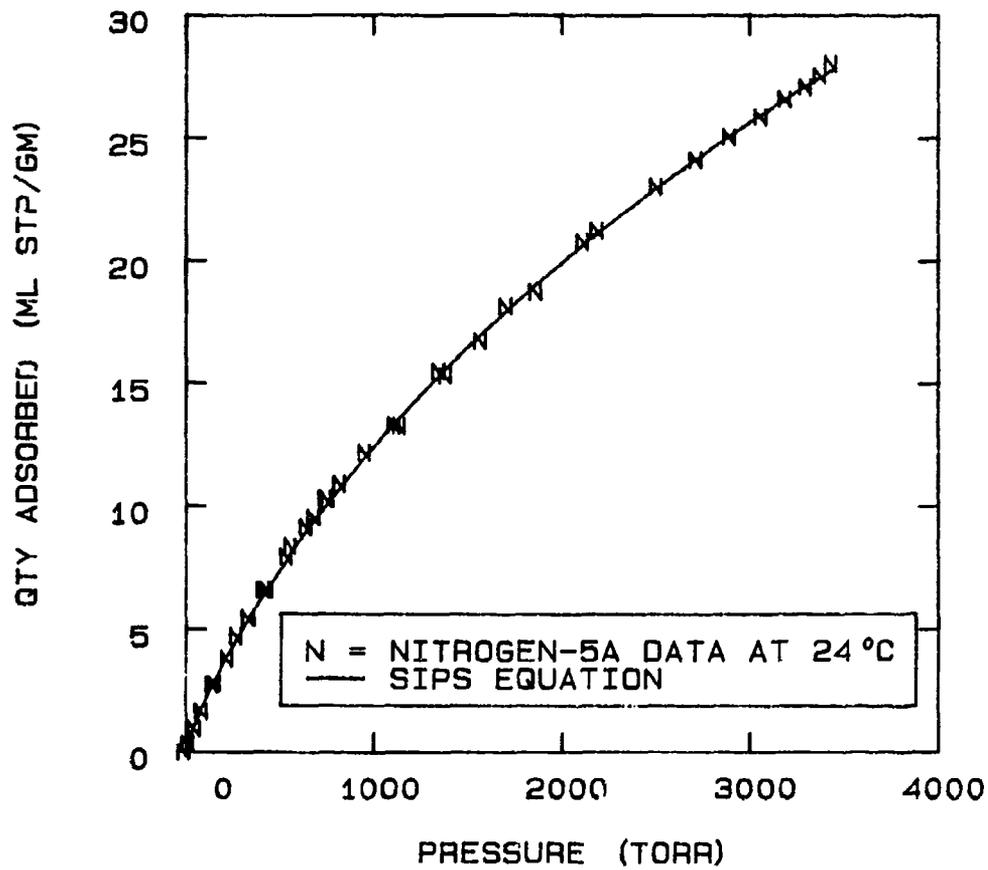
FIG 5-19. FITTING A SIPS EQUATION TO THE NITROGEN-5A DATA AT 24°C.
