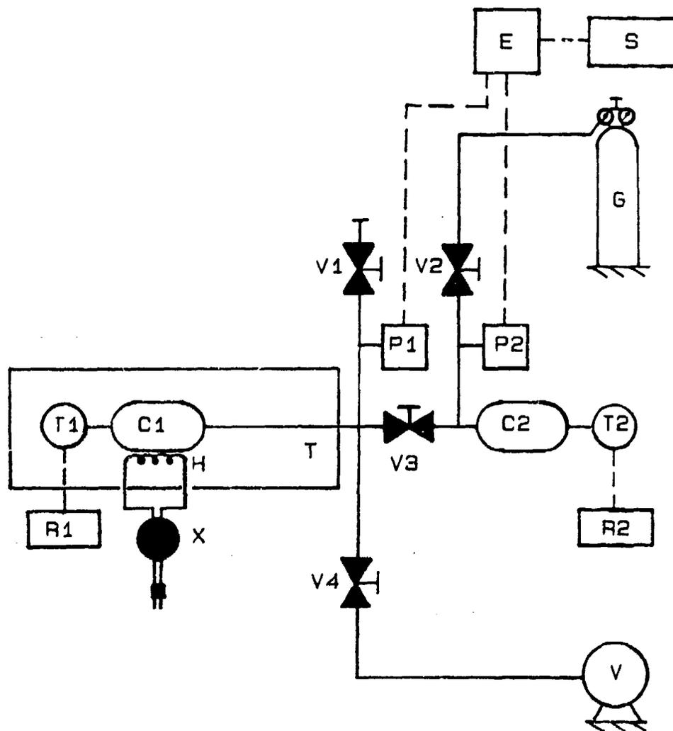
FIG 4-6. PURE COMPONENT EQUILIBRIUM APPARATUS. C1. SAMPLE CHAMBER, C2. CHARGE CHAMBER, E. PRESSURE TRANSDUCER ELECTRONICS BOX, G. BOTTLED GAS, H. HEATER, P1 AND P2. PRESSURE TRANSDUCERS, R1 AND R2. DIGITAL READOUTS, S. STRIP CHART RECORDER, T. ENVIRONMENTAL TEST CHAMBER, T1 AND T2. THERMOCOUPLES, V. VACUUM PUMP, V1-4. MANUAL VALVES, AND X. VARIAC.
