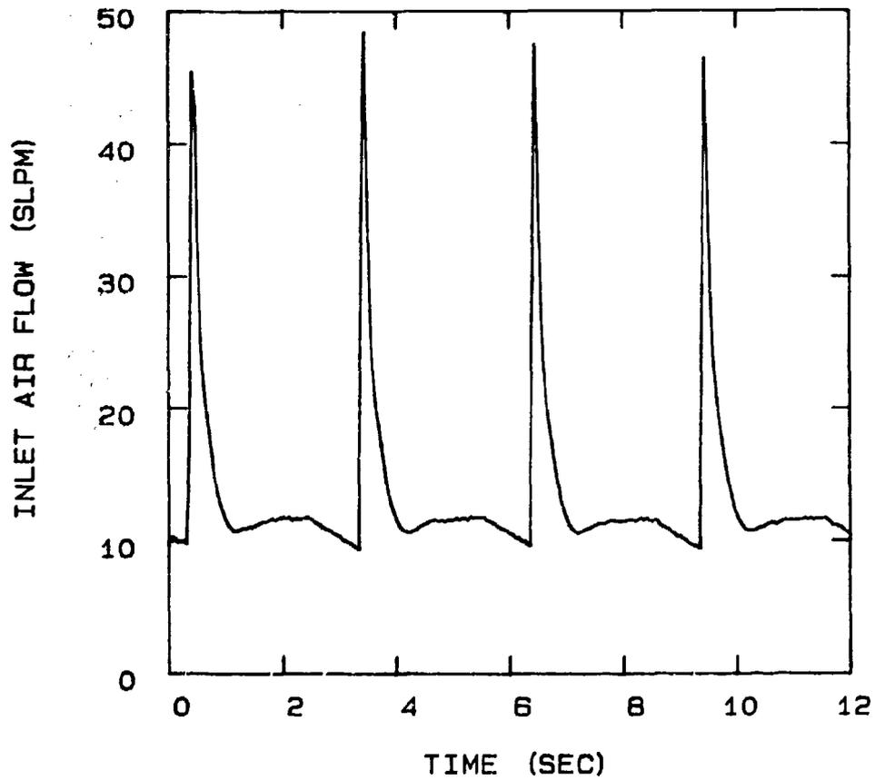
FIG 5-76. AIR FLOW INTO THE PSA UNIT OPERATING AT 24°C AND CONFIGURED FOR A 2 STEP CYCLE, 6 SEC. CYCLE TIME, 0.020" PURGE ORIFICE, AND 100 SCCM PRODUCT FLOW.
