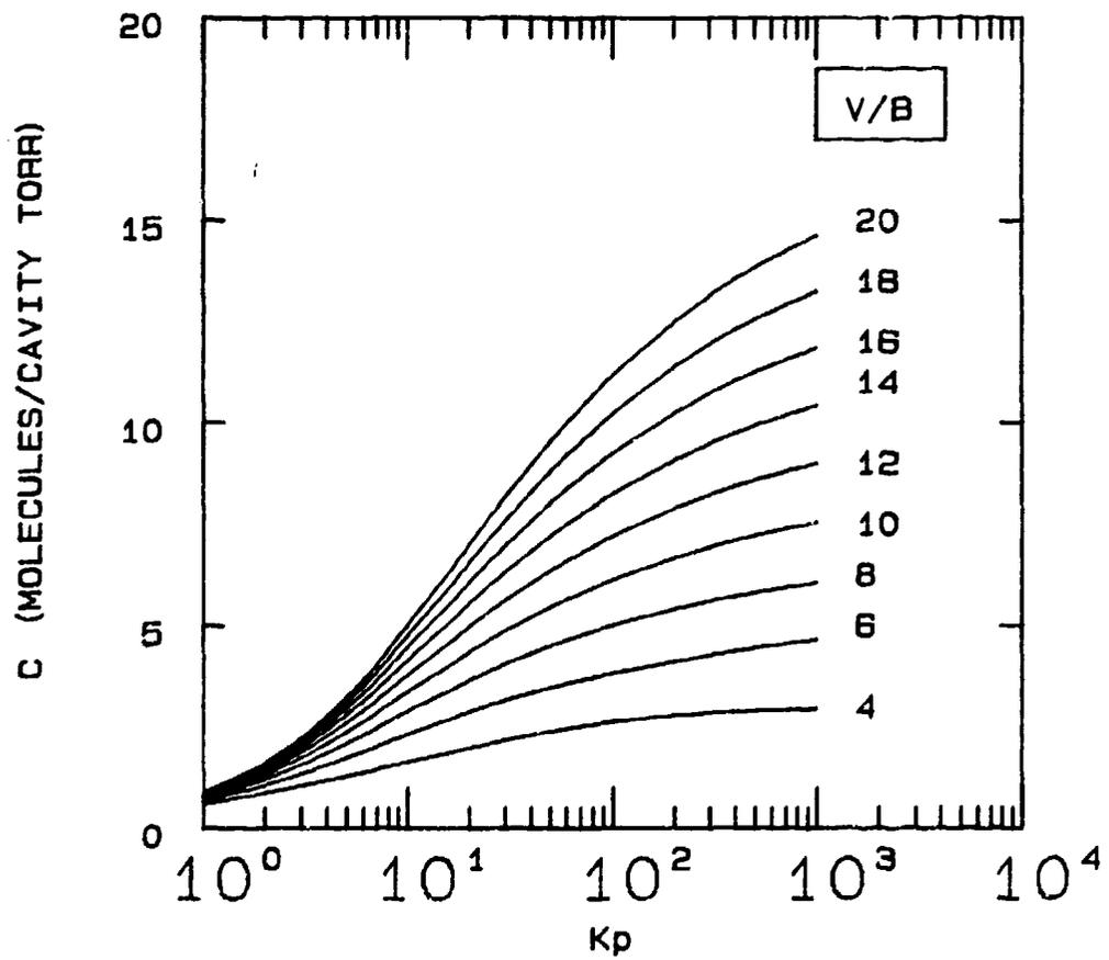
FIG 5-26. THEORETICAL EQUILIBRIUM CURVES CALCULATED USING THE STATISTICAL THERMODYNAMIC MODEL.
