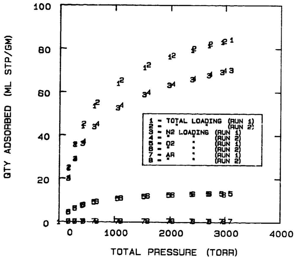
FIG 5-41. AIR-5A AT  $-70^{\circ}\text{C}$  WHERE THE TOTAL MOLAR RATIO OF NITROGEN, OXYGEN, AND ARGON WITHIN THE SYSTEM IS CONSTANT AT 78.14 : 20.92 : 0.94, RESPECTIVELY.
