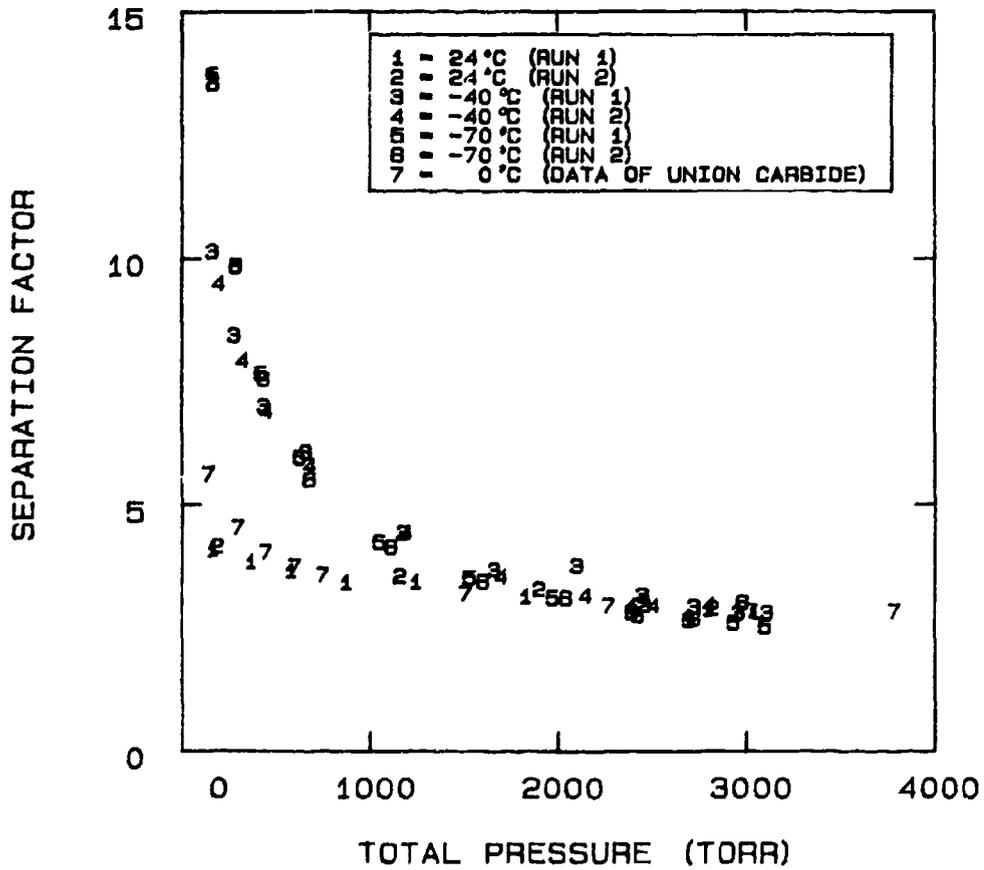
FIG 5-51. SEPARATION FACTORS FOR THE BINARY MIXTURE OF NITROGEN AND OXYGEN ON MOLECULAR SIEVE 5A.
