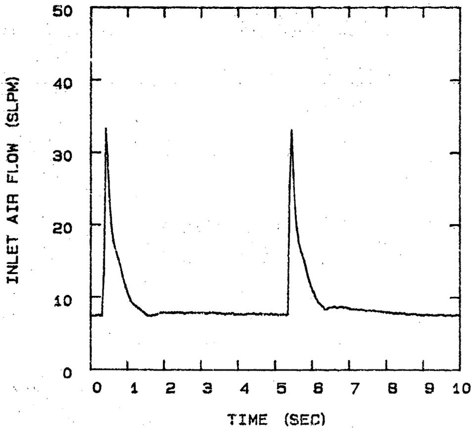
FIG 5-98. INLET FLOW FOR PSA UNIT CONFIGURATION: 24°C, 6 STEP CYCLE (1SEC, 3SEC, 1SEC), 10 SEC CYCLE TIME, 0.020" PURGE ORIFICE AND 100 SCCM PRODUCT FLOW.
