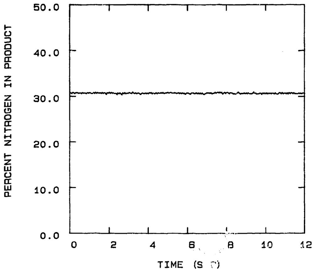
FIG 5-83. PRODUCT N2 FROM THE PSA UNIT OPERATING AT -40 °C AND CONFIGURED FOR A 2 STEP CYCLE, 6 SEC. CYCLE TIME, 0.020" PURGE ORIFICE, AND 100 SCCM PRODUCT FLOW.
