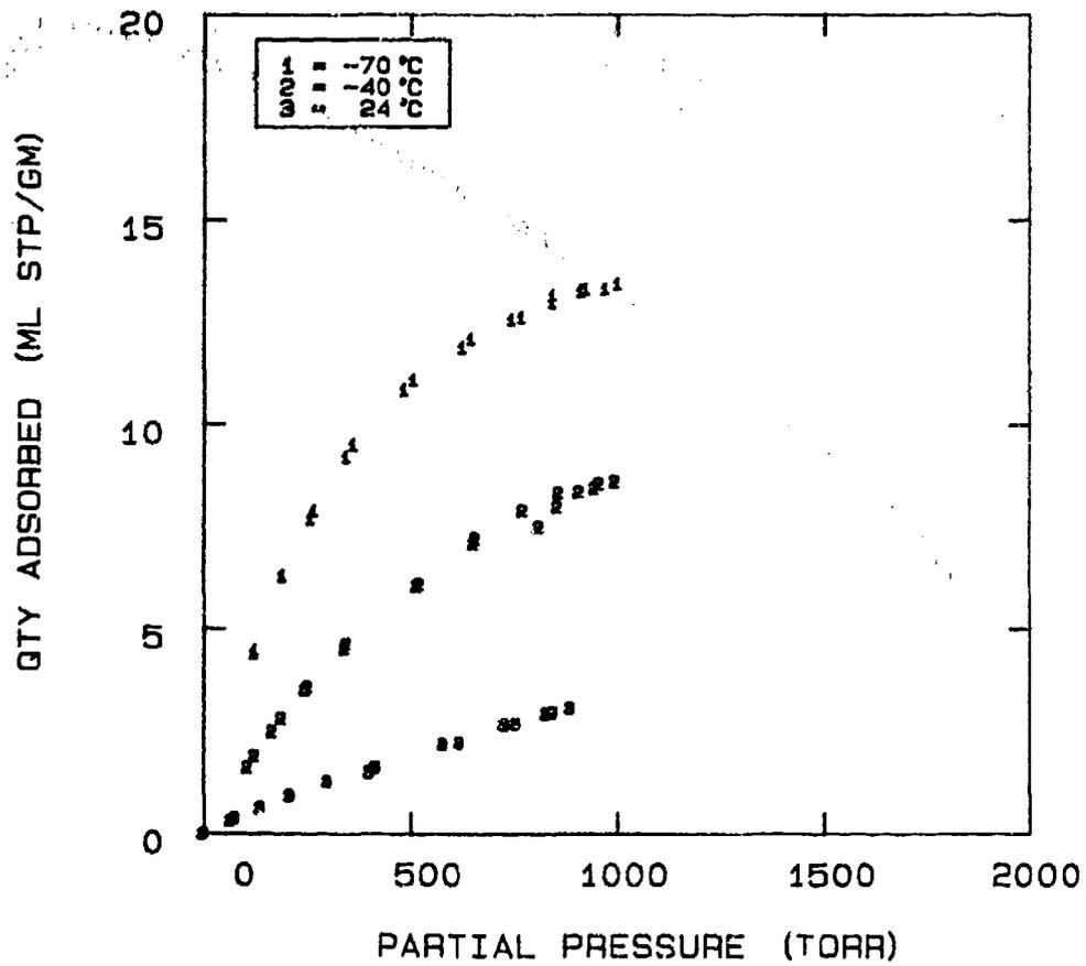
FIG 5-46. OXYGEN LOADING AT 24, -40, AND -70°C FOR THE AIR-5A SYSTEM.
