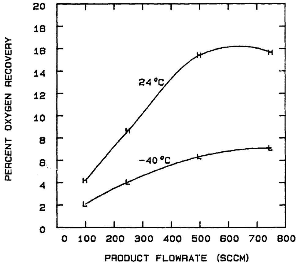
FIG 5-109. EFFECT OF PRODUCT FLOWRATE AND TEMPERATURE ON OXYGEN RECOVERY FOR A 2 STEP SYSTEM WITH A CYCLE TIME OF 8 SEC AND A 0.020" PURGE ORIFICE.
