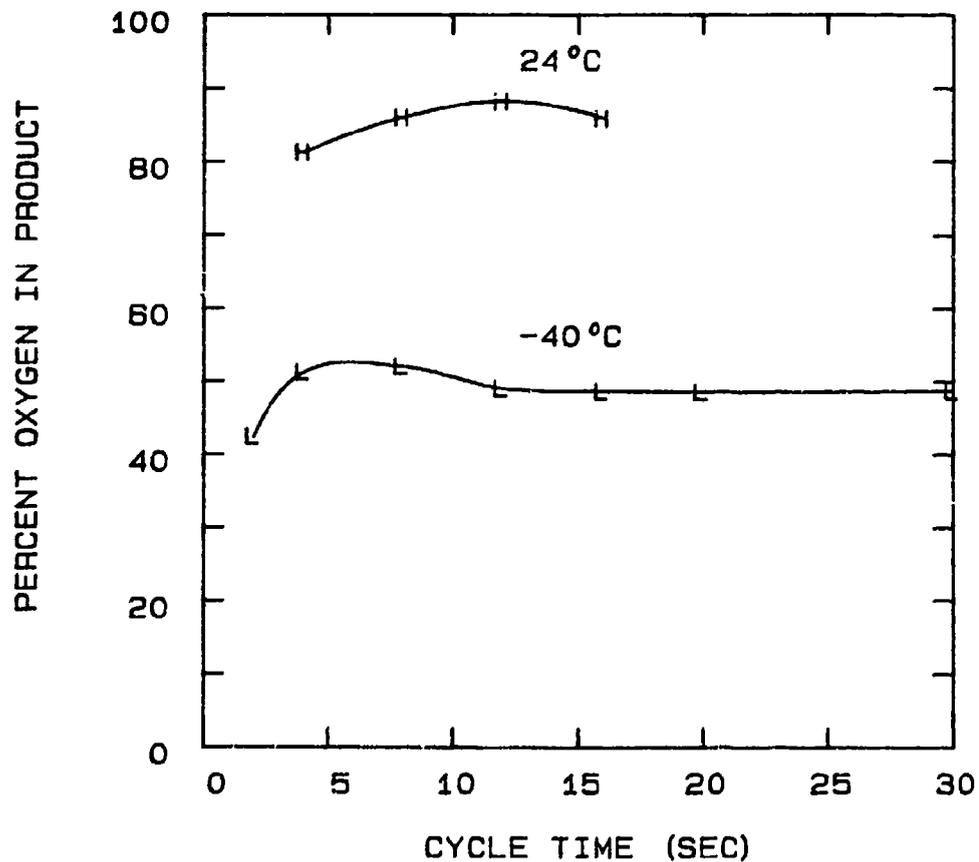
FIG 5-89. EFFECT OF CYCLE TIME AND TEMPERATURE ON THE PSA UNIT CONFIGURED FOR 2 STEPS/CYCLE, 0.010" PURGE ORIFICE, AND 100 SCCM PRODUCT FLOW.
