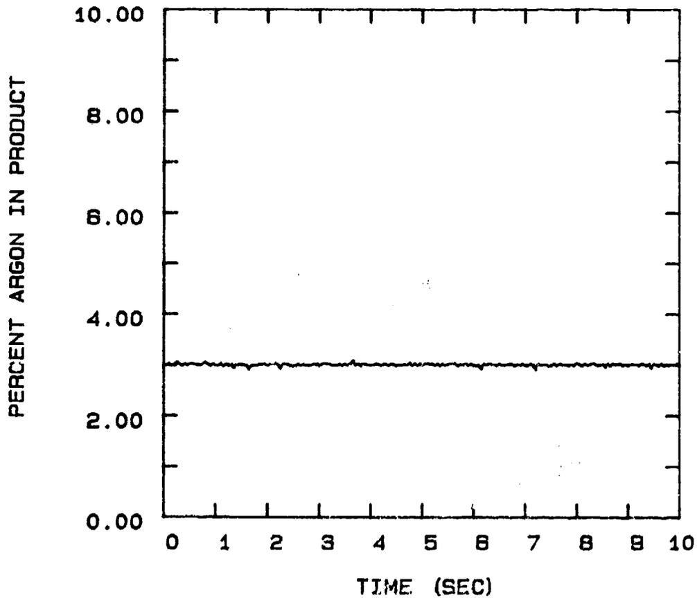
FIG 5-107. PRODUCT AR% FOR PSA UNIT CONFIGURATION:
