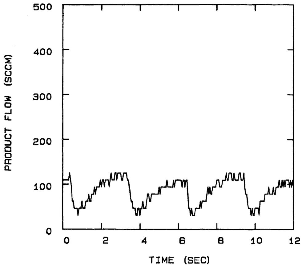
FIG 5-81. PRODUCT FLOW FROM THE PSA UNIT OPERATING AT  $-40^{\circ}\text{C}$  AND CONFIGURED FOR A 2 STEP CYCLE, 6 SEC CYCLE TIME, 0.020" PURGE ORIFICE, AND 100 SCCM PRODUCT FLOW.
