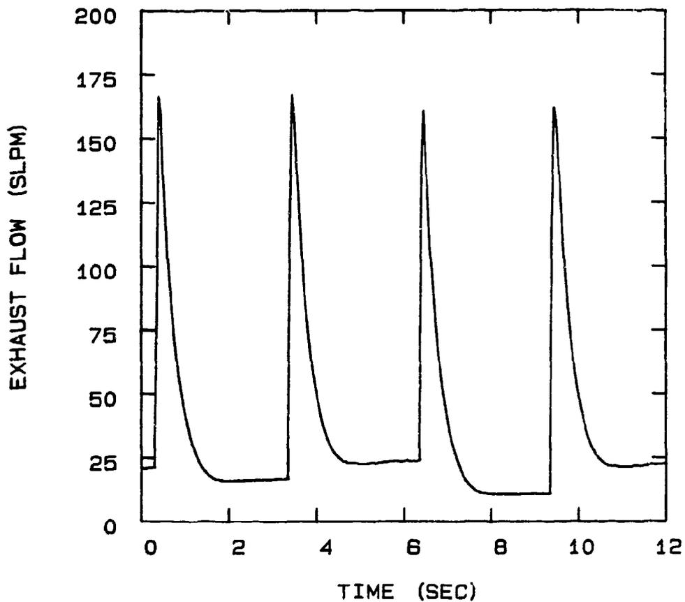
FIG 5-79. EXHAUST FLOW FROM THE PSA UNIT OPERATING AT -40°C AND CONFIGURED FOR A 2 STEP CYCLE, 6 SEC. CYCLE TIME, 0.020" PURGE ORIFICE, AND 100 SCCM PRODUCT FLOW.
