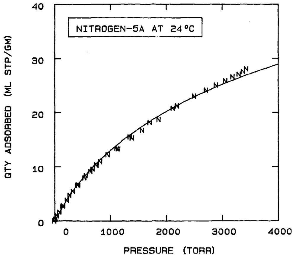
FIG 5-30. CORRELATION OF NITROGEN SORPTION ON MOLECULAR SIEVE 5A AT 24°C USING A STATISTICAL THERMODYNAMIC MODEL WHERE:  $K=0.001902$ ,  $B=97$ , AND  $m=8$ .
