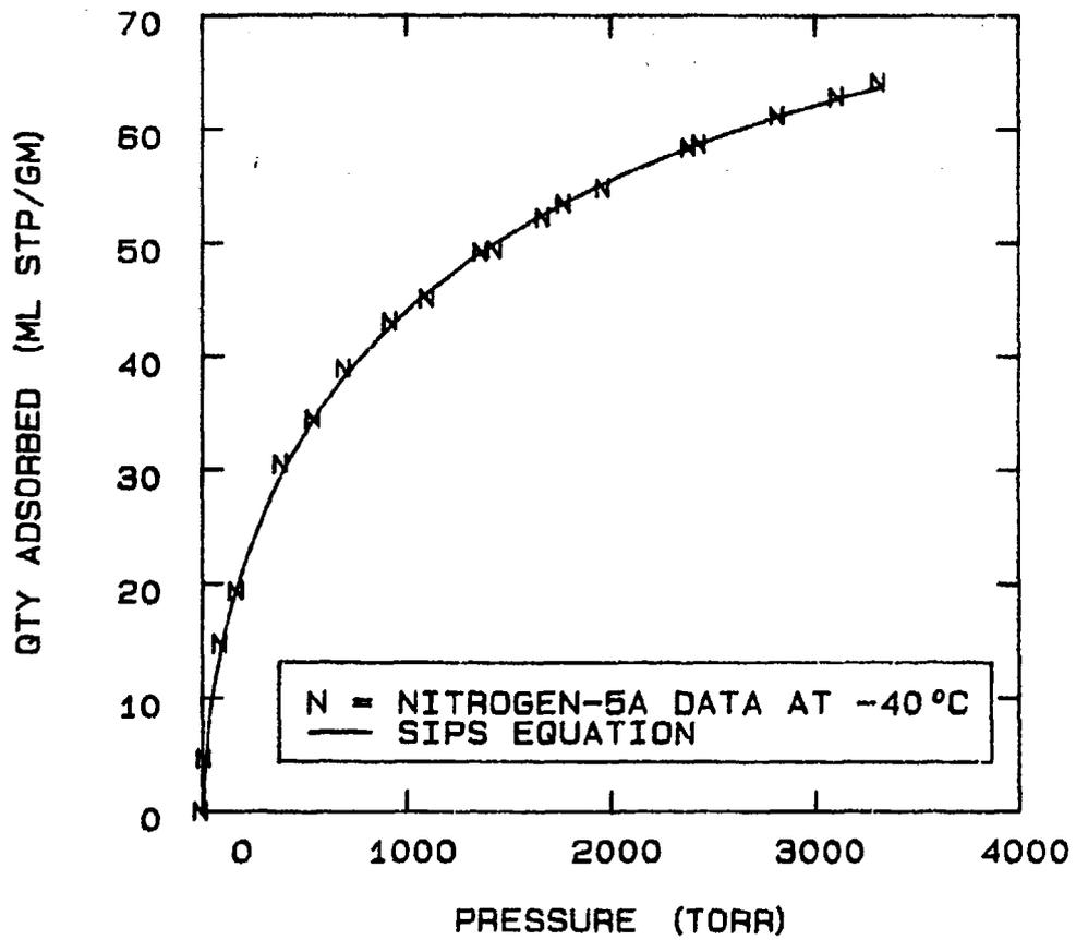
FIG 5-20. FITTING A SIPS EQUATION TO THE NITROGEN-5A DATA AT -40°C.
