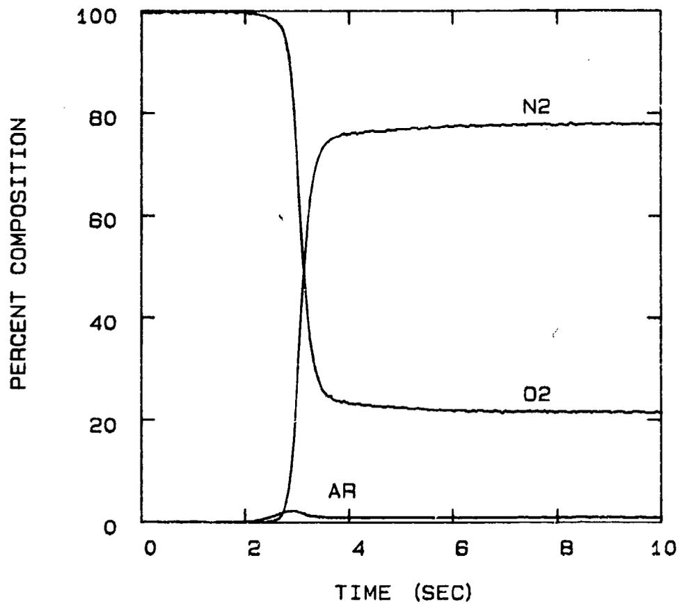
FIG 5-61. RUN 102021 : COLUMN NITROGEN BREAKTHROUGH AT 24°C, 25 SLPM, AND BED PRESSURE OF 25 PSIA.
