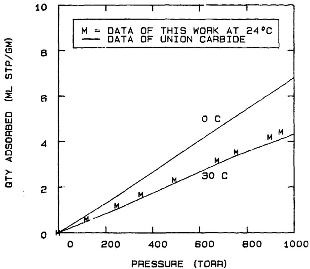
FIG 5-12. OXYGEN ISOTHERM ON MOLECULAR SIEVE 5A AT 24°C SHOWN WITH THE DATA OF UNION CARBIDE AT LOW PRESSURE.
