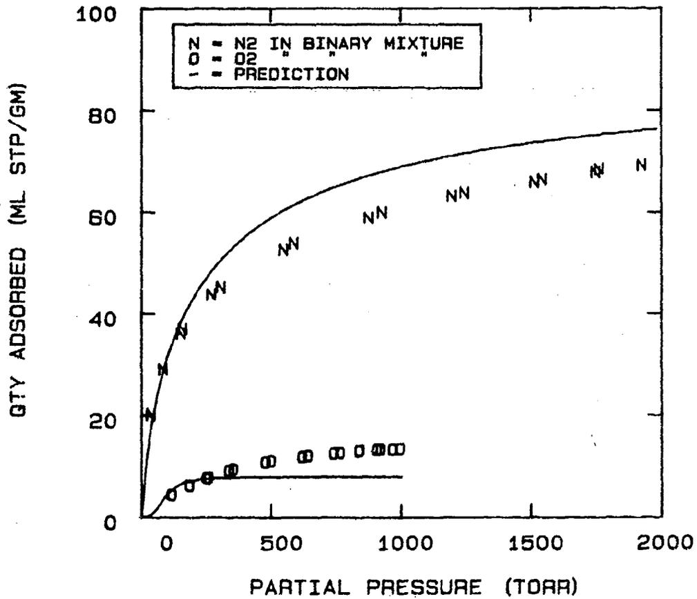
FIG 5-54. PREDICTION OF NITROGEN-OXYGEN ADSORPTION ON MOLECULAR SIEVE 5A AT -70°C USING A STATISTICAL THERMODYNAMIC MODEL WITH PURE COMPONENT PARAMETERS.
