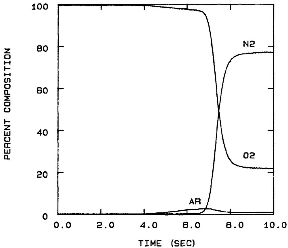
FIG 5-66. RUN 110413 : COLUMN NITROGEN BREAKTHROUGH AT -40 °C, 25 SLPM, AND BED PRESSURE OF APPROXIMATELY 18.5 PSIA.
