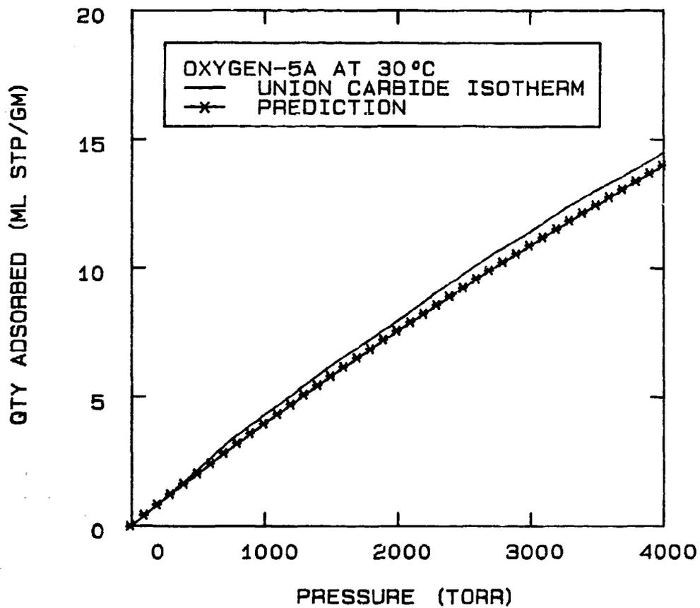
FIG 5-36. PREDICTION OF UNION CARBIDE DATA FOR OXYGEN-5A SORPTION AT 30°C USING A STATISTICAL THERMODYNAMIC MODEL WHERE:  $K=0.0003771$ ,  $B=38.8$ ,  $m=20$ .
