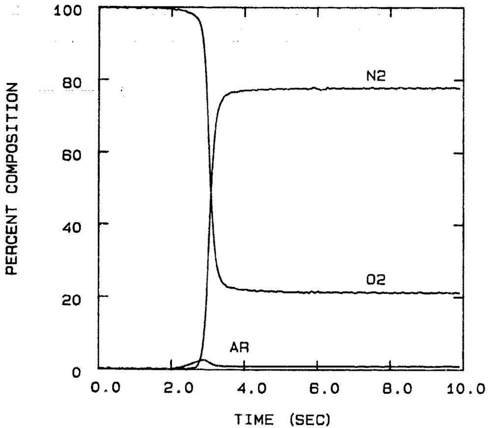
FIG 5-62. RUN 102712 : COLUMN NITROGEN BREAKTHROUGH AT 24°C, 25 SLPM, AND BED PRESSURE OF APPROXIMATELY 18.5 PSIA.
