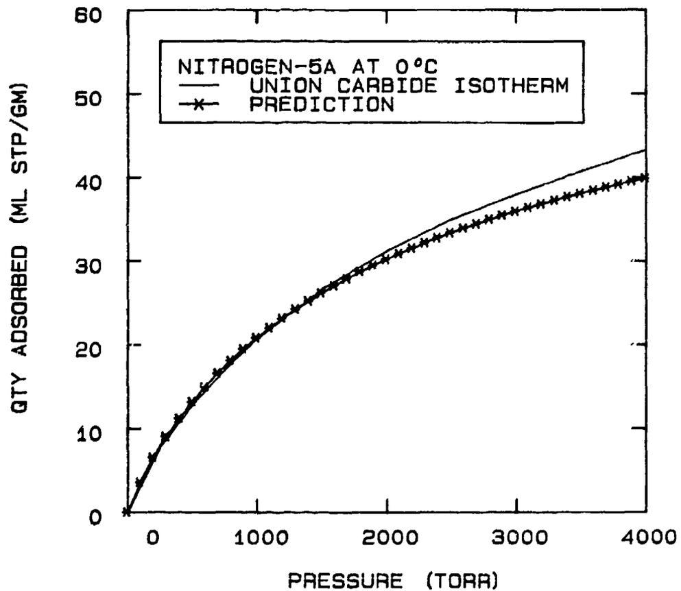
FIG 5-37. PREDICTION OF UNION CARBIDE DATA FOR NITROGEN-5A SORPTION AT 0°C USING A STATISTICAL THERMODYNAMIC MODEL WHERE:  $K=0.003711$ ,  $B=89.3$ ,  $m=8$ .
