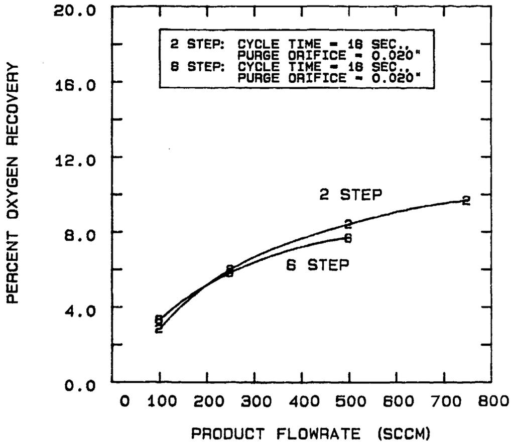
FIG 5-111. COMPARISON OF OXYGEN RECOVERY BETWEEN A 2 STEP AND 6 STEP SYSTEM OPERATING AT -40 °C.
