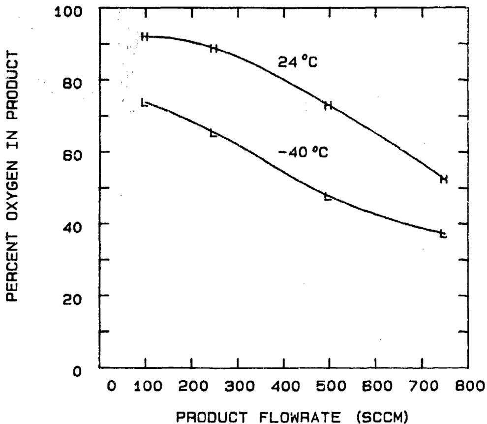
FIG 5-92. EFFECT OF PRODUCT FLOWRATE AND TEMPERATURE ON THE PSA UNIT CONFIGURED FOR 2 STEPS/CYCLE, 6 SEC. CYCLE TIME, AND 0.020" PURGE ORIFICE.
