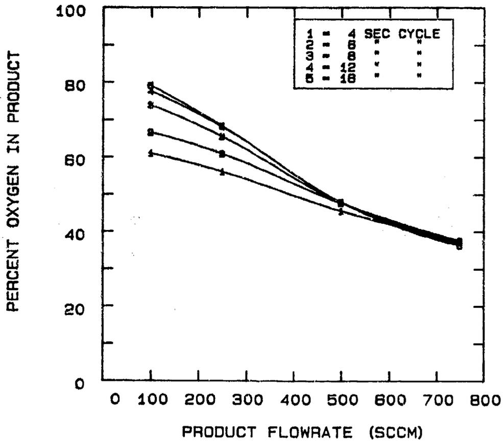
FIG 5-95. EFFECT OF PRODUCT FLOWRATE AND CYCLE TIME ON THE PSA UNIT OPERATING AT -40 °C AND CONFIGURED FOR 2 STEPS/CYCLE AND 0.020" PURGE ORIFICE.
