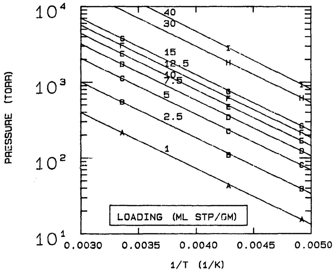
FIG 5-22. ISOSTERES FOR OXYGEN ON MOLECULAR SIEVE 5A.
