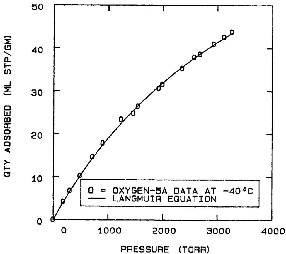
FIG 5-17. FITTING A LANGMUIR EQUATION TO THE OXYGEN-5A DATA AT -40 °C.
