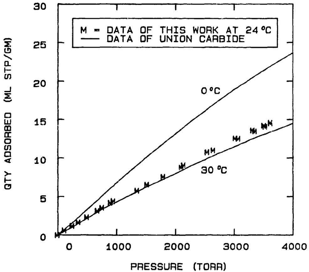
FIG 5-13. OXYGEN ISOTHERM ON MOLECULAR SIEVE 5A AT 24 °C SHOWN WITH THE DATA OF UNION CARBIDE.
