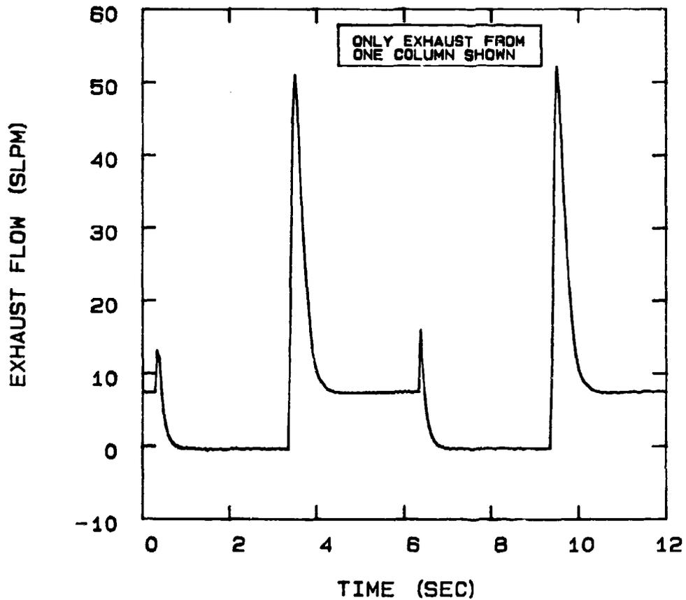
FIG 5-78. EXHAUST FLOW FROM THE PSA UNIT OPERATING AT 24°C AND CONFIGURED FOR A 2 STEP CYCLE, 6 SEC. CYCLE TIME, 0.020" PURGE ORIFICE, AND 100 SCCM PRODUCT FLOW.
