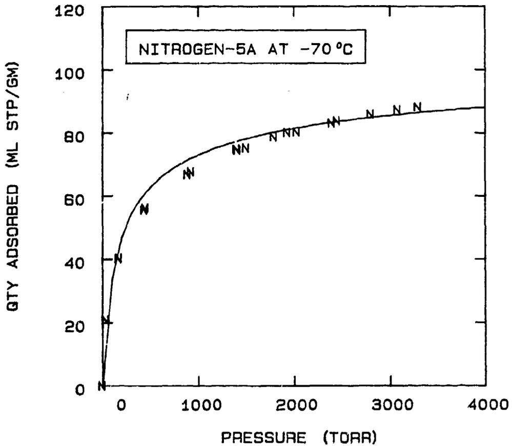
FIG 5-32. CORRELATION OF NITROGEN SORPTION ON MOLECULAR SIEVE 5A AT -70 °C USING A STATISTICAL THERMODYNAMIC MODEL WHERE:  $K=0.06585$ ,  $B=67$ , AND  $m=11$ .
