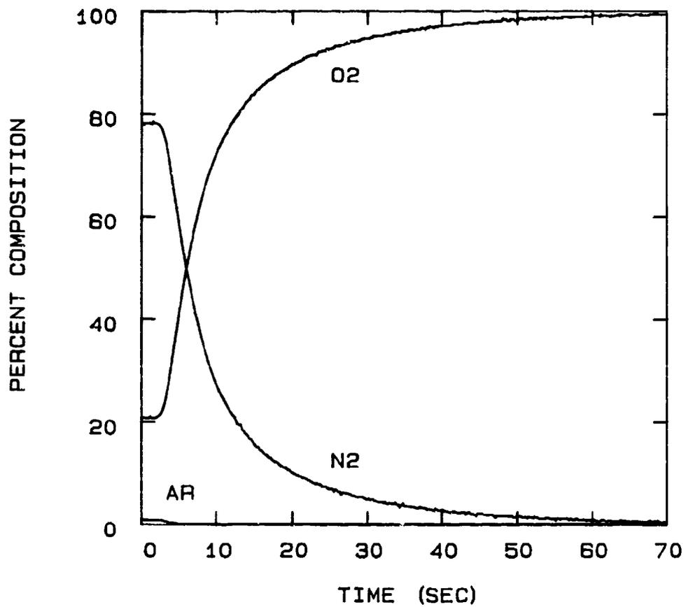
FIG 5-67. RUN 110408 : COLUMN OXYGEN BREAKTHROUGH AT -40°C, 25 SLPM, AND BED PRESSURE OF 25 PSIA.
