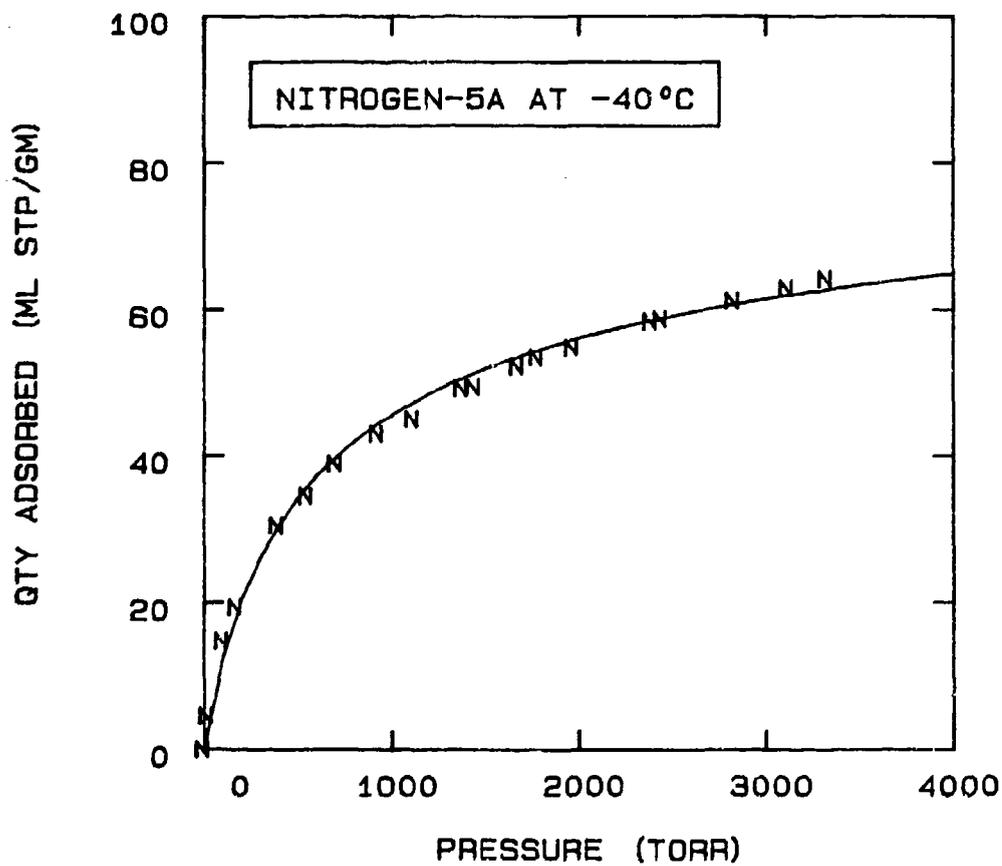
FIG 5-31. CORRELATION OF NITROGEN SORPTION ON MOLECULAR SIEVE 5A AT -40°C USING A STATISTICAL THERMODYNAMIC MODEL WHERE:  $K=0.01557$ ,  $B=76$ , AND  $m=10$ .
