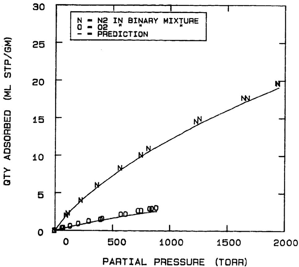
FIG 5-58. PREDICTION OF N<sub>2</sub>-O<sub>2</sub> SORPTION ON MOLECULAR SIEVE 5A AT 24°C USING THE IDEAL ADSORBED SOLUTION THEORY.
