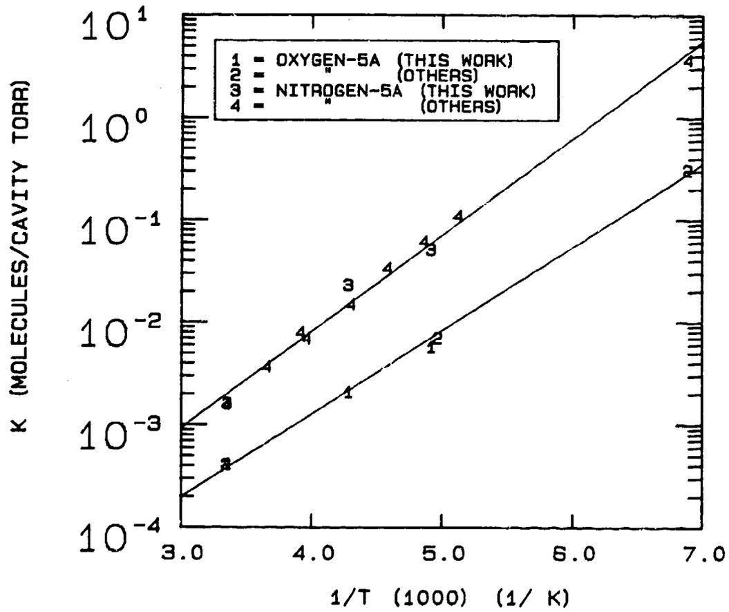
FIG 5-25. VANT HOFF PLOT SHOWING TEMPERATURE DEPENDENCE OF K.
