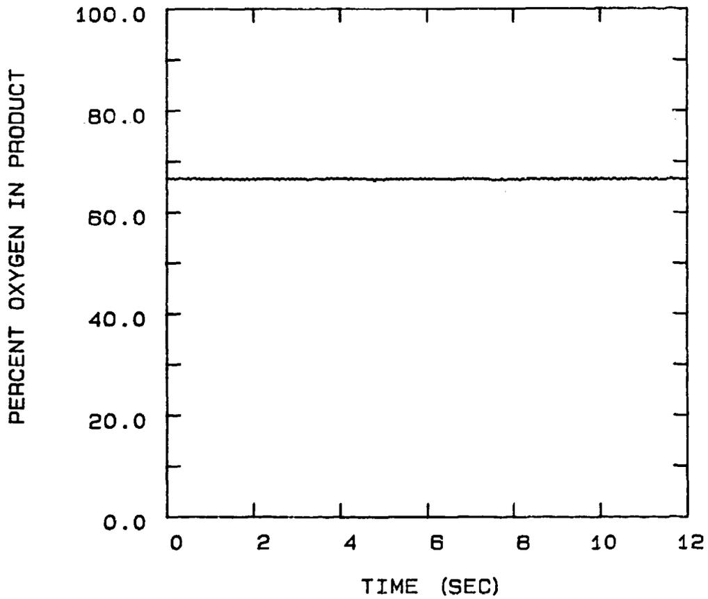
FIG 5-85. PRODUCT O<sub>2</sub> FROM THE PSA UNIT OPERATING AT -40 °C AND CONFIGURED FOR A 2 STEP CYCLE, 6 SEC. CYCLE TIME, 0.020" PURGE ORIFICE, AND 100 SCCM PRODUCT FLOW.
