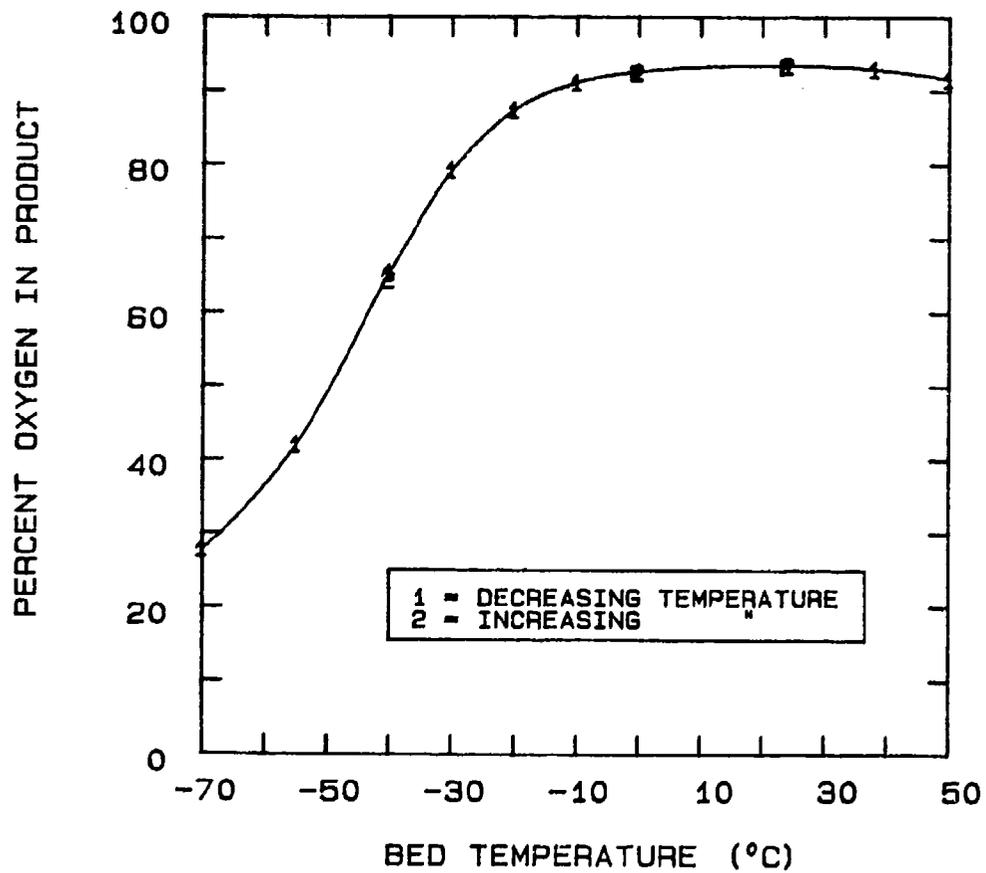
FIG 5-88. EFFECT OF BED TEMPERATURE ON A PSA UNIT CONFIGURED FOR A 2 STEP CYCLE, 6 SEC. CYCLE TIME, 0.020" PURGE ORIFICE, AND 100 SCCM PRODUCT FLOWRATE.
