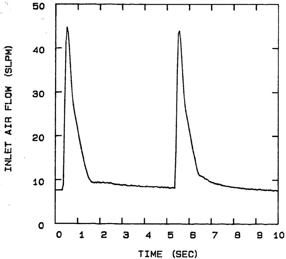
FIG 5-97. INLET FLOW FOR PSA UNIT CONFIGURATION:
