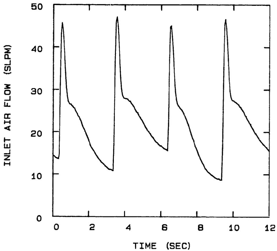
FIG 5-77. AIR FLOW INTO THE PSA UNIT OPERATING AT  $-40^{\circ}\text{C}$  AND CONFIGURED FOR A 2 STEP CYCLE, 6 SEC. CYCLE TIME, 0.020" PURGE ORIFICE, AND 100 SCCM PRODUCT FLOW.
