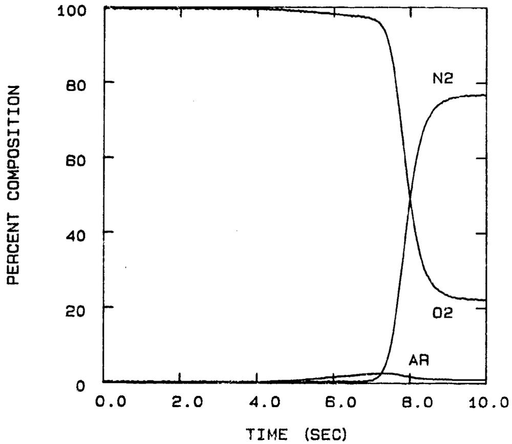
FIG 5-65. RUN 110407 : COLUMN NITROGEN BREAKTHROUGH AT -40°C, 25 SLPM, AND BED PRESSURE OF 25 PSIA.
