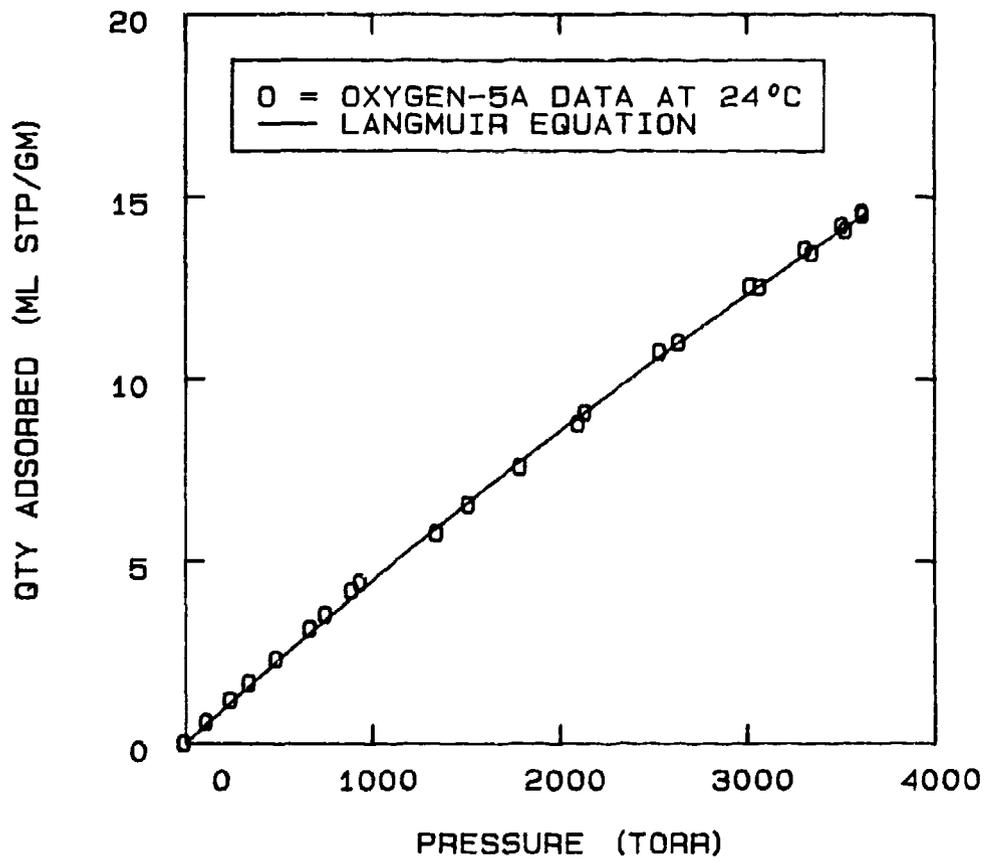
FIG 5-16. FITTING A LANGMUIR EQUATION TO THE OXYGEN-5A DATA AT 24°C.
