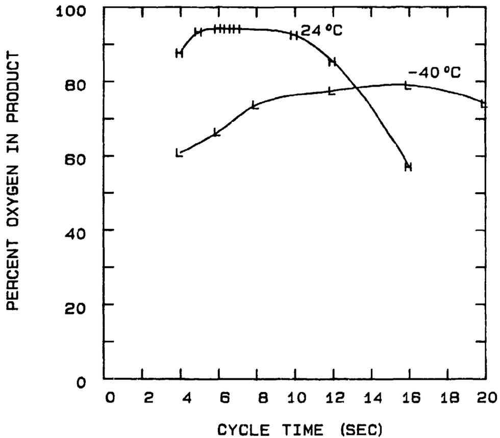
FIG 5-90. EFFECT OF CYCLE TIME AND TEMPERATURE ON THE PSA UNIT CONFIGURED FOR 2 STEPS/CYCLE, 0.020" PURGE ORIFICE, AND 100 SCCM PRODUCT FLOW.
