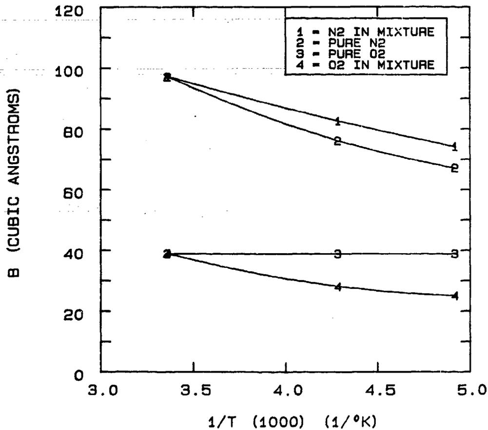
FIG 5-57. APPARENT EFFECTIVE MOLECULAR VOLUME FOR N2 AND O2 AS PURE COMPONENTS AND IN A N2-O2-Ar MIXTURE WITH TOTAL MOLAR RATIO OF 78.14 : 20.92 : 0.94 .
