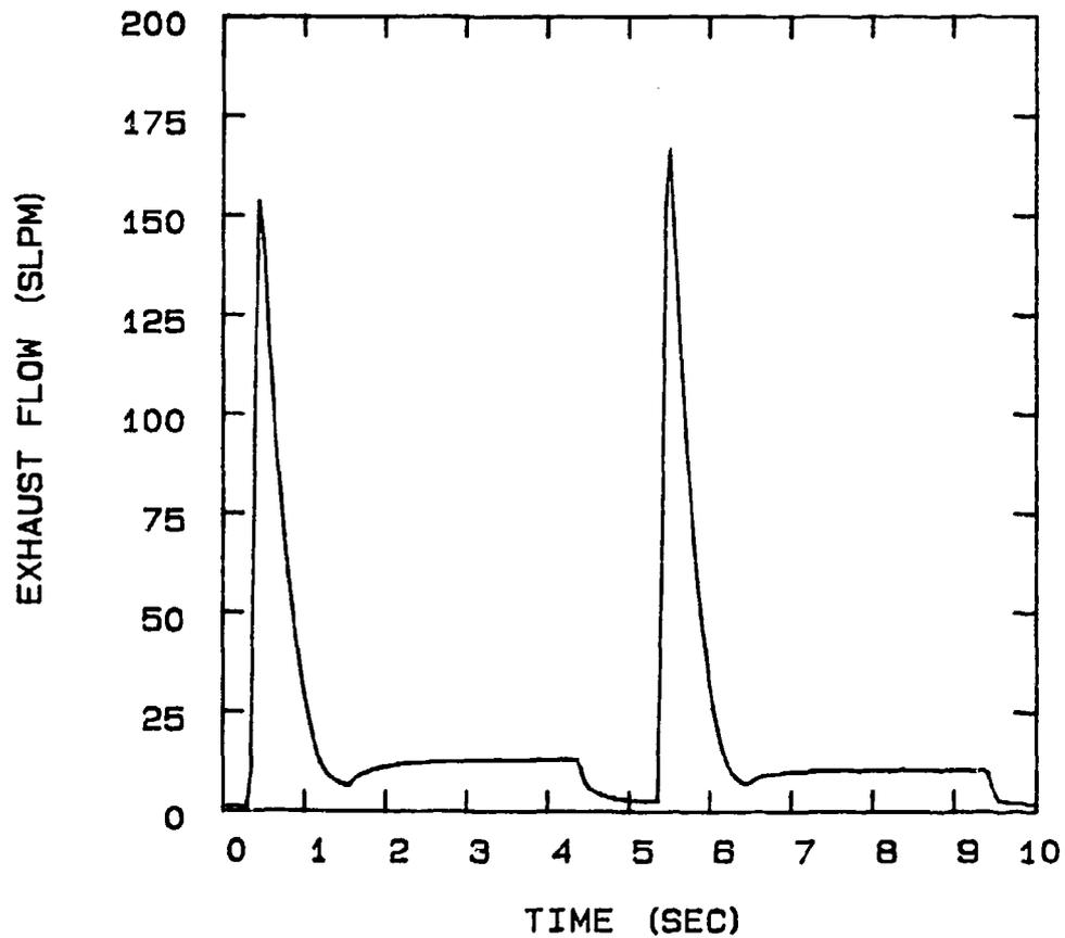
FIG 5-99. EXHAUST FLOW FOR PSA UNIT CONFIGURATION:
