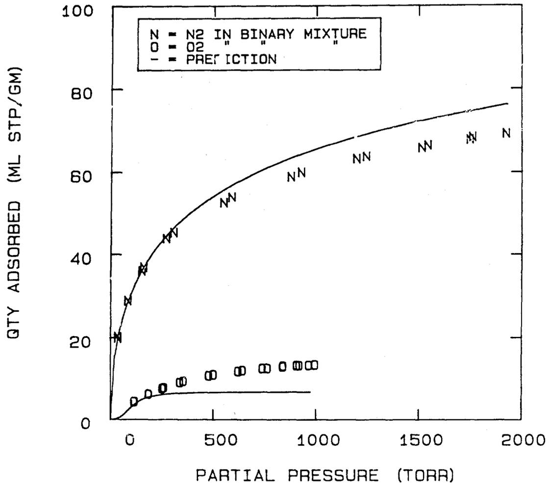
FIG 5-60. PREDICTION OF N<sub>2</sub>-O<sub>2</sub> SORPTION ON MOLECULAR SIEVE 5A AT -70°C USING THE IDEAL ADSORBED SOLUTION THEORY.
