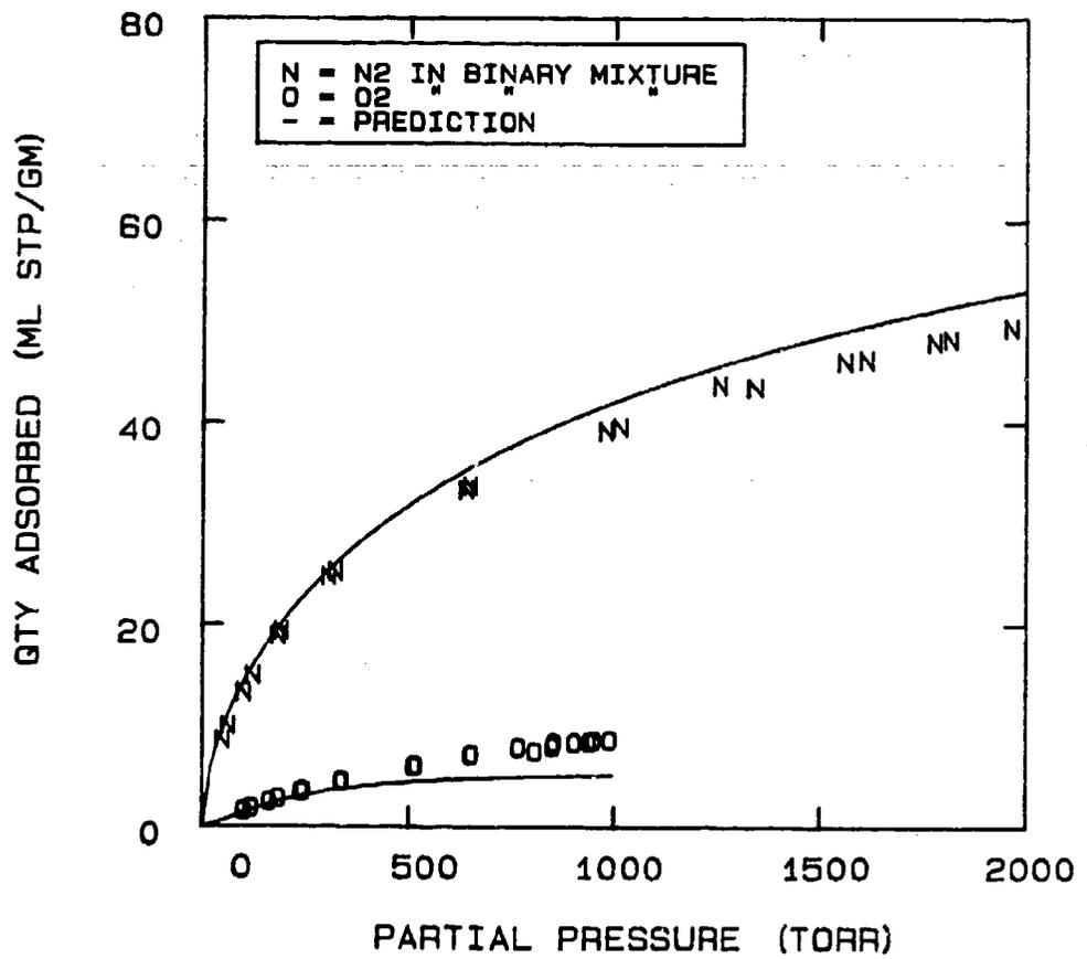
FIG 5-59. PREDICTION OF N<sub>2</sub>-O<sub>2</sub> SORPTION ON MOLECULAR SIEVE 5A AT -40°C USING THE IDEAL ADSORBED SOLUTION THEORY.
