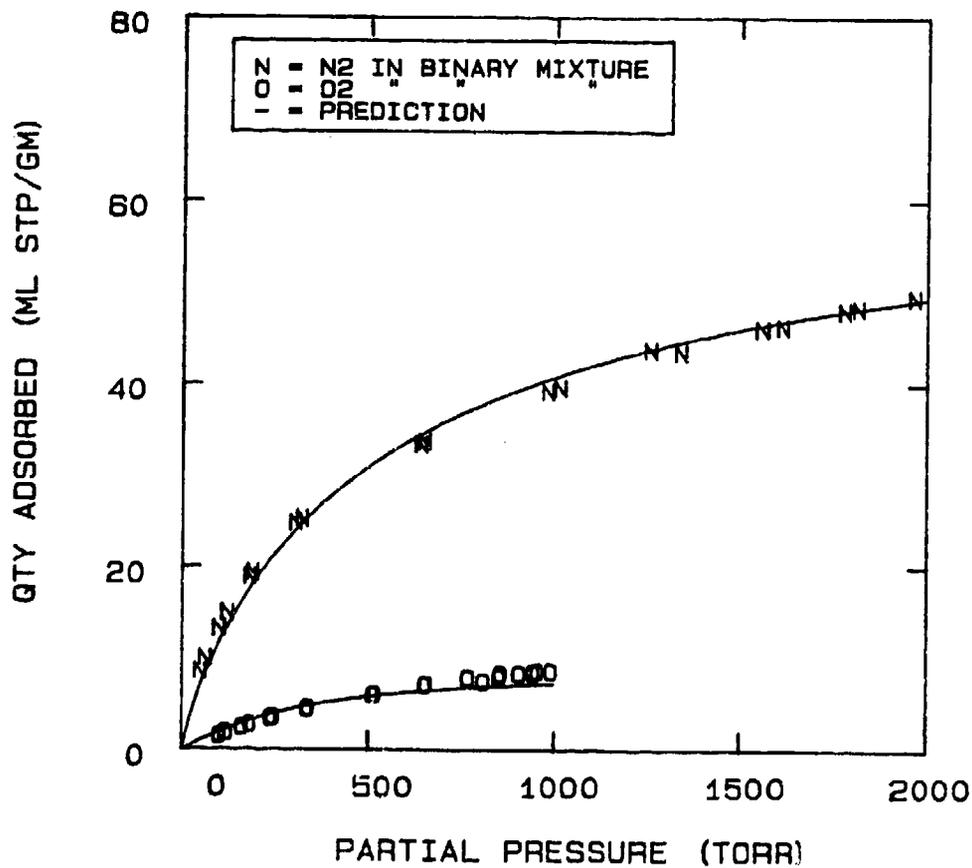
FIG 5-55. PREDICTION OF N<sub>2</sub>-O<sub>2</sub> SORPTION AT -40°C USING A STATISTICAL THERMODYNAMIC MODEL WITH ADJUSTED EFFECTIVE MOLECULAR VOLUMES (B<sub>O<sub>2</sub></sub> = 28, B<sub>N<sub>2</sub></sub> = 82.5) .
