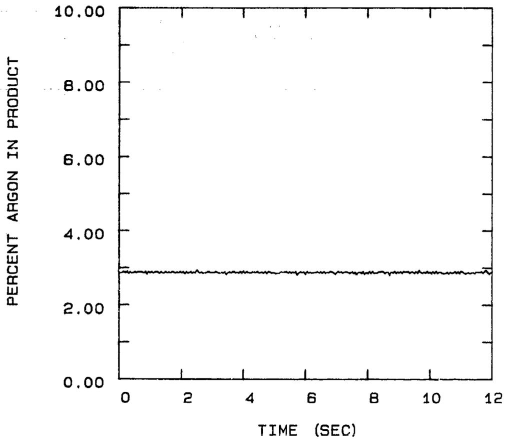
FIG 5-87. PRODUCT AR FROM THE PSA UNIT OPERATING AT  $-40^{\circ}\text{C}$  AND CONFIGURED FOR A 2 STEP CYCLE, 6 SEC. CYCLE TIME, 0.020" PURGE ORIFICE, AND 100 SCCM PRODUCT FLOW.
