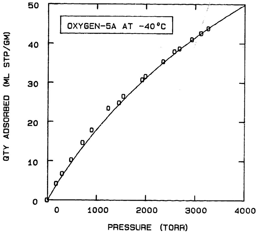
FIG 5-28. CORRELATION OF OXYGEN SORPTION ON MOLECULAR SIEVE 5A AT  $-40^{\circ}\text{C}$  USING A STATISTICAL THERMODYNAMIC MODEL WHERE:  $K = 0.002031$ ,  $B = 38.8$ , AND  $m = 20$ .
