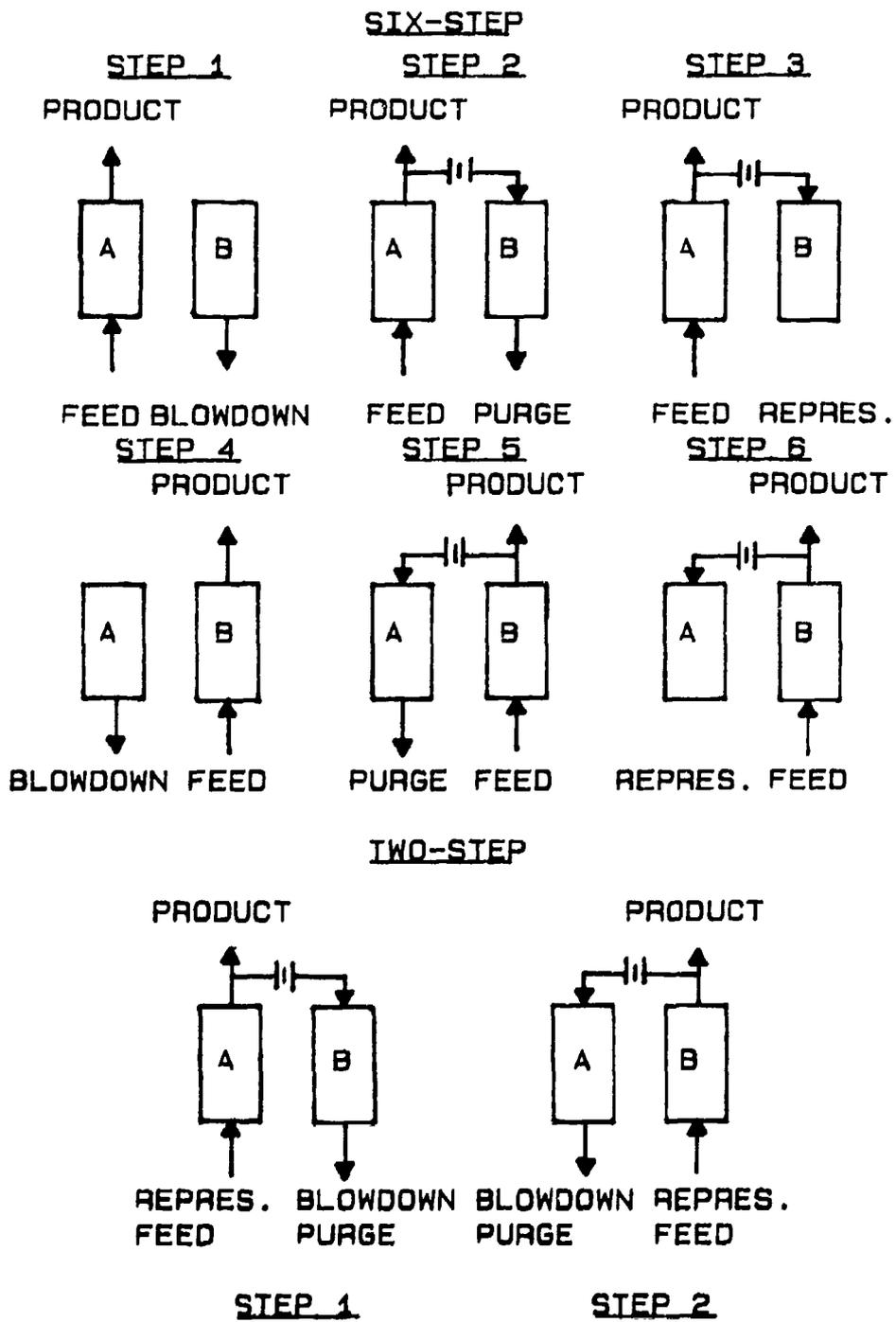
FIG 3-4. COMPARISON OF SIX-STEP AND TWO-STEP CYCLE.
