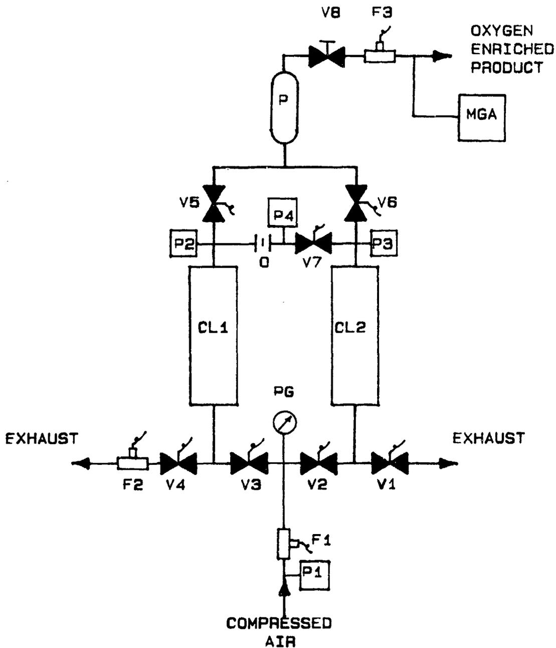
FIG 4-11. PSA AIR SEPARATION UNIT. F1-3. MASS FLOWMETERS, V1-7. SOLENOID VALVES, V8. MANUAL VALVE, P. PLENUM, MGA. MEDICAL GAS ANALYZER, P1-4. PRESSURE TRANSDUCERS, O. ORIFICE, CL1-2. COLUMNS OF MOLECULAR SIEVE, AND PG. PRESSURE GAUGE.
