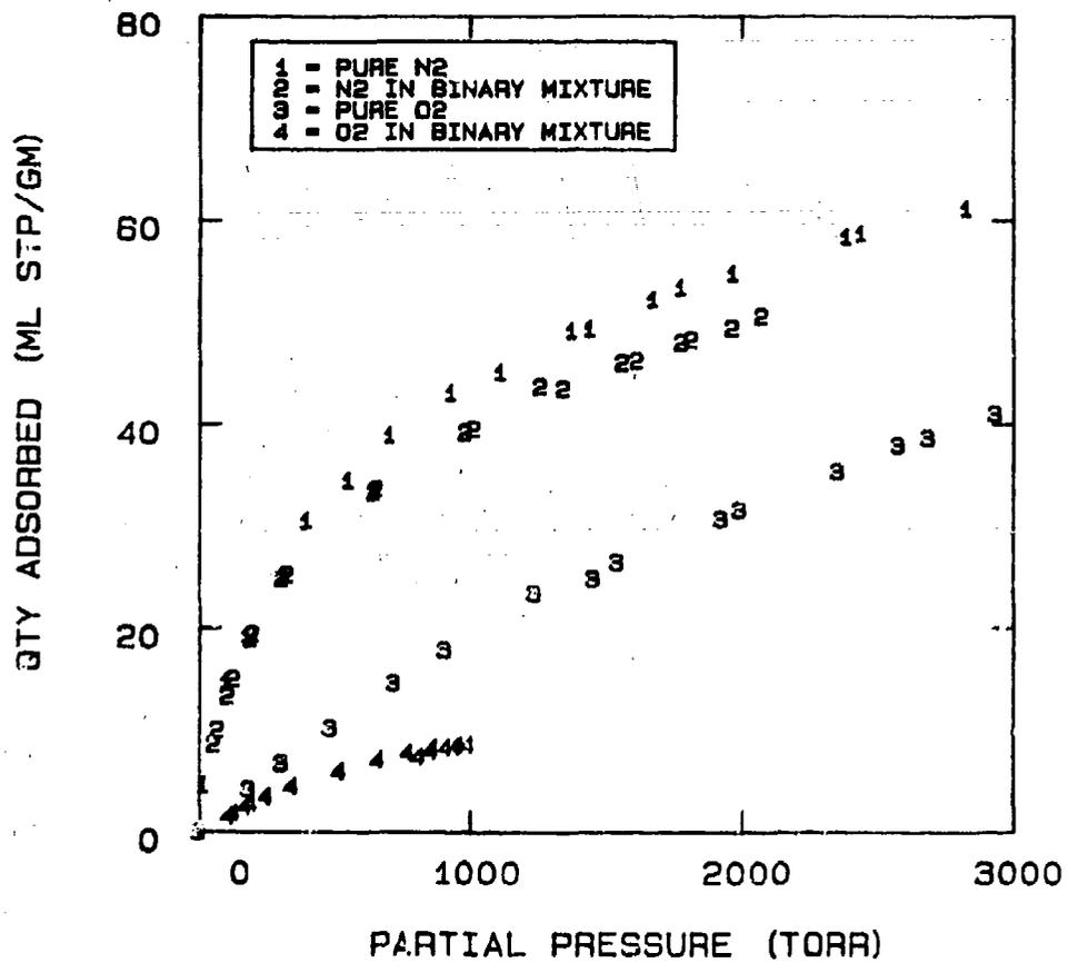
FIG 5-49. PURE AND MULTICOMPONENT DATA OF NITROGEN AND OXYGEN ON MOLECULAR SIEVE 5A AT -40°C.
