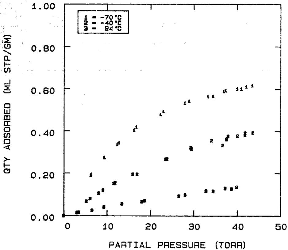
FIG 5-47. ARGON LOADING AT 24, -40, AND -70°C FOR THE AIR-5A SYSTEM.
