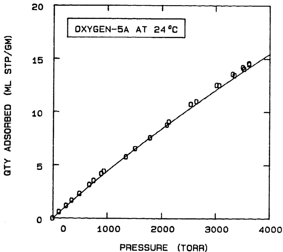
FIG 5-27. CORRELATION OF OXYGEN SORPTION ON MOLECULAR SIEVE 5A AT 24°C USING A STATISTICAL THERMODYNAMIC MODEL WHERE:  $K = 0.0004234$ ,  $B = 38.8$ , AND  $m = 20$ .
