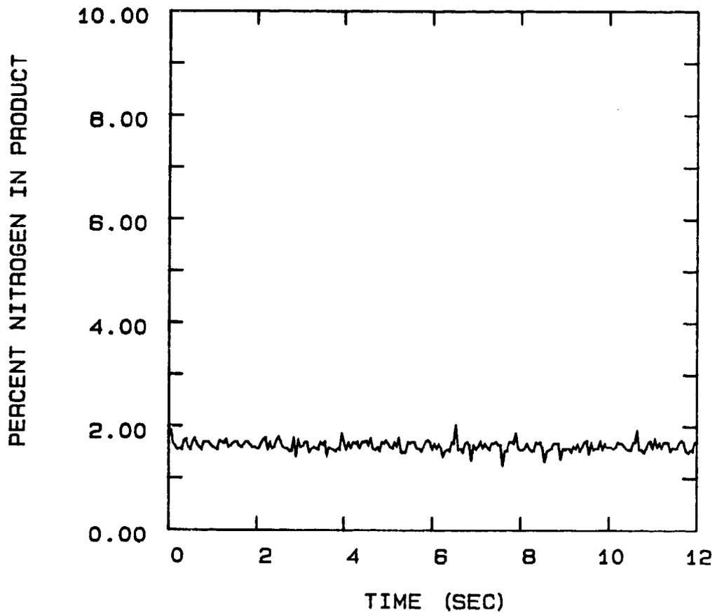
FIG 5-82. PRODUCT N2 FROM THE PSA UNIT OPERATING AT 24 °C AND CONFIGURED FOR A 2 STEP CYCLE, 6 SEC. CYCLE TIME, 0.020" PURGE ORIFICE, AND 100 SCCM PRODUCT FLOW.
