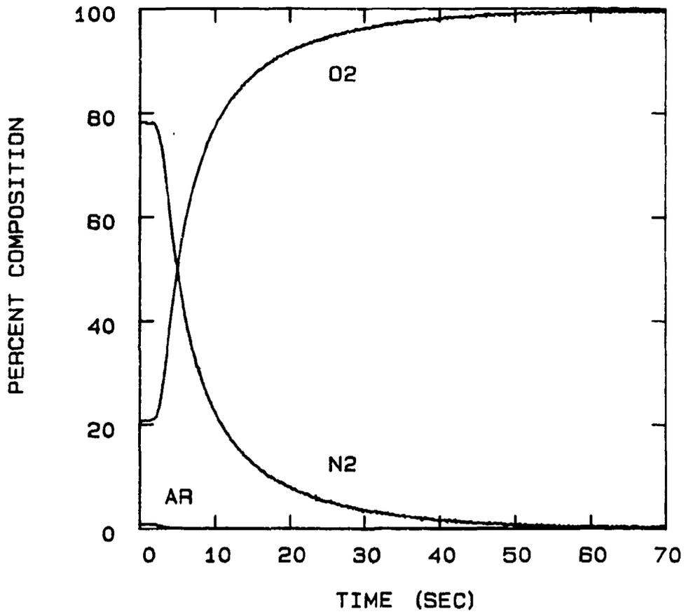
FIG 5-68. RUN 110412 : COLUMN OXYGEN BREAKTHROUGH AT -40°C, 25 SLPM, AND BED PRESSURE OF APPROXIMATELY 18.5 PSIA.
