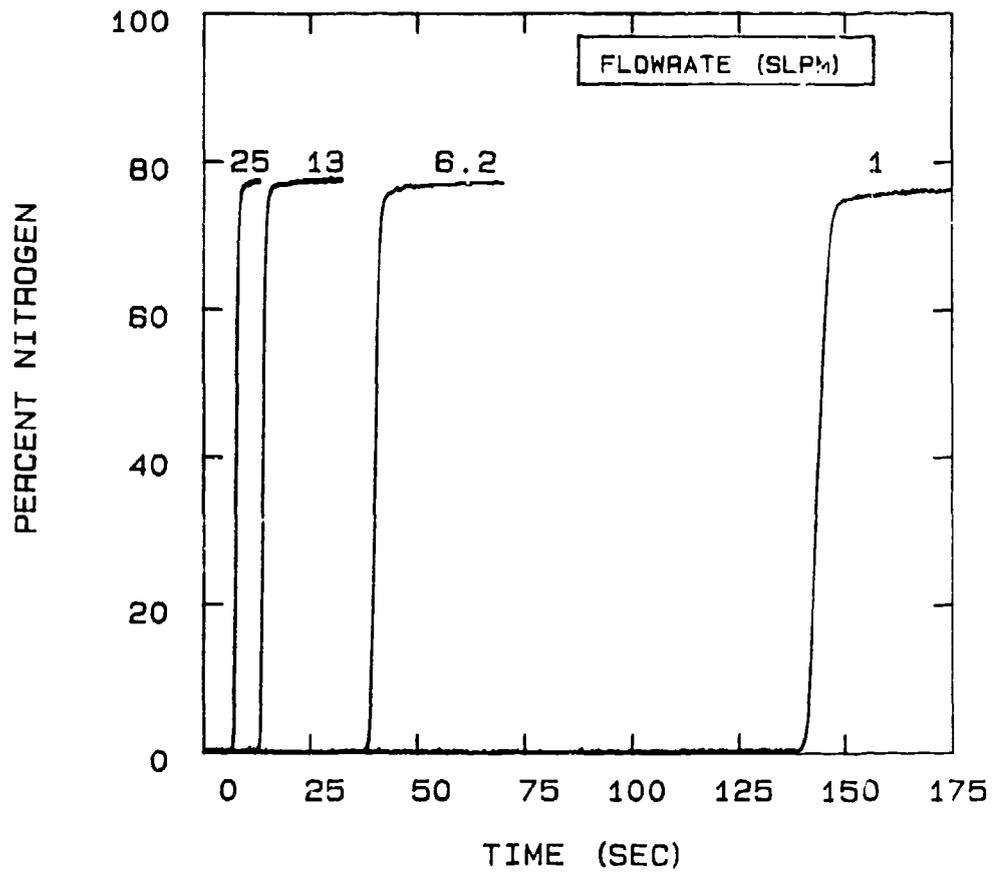
FIG 5-72. DEPENDENCE OF NITROGEN BREAKTHROUGH ON FLOWRATE AT  $-40^{\circ}\text{C}$  AND BED PRESSURE OF 25 PSIA.
