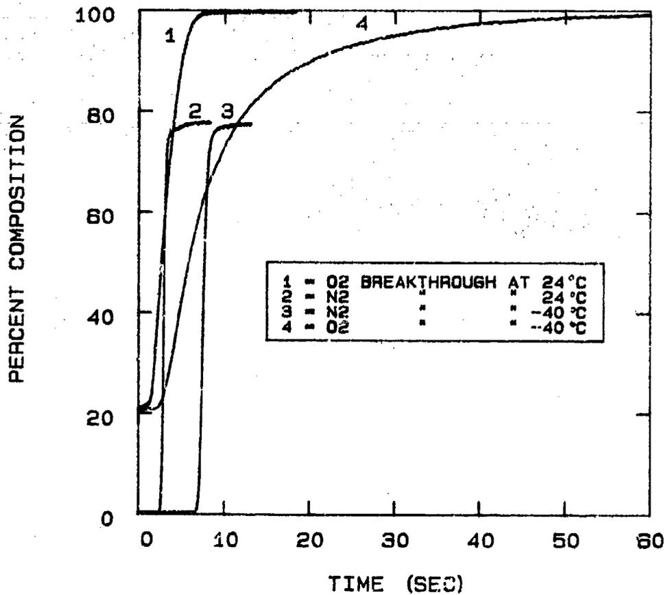
FIG 5-74. EFFECT OF TEMPERATURE ON NITROGEN AND OXYGEN BREAKTHROUGH FOR A FLOWRATE OF 25 SLPM AND BED PRESSURE OF 25 PSIA.
