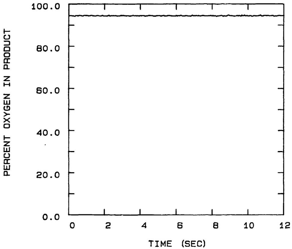
FIG 5-84. PRODUCT O<sub>2</sub> FROM THE PSA UNIT OPERATING AT 24°C AND CONFIGURED FOR A 2 STEP CYCLE, 6 SEC. CYCLE TIME, 0.020" PURGE ORIFICE, AND 100 SCCM PRODUCT FLOW.
