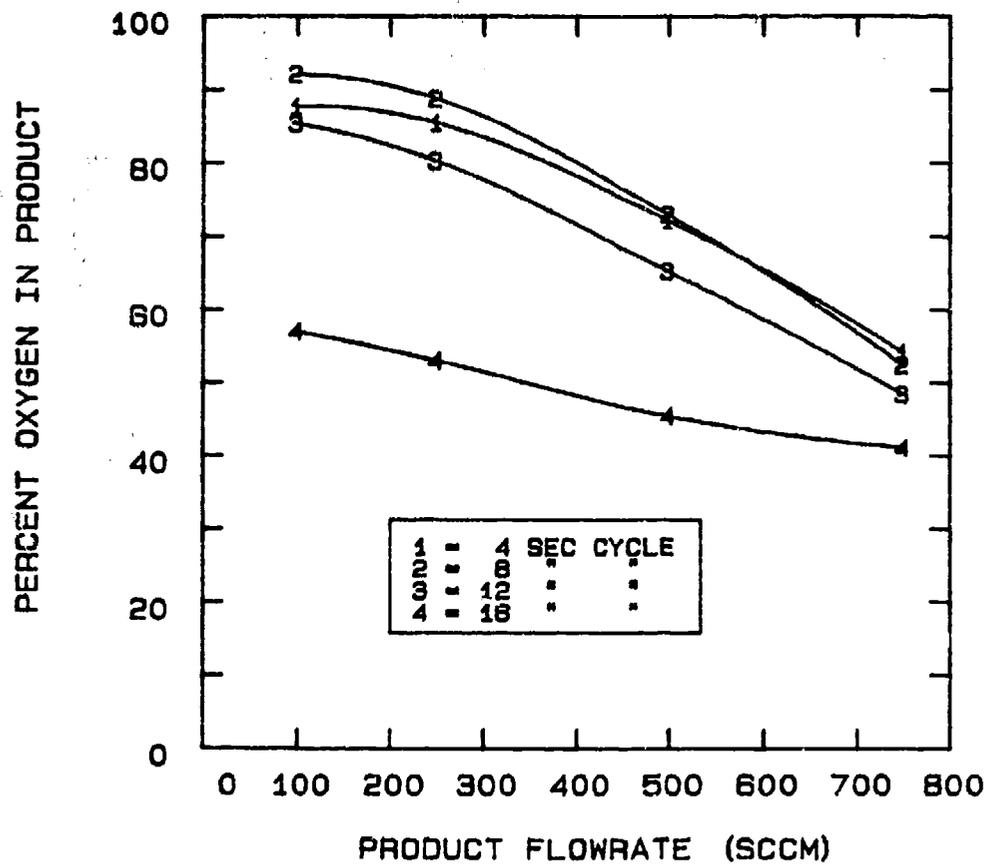
FIG 5-84. EFFECT OF PRODUCT FLOWRATE AND CYCLE TIME ON THE PSA UNIT OPERATING AT 24°C AND CONFIGURED FOR 2 STEPS/CYCLE AND 0.020" PURGE ORIFICE.
