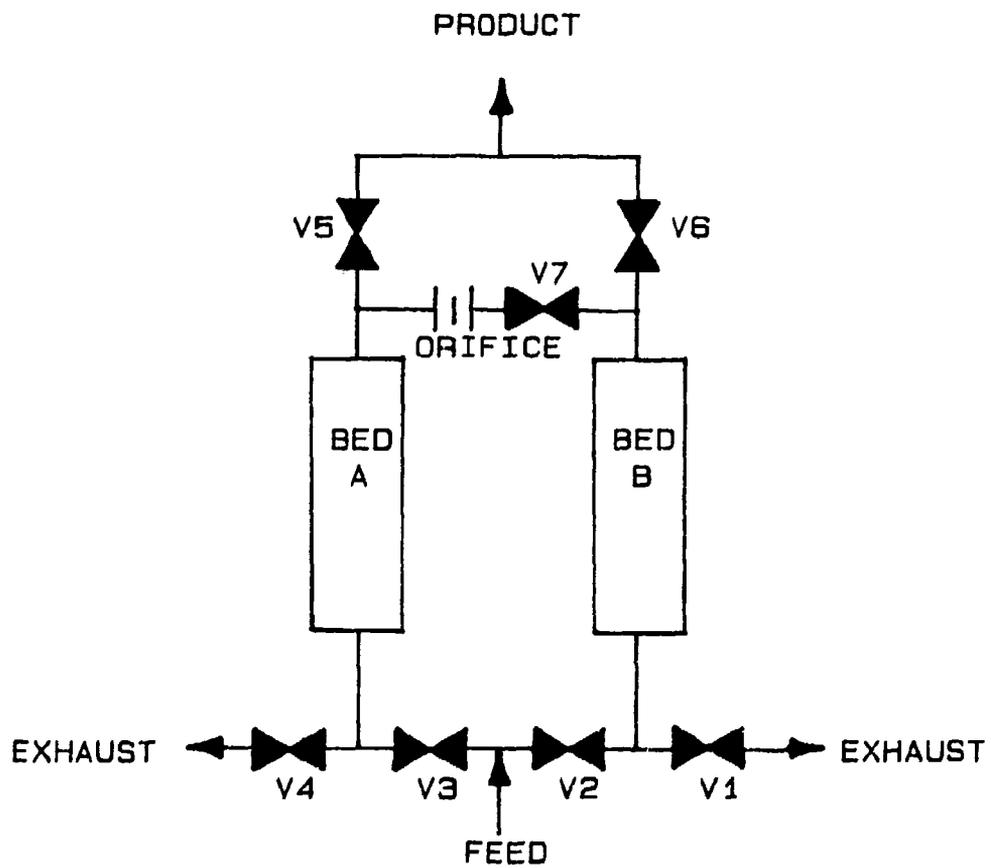
FIG 3-2. SIMPLIFIED SCHEMATIC DIAGRAM OF A DUAL COLUMN PSA AIR SEPARATION UNIT.
