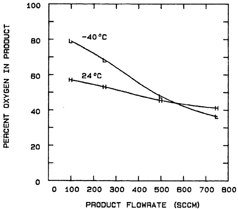
FIG 5-93. EFFECT OF PRODUCT FLOWRATE AND TEMPERATURE ON THE PSA UNIT CONFIGURED FOR 2 STEPS/CYCLE, 16 SEC. CYCLE TIME, AND 0.020" ORIFICE.
