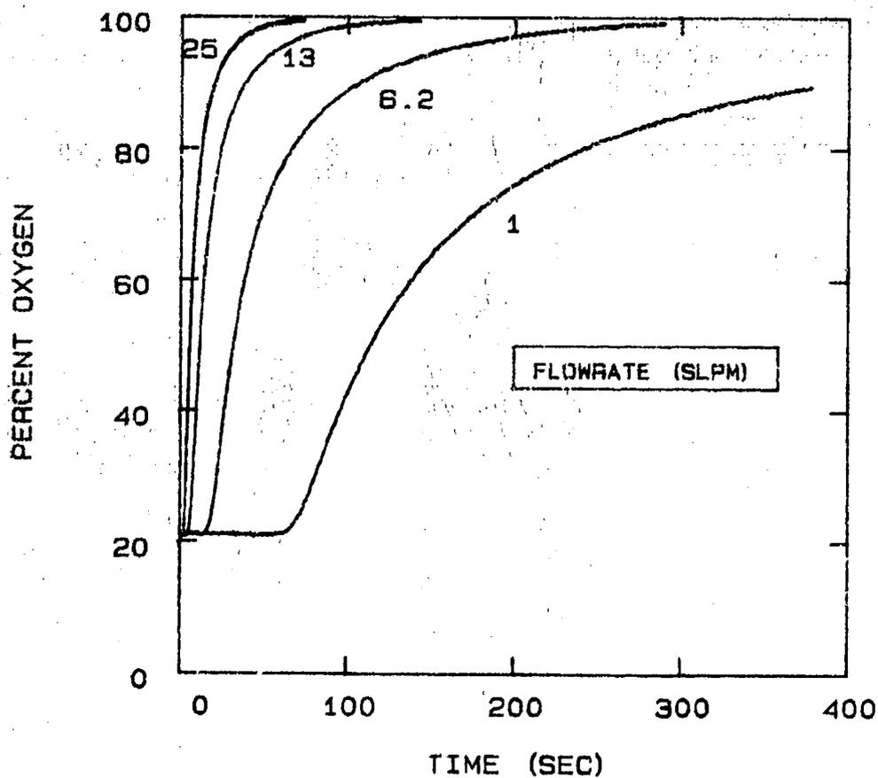
FIG 5-73. DEPENDENCE OF OXYGEN BREAKTHROUGH ON FLOWRATE AT  $-40^{\circ}\text{C}$  AND BED PRESSURE OF 25 PSIA.
