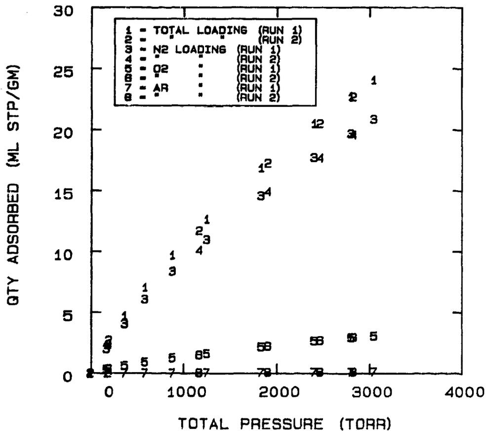
FIG 5-39. AIR-5A AT 24 °C WHERE THE TOTAL MOLAR RATIO OF NITROGEN, OXYGEN, AND ARGON WITHIN THE SYSTEM IS CONSTANT AT 78.14 : 20.92 : 0.94, RESPECTIVELY.
