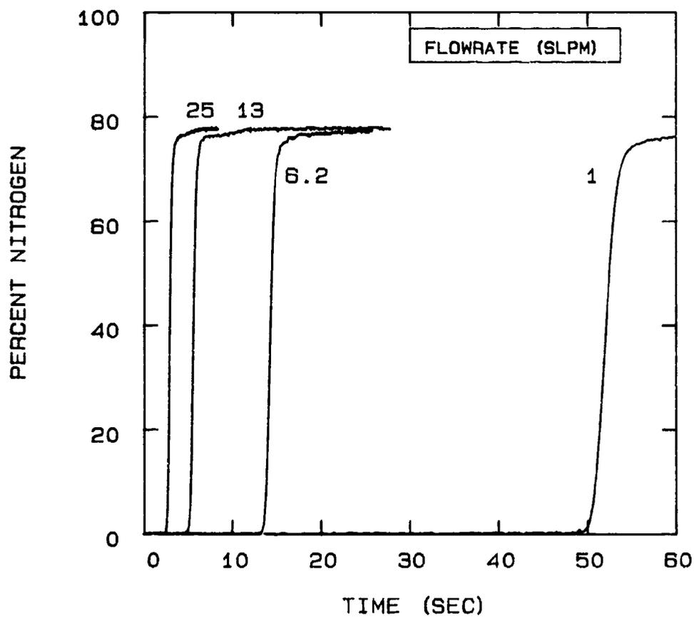
FIG 5-70. DEPENDENCE OF NITROGEN BREAKTHROUGH ON FLOWRATE AT 24°C AND BED PRESSURE OF 25 PSIA.
