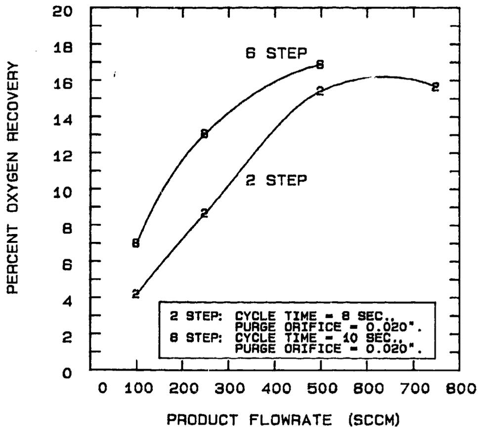
FIG 5-110. COMPARISON OF OXYGEN RECOVERY BETWEEN A 2 STEP AND 6 STEP SYSTEM OPERATING AT 24 °C.
