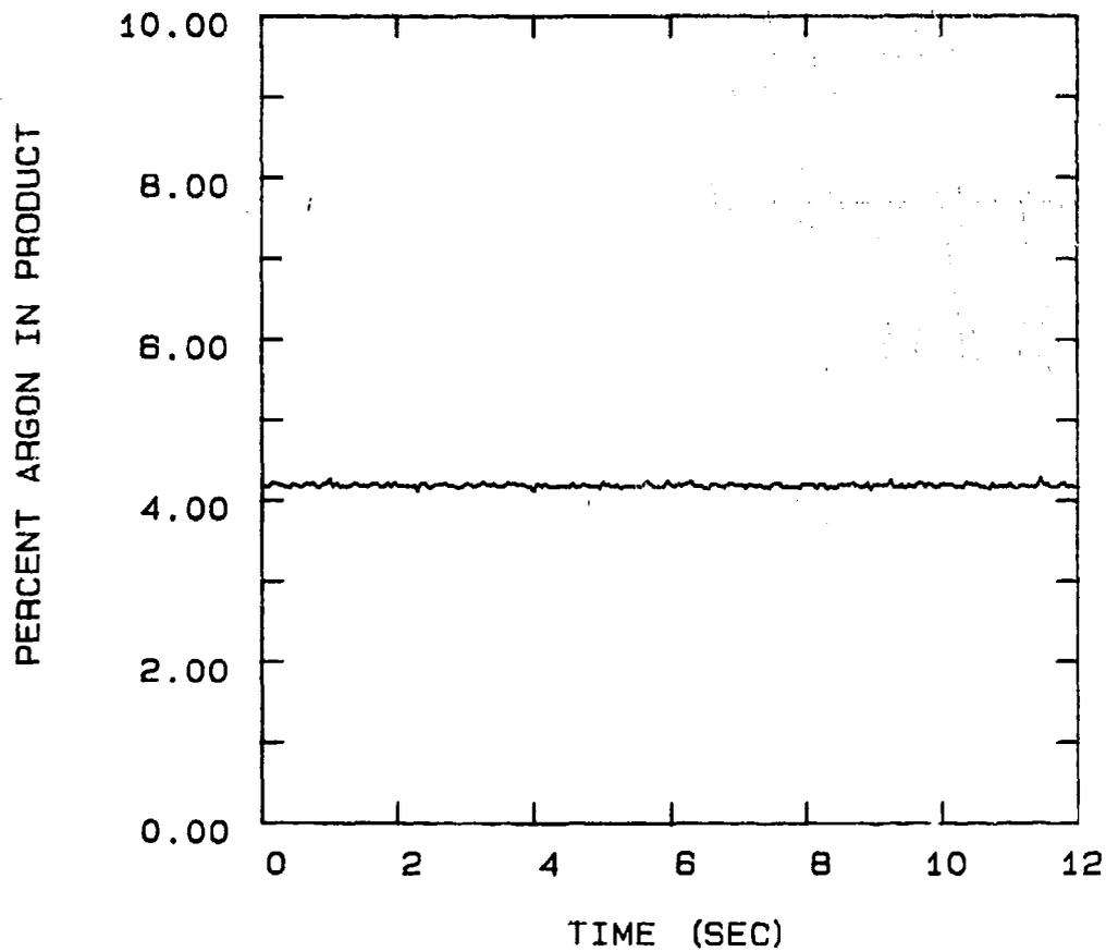
FIG 5-86. PRODUCT AR FROM THE PSA UNIT OPERATING AT 24°C AND CONFIGURED FOR A 2 STEP CYCLE, 6 SEC. CYCLE TIME, 0.020" PURGE ORIFICE, AND 100 SCCM PRODUCT FLOW.
