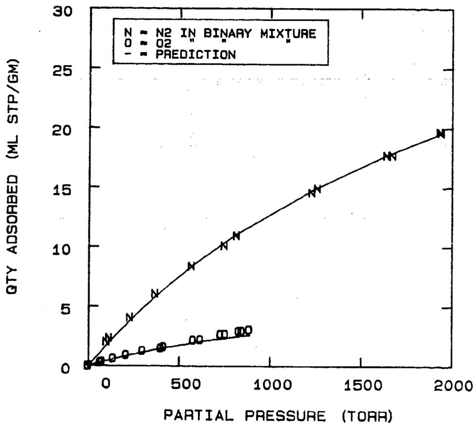
FIG 5-52. PREDICTION OF NITROGEN-OXYGEN ADSORPTION ON MOLECULAR SIEVE 5A AT 24°C USING A STATISTICAL THERMODYNAMIC MODEL WITH PURE COMPONENT PARAMETERS.
