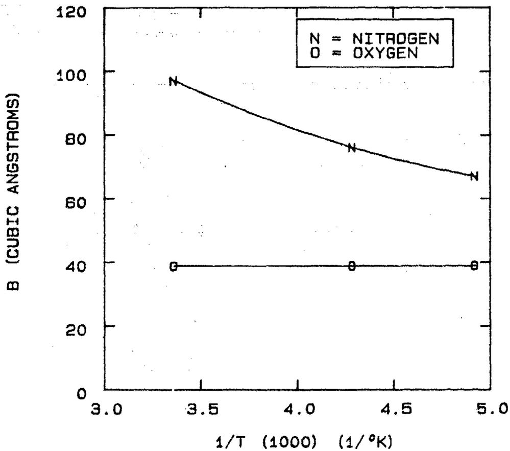
FIG 5-33. TEMPERATURE DEPENDENCE OF THE APPARENT EFFECTIVE MOLECULAR VOLUME FOR PURE NITROGEN AND OXYGEN ON MOLECULAR SIEVE 5A.
