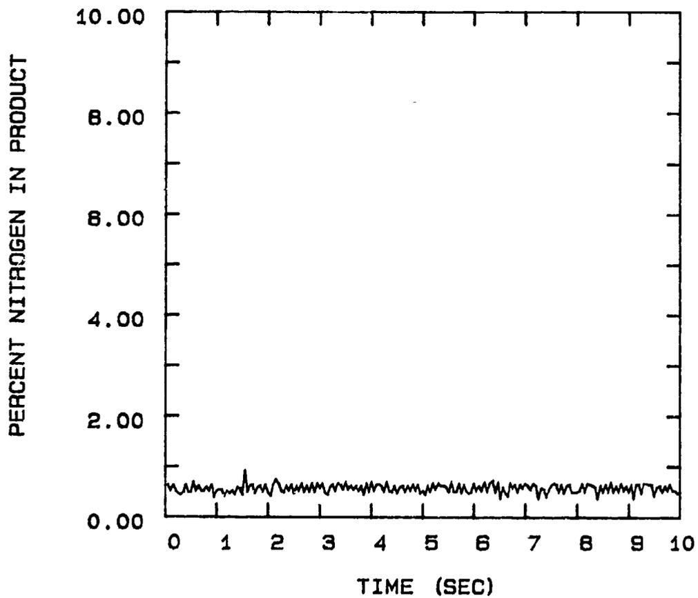
FIG 5-102. PRODUCT N2% FOR PSA UNIT CONFIGURATION:
