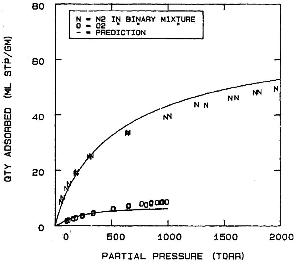
FIG 5-53. PREDICTION OF NITROGEN-OXYGEN ADSORPTION ON MOLECULAR SIEVE 5A AT -40°C USING A STATISTICAL THERMODYNAMIC MODEL WITH PURE COMPONENT PARAMETERS.
