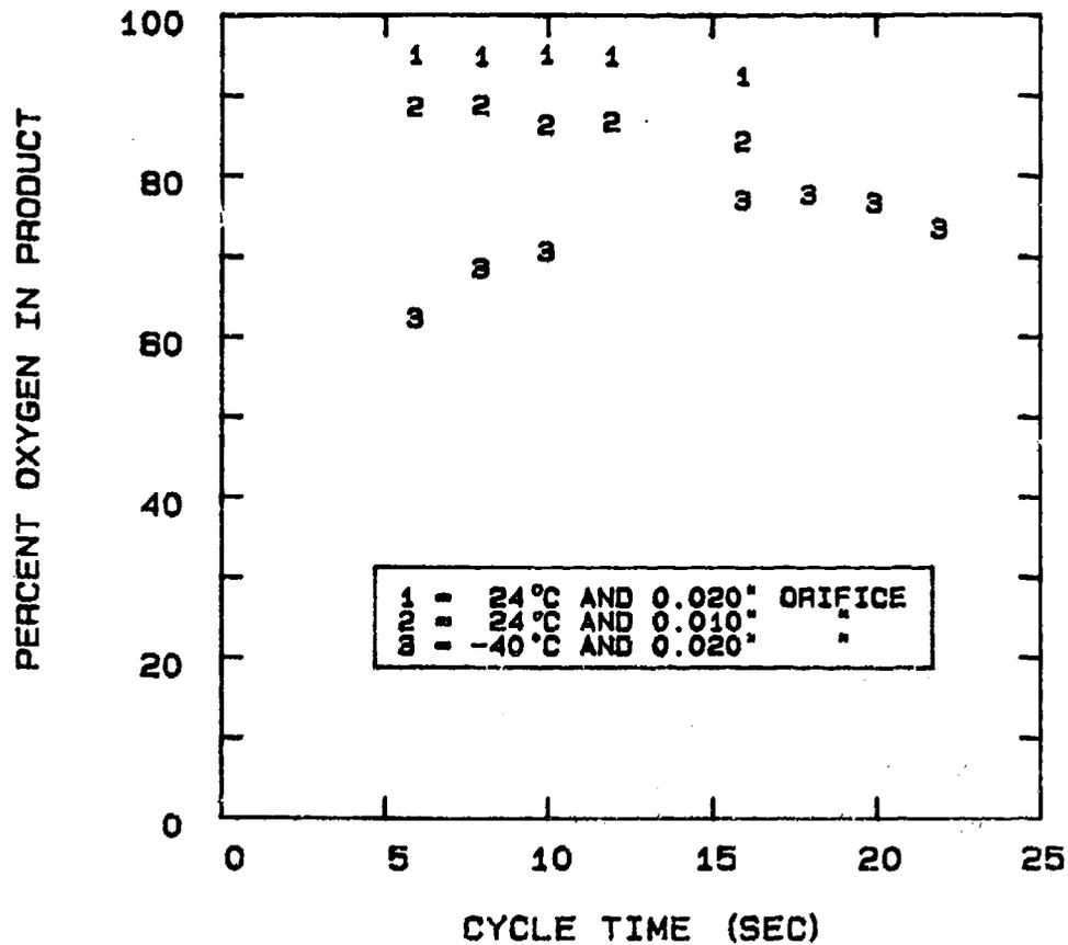
FIG 5-108. EFFECT OF CYCLE TIME AND TEMPERATURE ON THE PSA UNIT CONFIGURED FOR 8 STEP OPERATION AND 100 SCCM PRODUCT FLOW.
