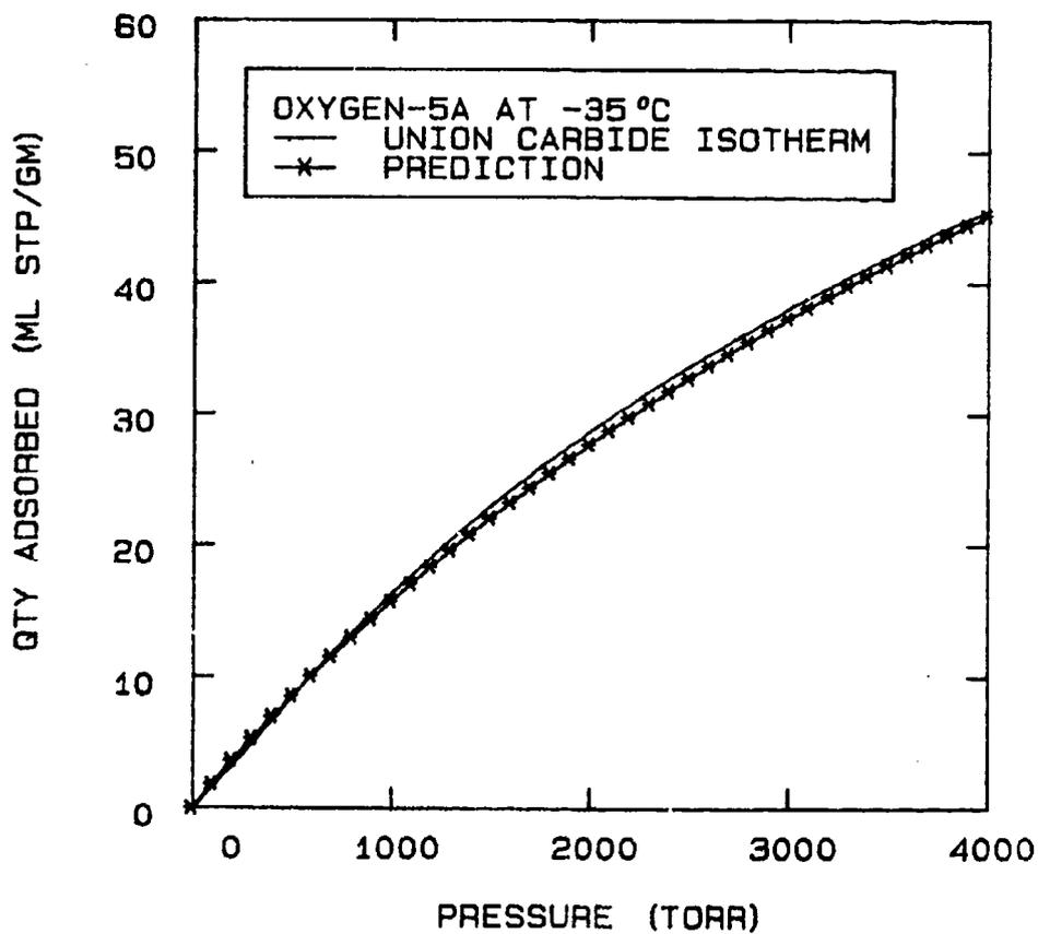
FIG 5-35. PREDICTION OF UNION CARBIDE DATA FOR OXYGEN-5A SORPTION AT -35 °C USING A STATISTICAL THERMODYNAMIC MODEL WHERE:  $K=0.001735$ ,  $B=38.8$ ,  $m=20$ .
