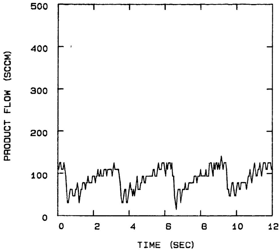
FIG 5-80. PRODUCT FLOW FROM THE PSA UNIT OPERATING AT 24°C AND CONFIGURED FOR A 2 STEP CYCLE, 6 SEC CYCLE TIME, 0.020" PURGE ORIFICE, AND 100 SCCM PRODUCT FLOW.
