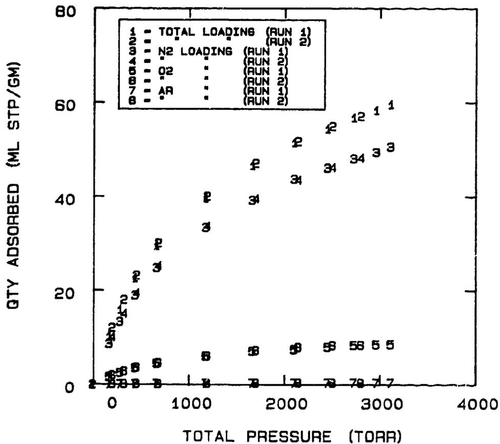
FIG 5-40. AIR-5A AT  $-40^{\circ}\text{C}$  WHERE THE TOTAL MOLAR RATIO OF NITROGEN, OXYGEN, AND ARGON WITHIN THE SYSTEM IS CONSTANT AT 78.14 : 20.92 : 0.94, RESPECTIVELY.
