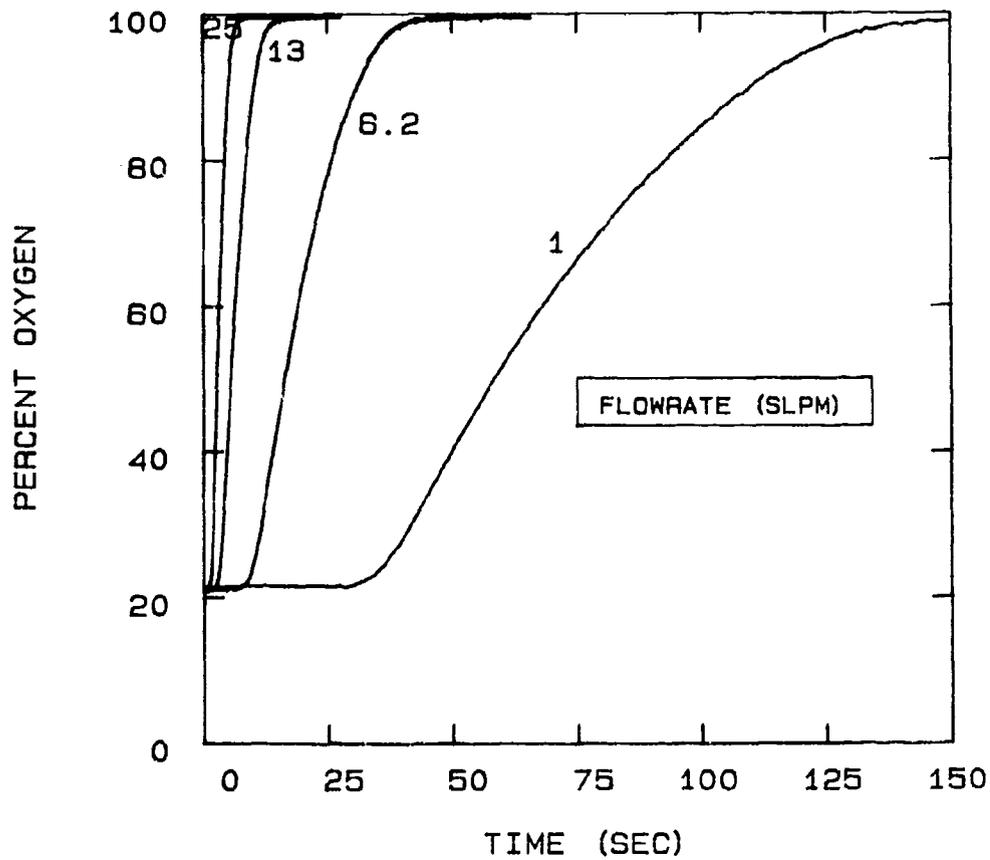
FIG 5-71. DEPENDENCE OF OXYGEN BREAKTHROUGH ON FLOWRATE AT 24°C AND BED PRESSURE OF 25 PSIA.
