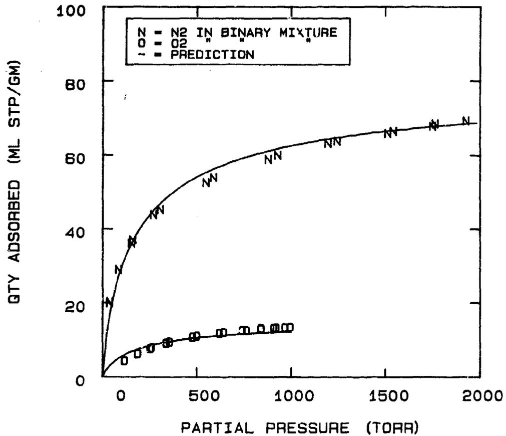
FIG 5-56. PREDICTION OF N2-O2 SORPTION AT -70°C USING A STATISTICAL THERMODYNAMIC MODEL WITH ADJUSTED EFFECTIVE MOLECULAR VOLUMES ( $B_{O_2} = 25$ ,  $B_{N_2} = 74$ ).
