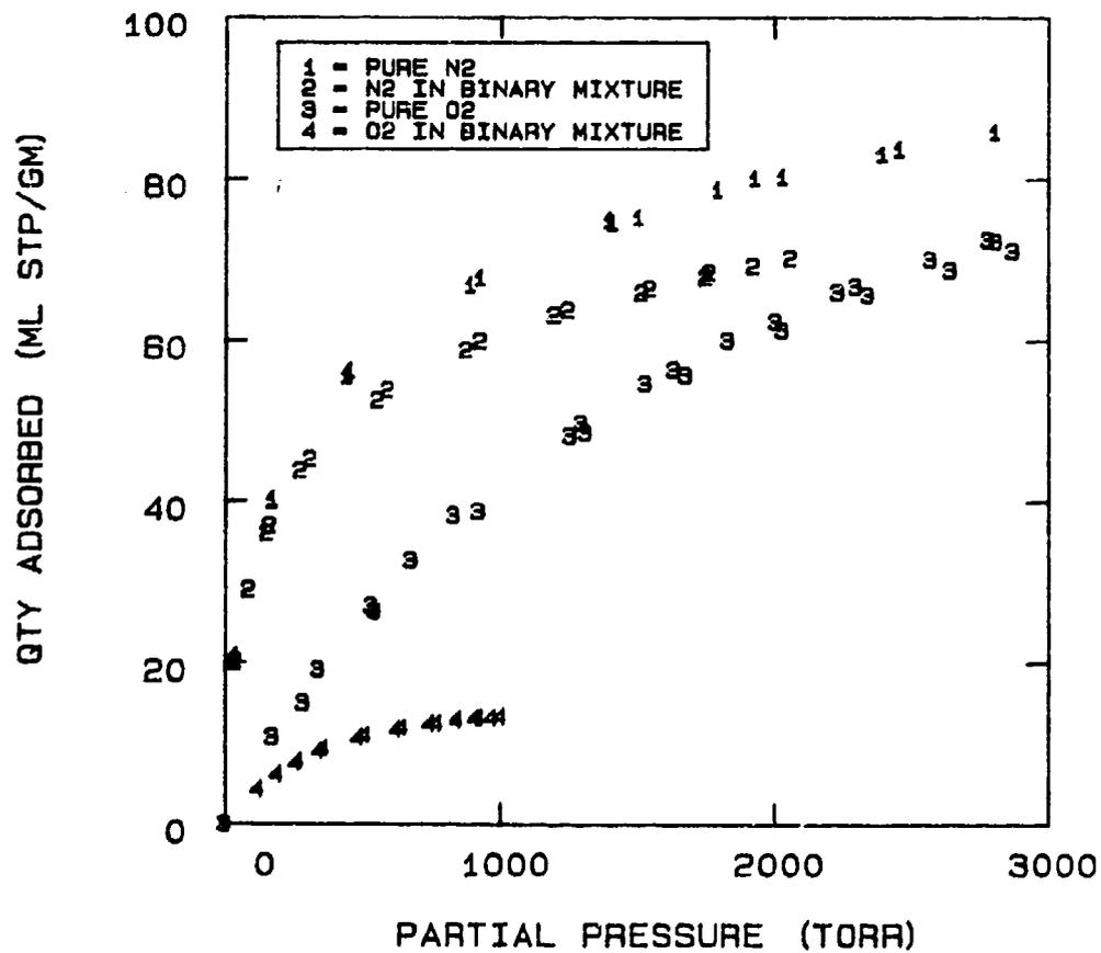
FIG 5-50. PURE AND MULTICOMPONENT DATA OF NITROGEN AND OXYGEN ON MOLECULAR SIEVE 5A AT  $-70^{\circ}\text{C}$ .
