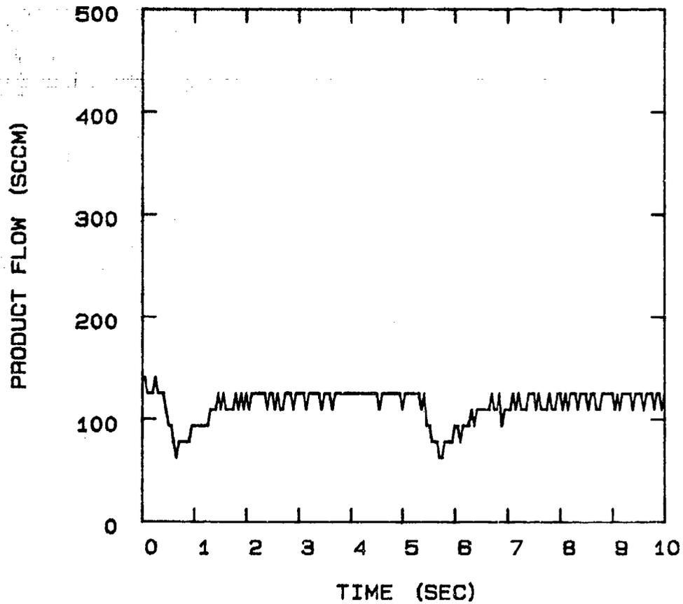
FIG 5-101. PRODUCT FLOW FOR PSA UNIT CONFIGURATION:
