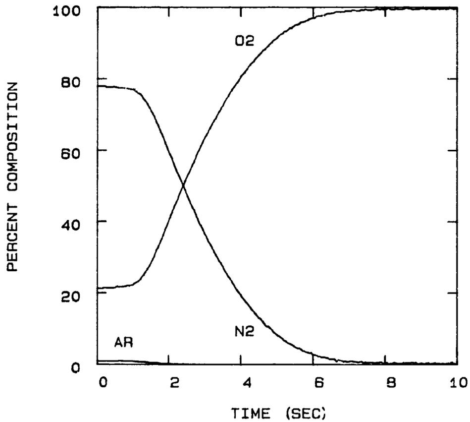
FIG 5-63. RUN 102023 : COLUMN OXYGEN BREAKTHROUGH AT 24°C, 25 SLPM, AND BED PRESSURE OF 25 PSIA.
