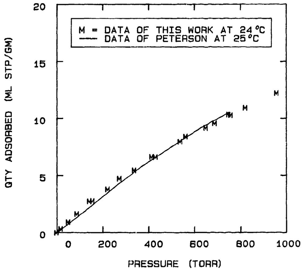
FIG 5-14. NITROGEN ISOOTHERM ON MOLECULAR SIEVE 5A AT 24°C SHOWN WITH THE DATA PETERSON AT 25°C.
