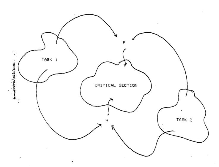
Figure 16-1: Task Communication with Semaphores
