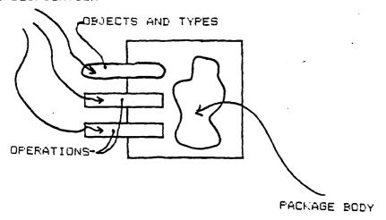
Figure 6-5: Symbol for an Ada Package
