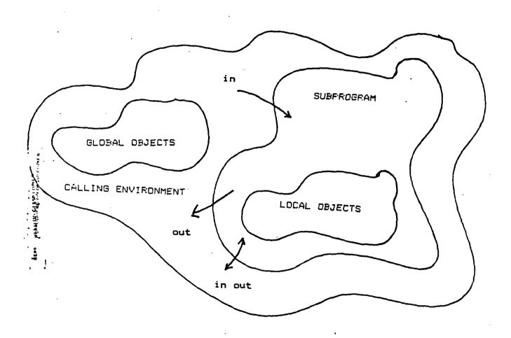
Figure 10-2: Model of an Ada Subprogram
