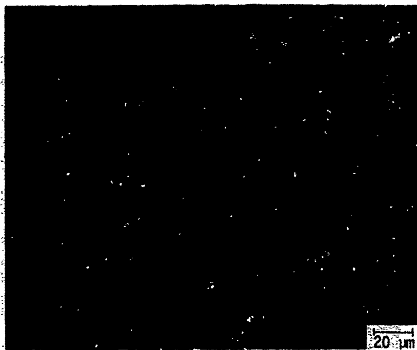
(c) UKAEA/British Nuclear Fuels Refel siliconized SiC; dense interior microstructure of as-processed material, electrolytically etched 3 min with 20% KOH.
