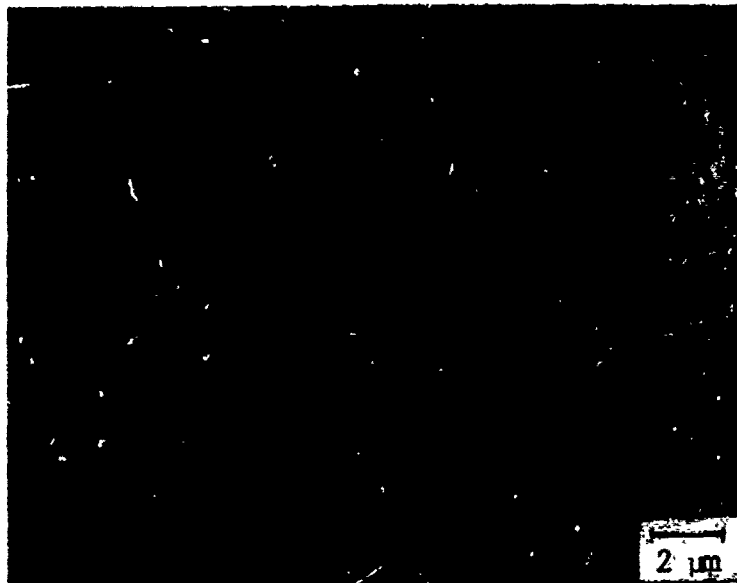
(b) Replica TEM micrograph of Norton NC-132 (1% MgO). Courtesy of K. S. Mazdiasni, AFWAL.
