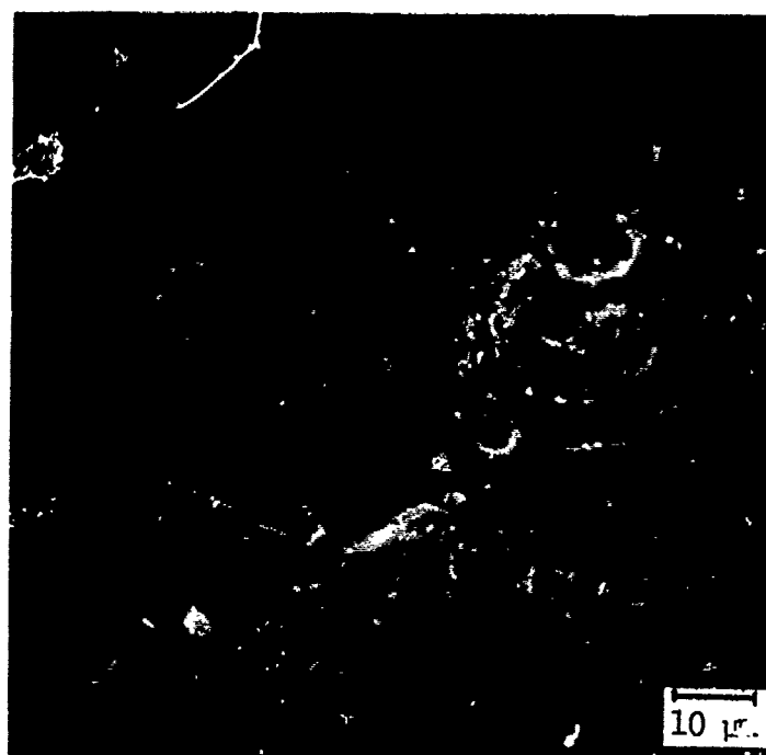
(b) SEM micrograph of sample broken at 25°C (far from the tensile surface).
