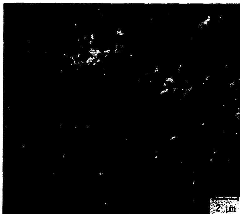
(e) Kyocera SN-3 (4% MgO, 5% Al 2 O 3 ) etched 15 sec at room temperature.
