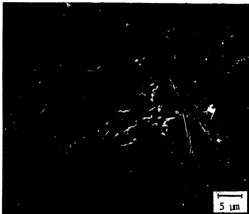
(e) Rocketdyne SN-50 (6% \text{Y}_2\text{O}_3 , 4% \text{Al}_2\text{O}_3 ) etched 9.5 min c
