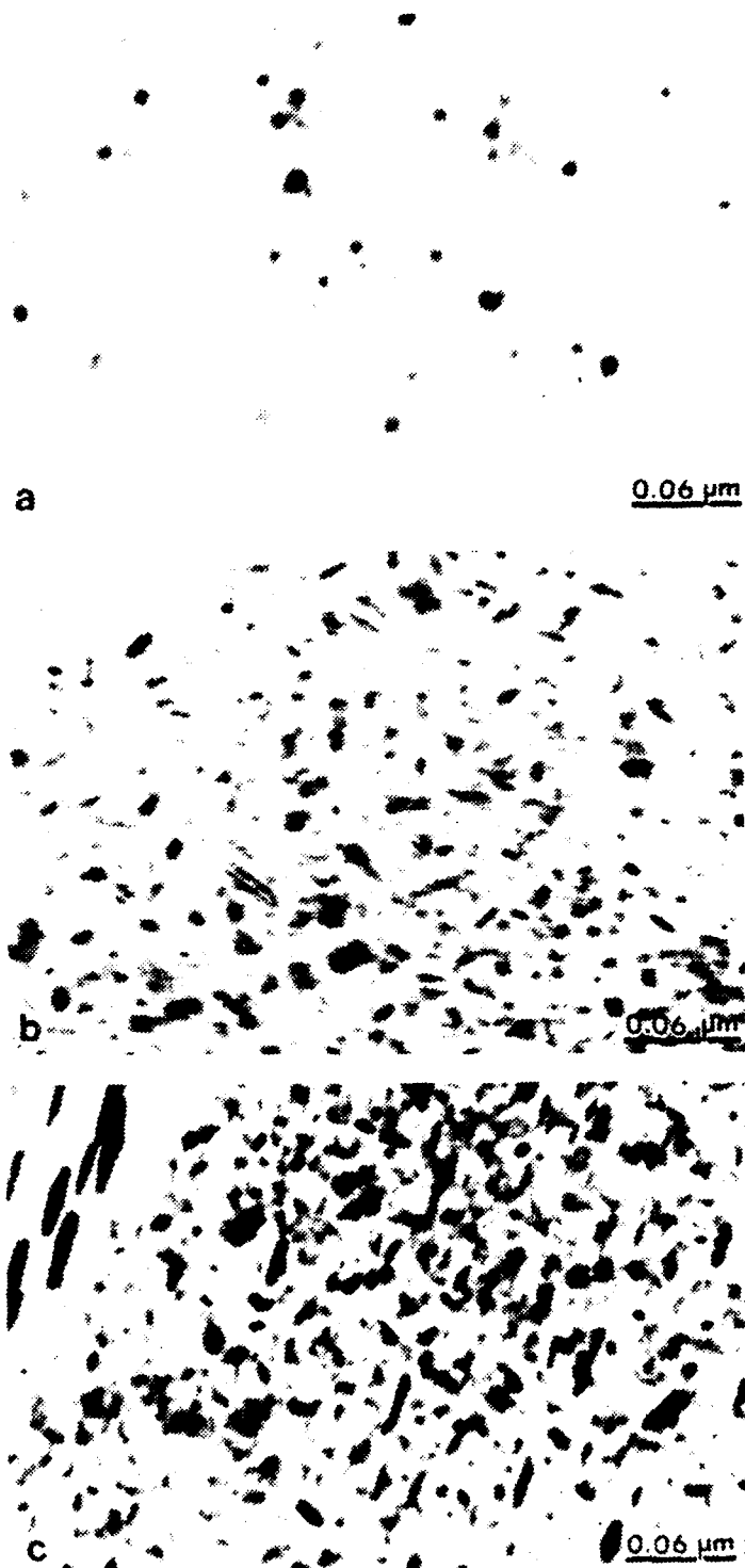
Fig. 4.1. Transmission electron micrographs of a) underaged, b) peak-aged (T6) and c) overaged (T7) I/M 7150 aluminum alloy.
