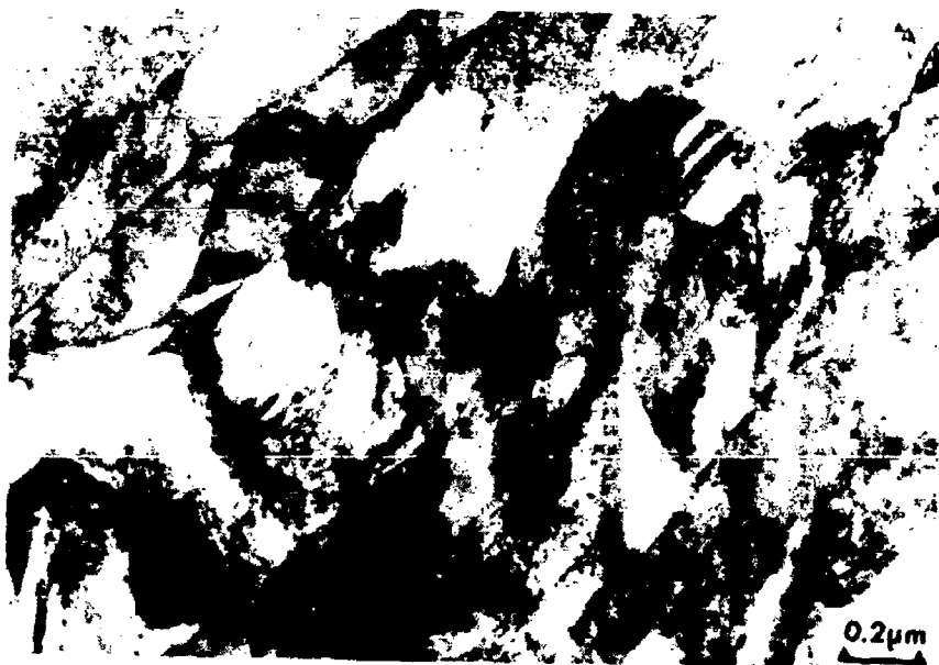
Figure 8. TRANSMISSION ELECTRON MICROGRAPHS SHOWING SUB-STRUCTURE OF PLATE D1 OF Mn-Mo-B STEEL IN THE AS-QUENCHED CONDITION. LONGITUDINAL SECTION.
