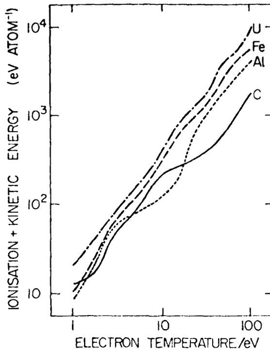
Fig. 20.10 The total (ionisation and kinetic) energy per atom as a function of electron temperature computed from the coronal plasma model of Mosher<sup>18</sup> for four elements.
