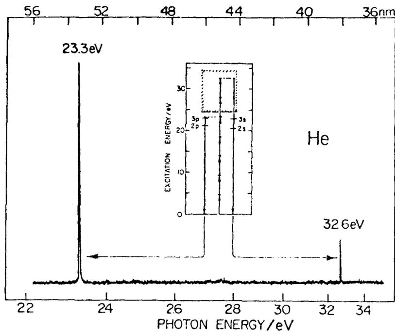
Fig. 20.3 Densitometer tracing of the spectrum of coherent radiation obtained by fifth and seventh order non-linear interactions in He excited by the fourth harmonic of a Nd laser and measured by Reintjes et al<sup>18</sup>. The insert shows the energy levels of helium.
