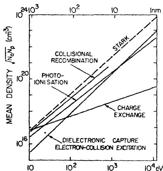
Fig. 20.4 Mean density of ground-state ( $N_0$ ) and pump ( $N_p$ ) particles necessary for laser action with a gain coefficient of five calculated as a function of laser output photon energy for various mechanisms by Elton and his colleagues<sup>6,22</sup>. Stark broadening sets a limit (dashed line) on useful densities.
