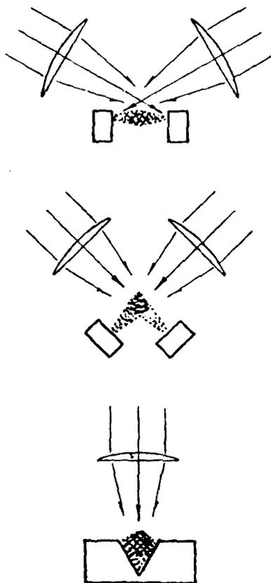
Fig. 20.14 Top and centre: possible configurations for collision of laser-produced plasmas to produce population inversions by charge exchange. One target and laser beam could be replaced with an orifice through which a puff of gas could escape to interact with a plasma. Bottom: related geometry in which a confined and self-colliding plasma is produced by a single laser pulse. Interaction regions, where charge-exchange pumping might occur, are cross-hatched.
