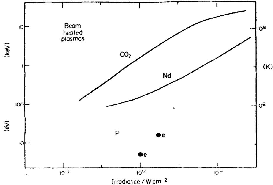
Fig. 20.11 Measured plasma temperatures for the heating of solid targets by  $\text{CO}_2$  and Nd lasers, proton beams and electron beams as a function of irradiance<sup>58</sup>. The energetic ( $\sim \text{MeV}$ ) particle beams are more penetrating than laser pulses so that they heat more matter and yield lower temperatures.
