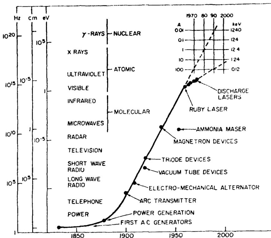
Fig. 20.1 History of the ability to generate coherent electric and electromagnetic waves, as updated<sup>3</sup> from a compilation by Eaglesfield<sup>12</sup>.
