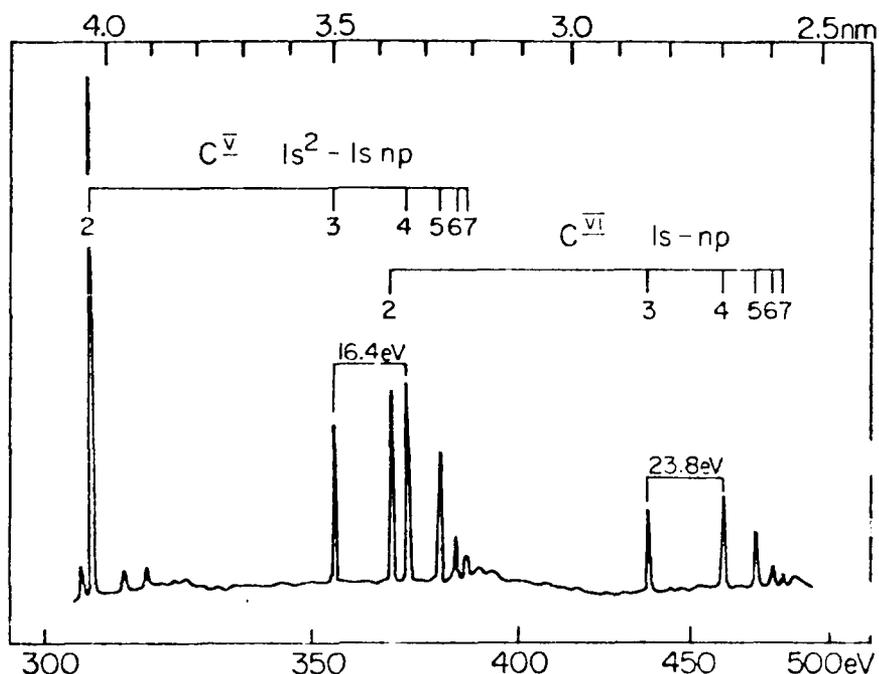
Fig. 20.6 Densitometer trace of the spectrum obtained 18 ns from a laser-heated carbon target with background gas of a few Torr pressure by Dixon and Elton<sup>40</sup>. The energy separation of lines from inverted levels is indicated.
