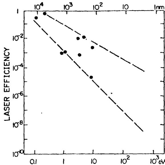
Fig. 20.7 Measured laser efficiencies as a function of laser photon energy plotted by Rhodes and Hoff<sup>20</sup>. The dashed lines indicate a wide region of projected efficiencies for higher-energy lasers.
