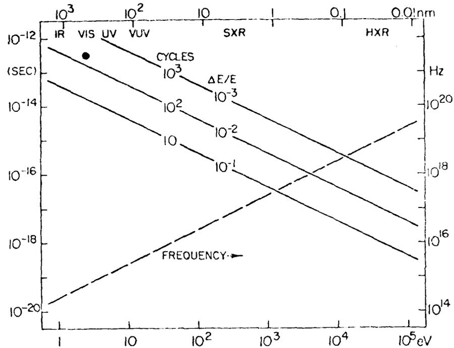
Fig. 20.8 Plot of laser pulse length vs. laser photon energy as a function of the number of cycles in the laser pulse and the relative line width  $\Delta E/E$  from the Uncertainty Principle. The dot indicates the sub-ps pulse length already demonstrated with a Nd laser<sup>50</sup>. The relationship between electromagnetic frequency and photon energy is also given (dashed line).
