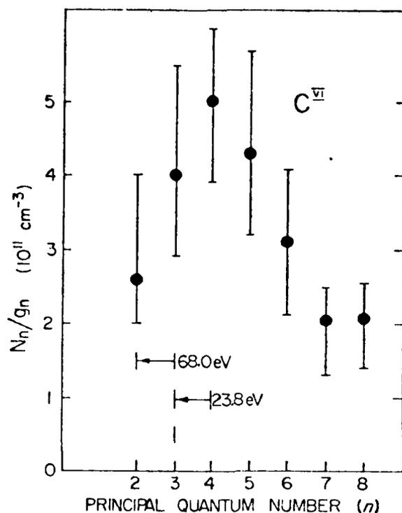
Fig. 20.5 Level population densities obtained by Irons and Peacock<sup>38</sup> from space-resolved spectra 2.8 mm from a laser-heated carbon target. Photon energies between inverted levels are indicated.
