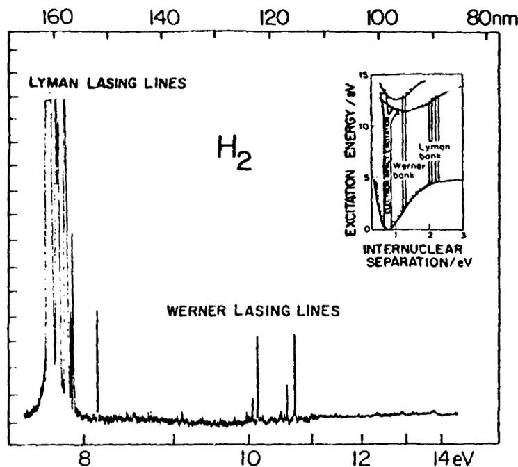
Fig. 20.2 Densitometer tracing of H<sub>2</sub> vacuum-uv laser output obtained by Waynant<sup>16</sup>. The insert shows the transitions in H<sub>2</sub> which produce the Lyman and Werner lines.
