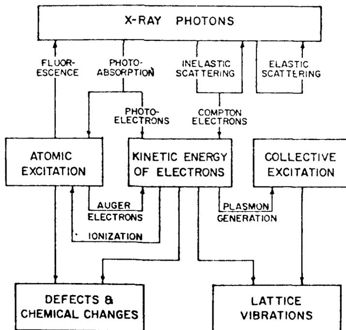
Fig. 20.13 Flow diagram for the photophysical processes by which X-ray photon energy is converted first to electronic vibrations and then to defects, chemical changes and lattice vibrations (heat)<sup>75</sup>.
