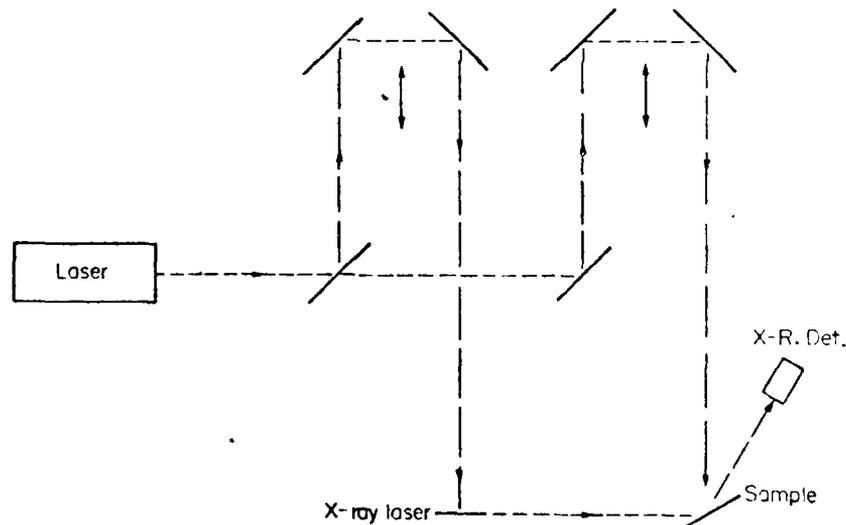
Fig. 20.12 Schematic arrangement for an experiment in which one laser is used to pump an X-ray laser producing a transient effect in a sample (e.g. a shock wave) which is probed by the X-ray laser pulse<sup>68</sup>.
