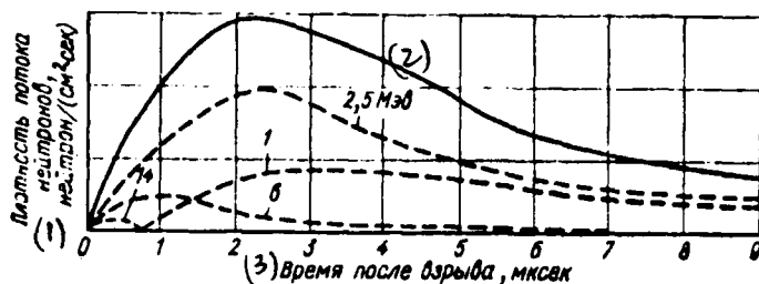
Fig. 1.1. Typical distribution in the time of the neutron flux density of different energy during the thermonuclear blast.
