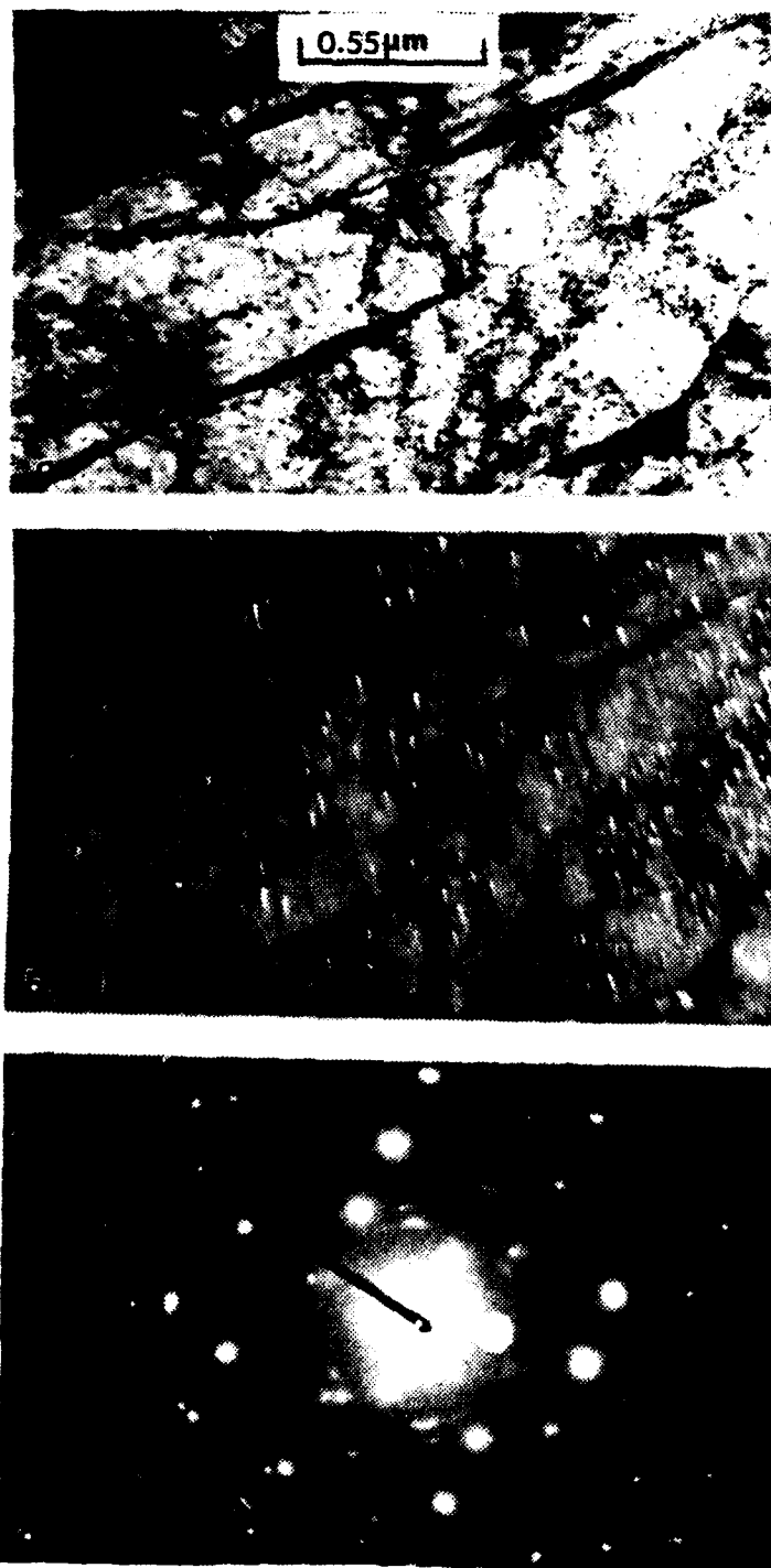
Figure 22 TEM micrograph of SAW upper weld region exhibiting type-II Bainite with fine cementite particles distributed in the ferrite laths: (a) bright field, (b) dark field and (c) corresponding SADP using cementite diffraction spot.
