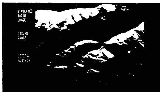
FIGURE 7.3: Simulated radar image: approximated flight path and elevation model serve as input. Ground range presentation and diffuse scattering are assumed.
