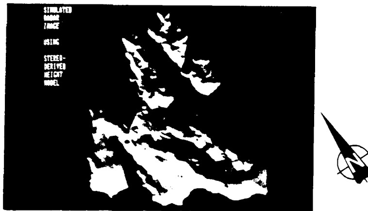
FIGURE 7.8: Simulated radar image using imaging and sensor parameters from the SIR-A recordings and stereo-derived elevation model.
