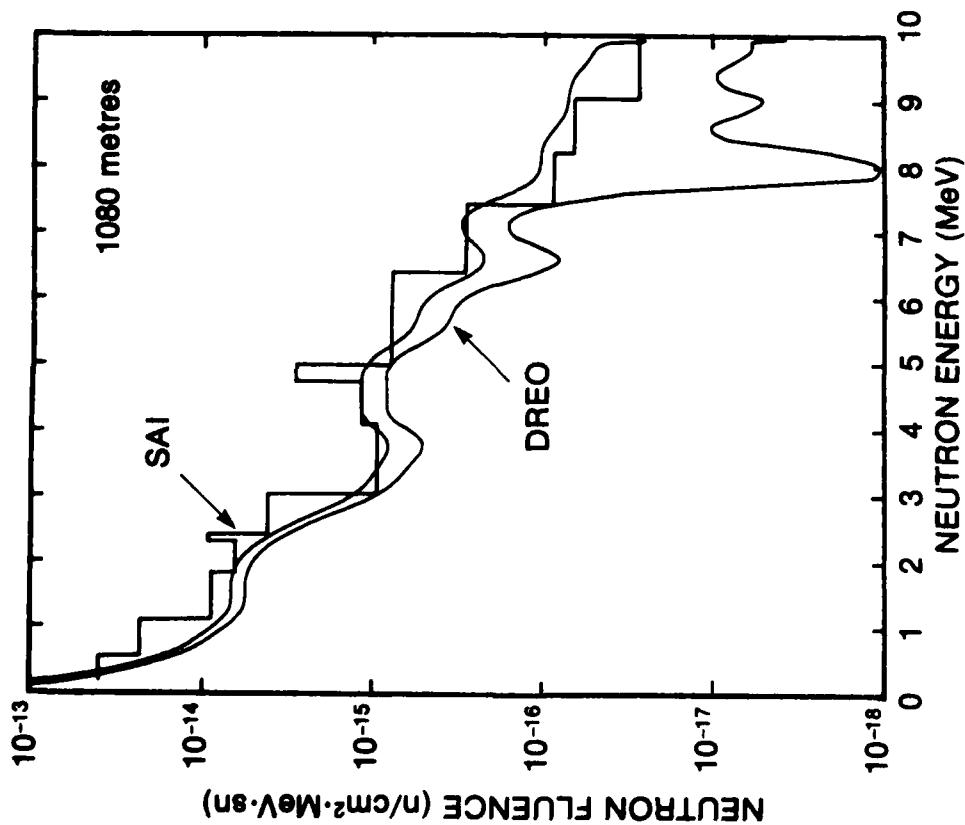
Figure 21 - Comparison of SAI-Calculated and DREO-Measured Neutron Spectra at 1080 Meters
