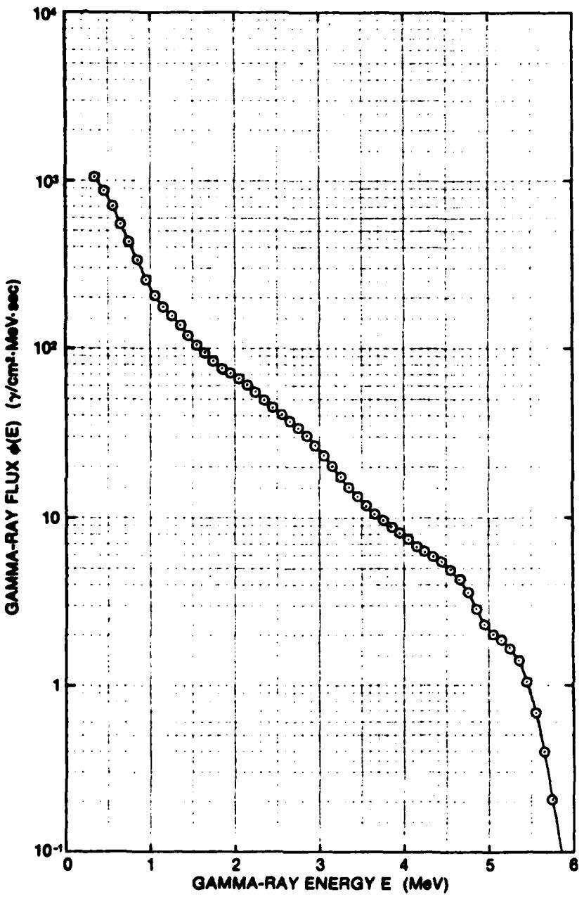
Figure J-2: Gamma-Ray Spectrum Recorded by DREO One Meter from the APRD Cf<sup>252</sup> Source
