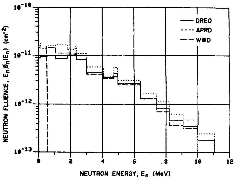
Figure 4 - Measured Neutron Spectra at a Ground Range of 300 Meters
