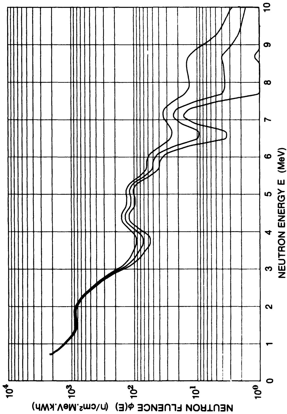
Figure A-9: Free-Field Neutron Spectrum Obtained
