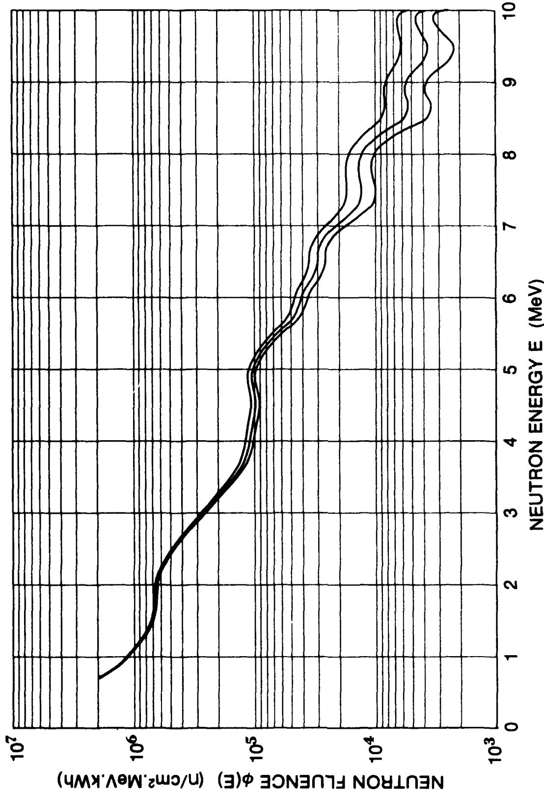
Figure A-6: Free-Field Neutron Spectrum Obtained
