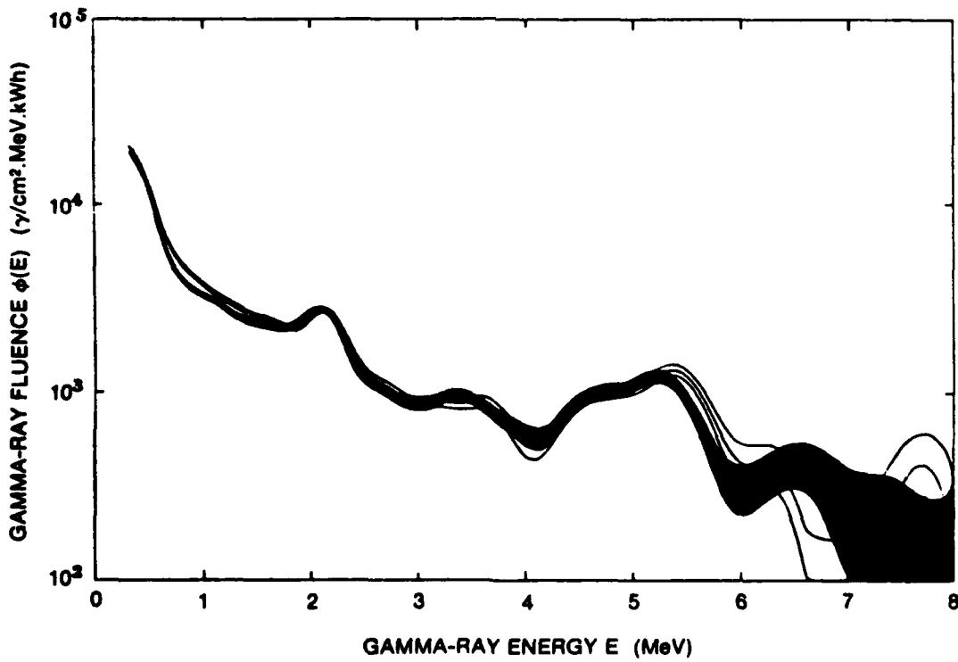
Figure 11 - Gamma-Ray Spectrum Measured in 1982 at 1080 Meters (Open)
