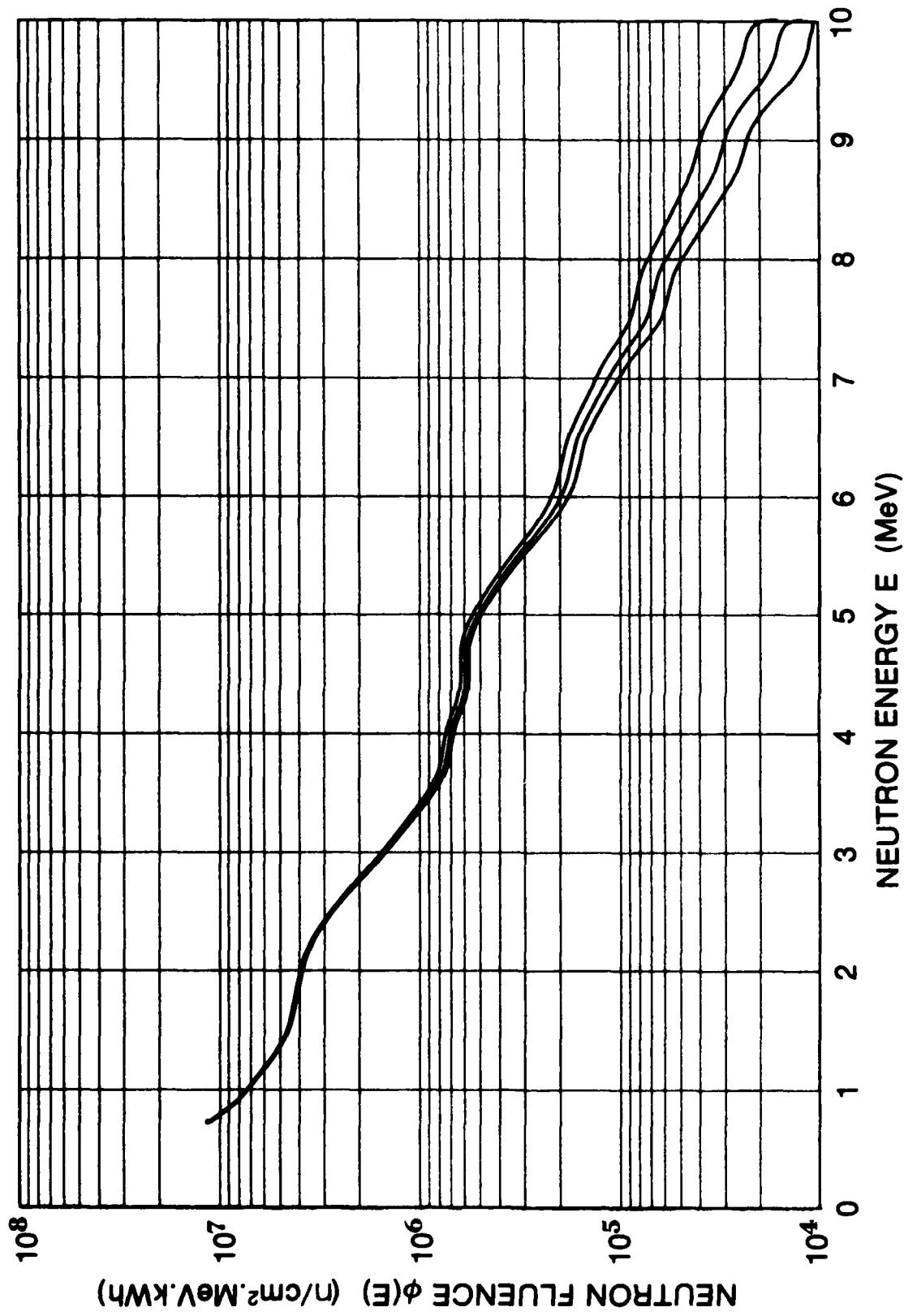
Figure A-4: Free-Field Neutron Spectrum Obtained
