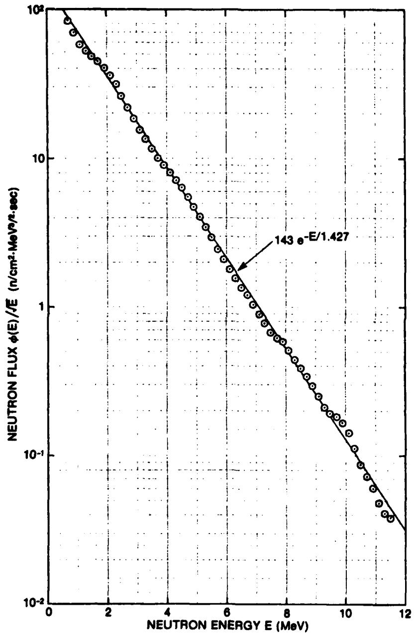
Figure J-1: Neutron Spectrum Recorded by DREO One Meter from the APRD Cf<sup>252</sup> Source
