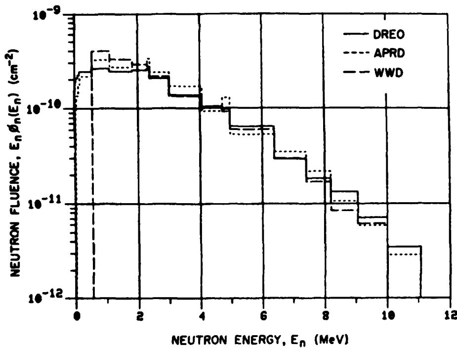
Figure 2 - Measured Neutron Spectra at a Ground Range of 100 Meters
