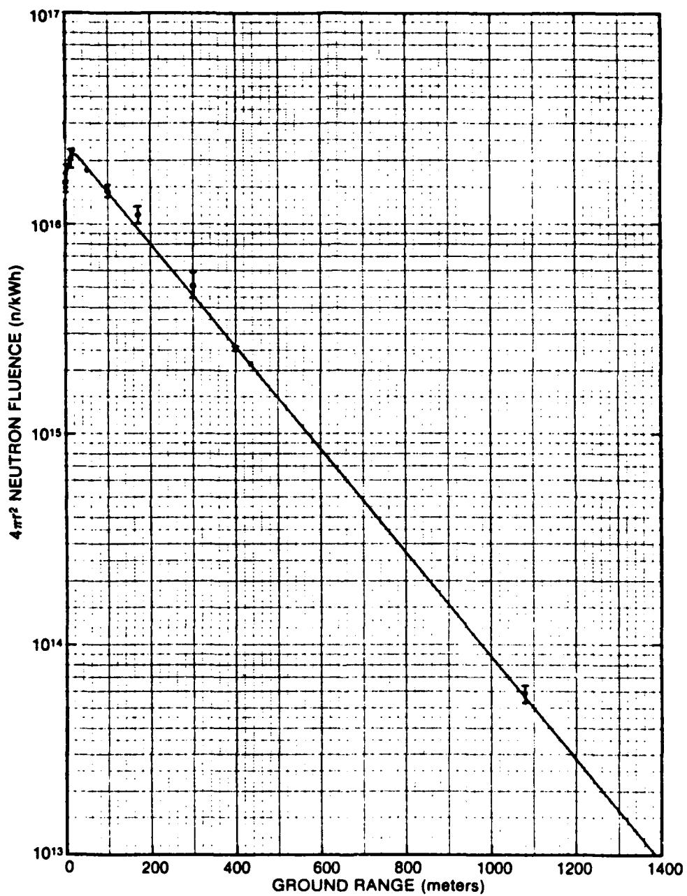
Figure 12 - Measured Variation of Neutron Fluence above 3 MeV with Increasing Ground Range
