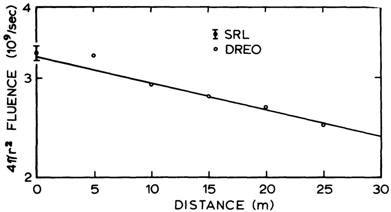
Figure J-4: Comparison of DREO Measurement to SRL Calibration of the Neutron Emission Rate ( $> 600$  keV) from a Californium-252 Source
