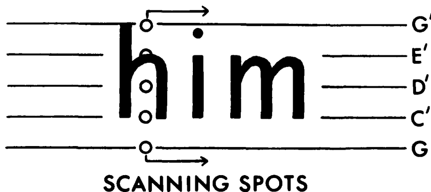
FIGURE 1 Tone generating method of the black-reading Optophone.
