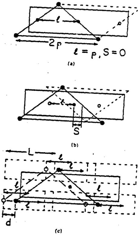
Figure 6: Effect on stability margin of shortening stroke
