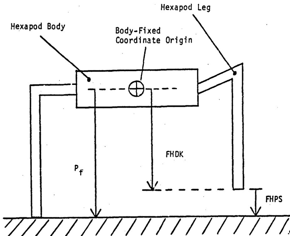
FHPS: Foot Height as measured by Proximity Sensor
