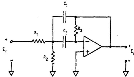
$$\frac{E_o(s)}{E_i(s)} = \left\{ \frac{-\left(\frac{1}{R_1 C_1}\right)s}{s^2 + \left(\frac{C_1 + C_2}{R_3 C_1 C_2}\right)s + \left(\frac{R_1 + R_2}{R_1 R_2 R_3 C_1 C_2}\right)} \right\} = \frac{-H_0 \alpha \omega_0 s}{s^2 + \alpha \omega_0 s + \omega_0^2}$$
