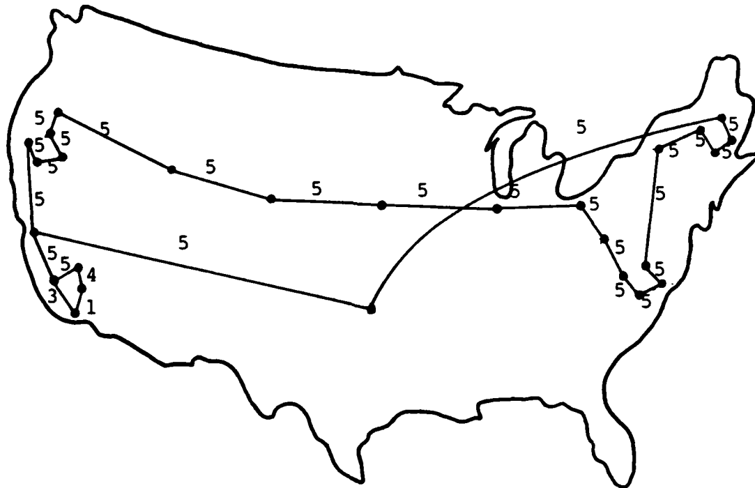
Figure 34. Starting topology for 52-node network
