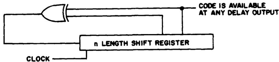
Figure 4. Maximal Length Code Generator
