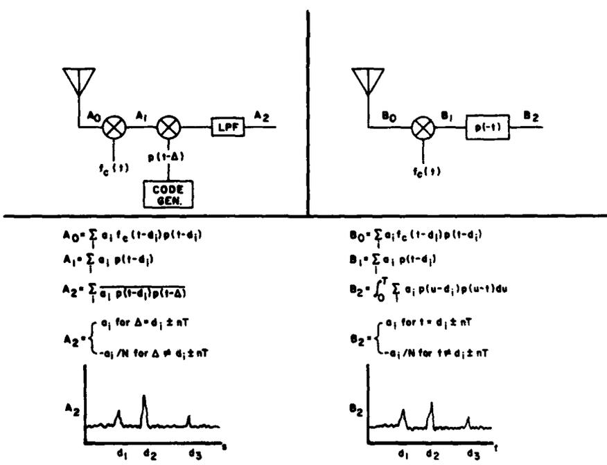
Figure 6b. Receiver Processing Options
