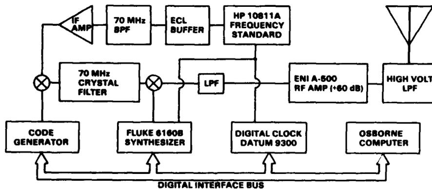
Figure 8. Wideband Channel Probe Transmitter
