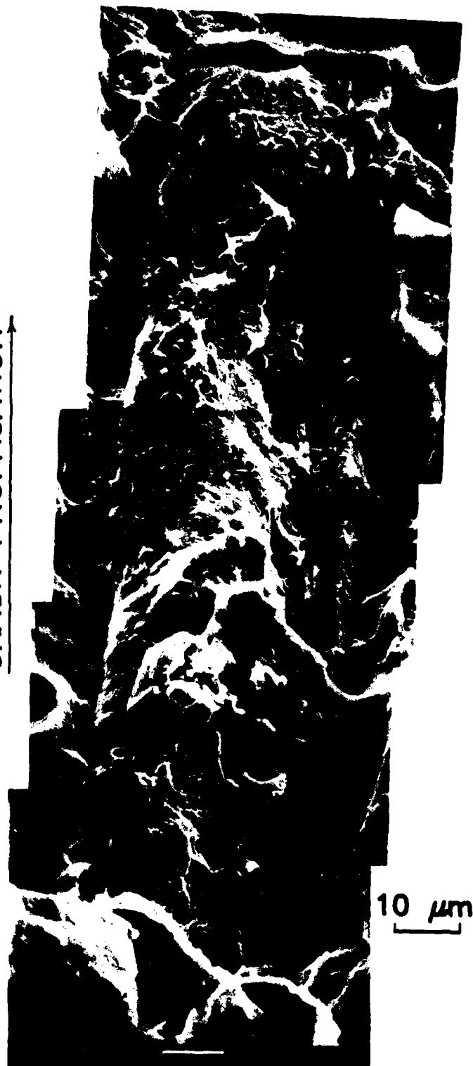
FIGURE (46) HIGH MAGNIFICATION FRACTOGRAPH TAKEN FROM A 2219-T851 (T-L) CT SPECIMEN SHOWING EVIDENCE OF GRAIN-BOUNDARY CAVITATION ( K_{MAX} = 20 MPa√m, T = 175 °C) .
