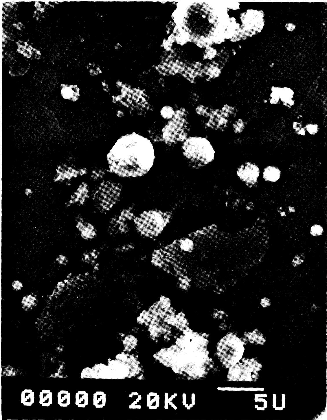
Figure 18. SEM Photograph of Cleaned Exhaust Products.
