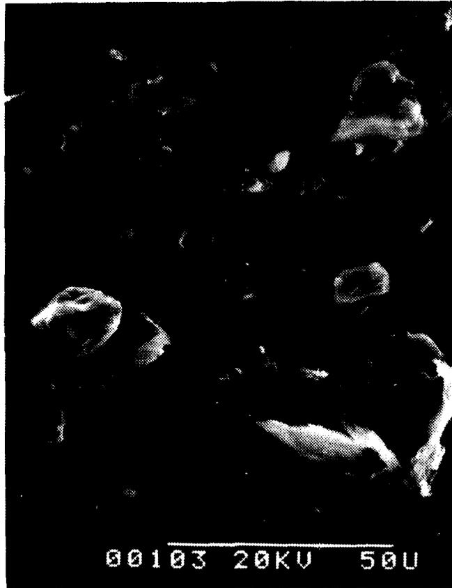
Figure 19. SEM Photograph of Uncleaned Exhaust Products.
