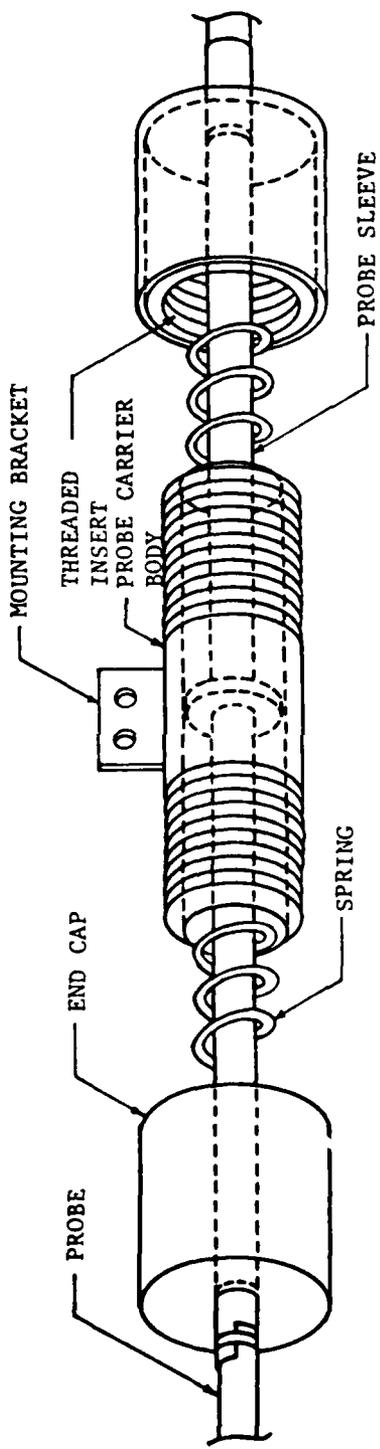
Figure 1. Schematic diagram of spring-loaded in-situ probe holder.
