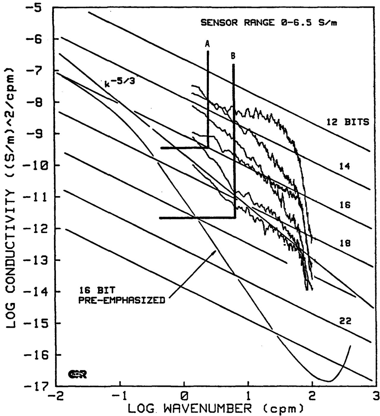
Fig. 6 - Conductivity spectrum, with various sensor noise levels
