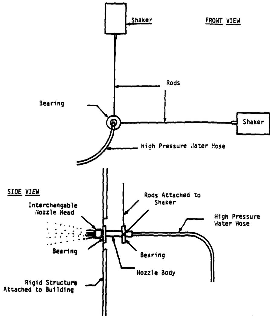
Figure 2. Sketch of Vibrating Nozzle Hardware.
