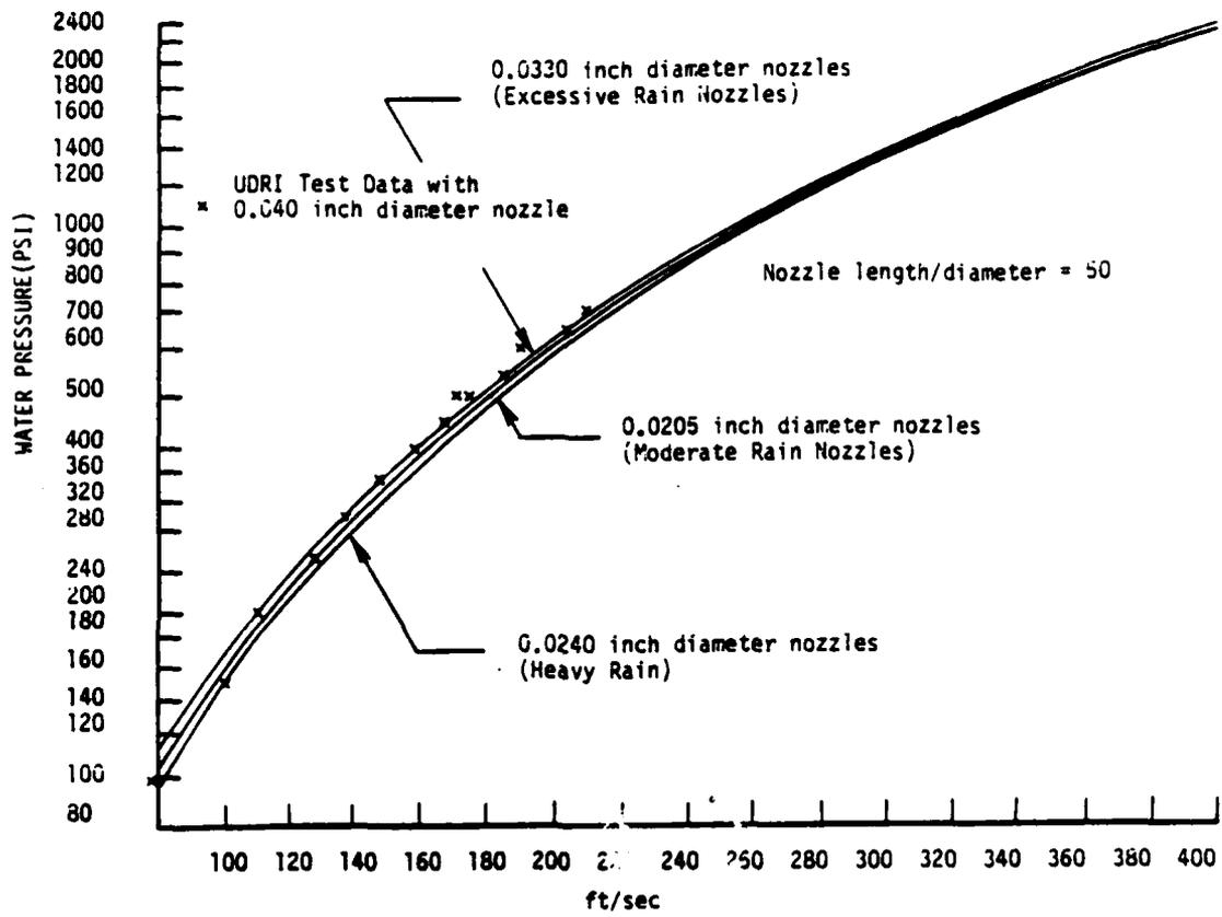
Figure 3. Water Pressure vs. Exit Velocity for Various Nozzles from Melene<sup>1</sup>. X's are UDRI Test Data with .040 inch Diameter Nozzle.
