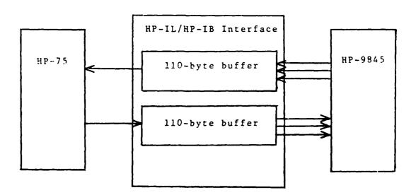
Figure 2. How data is transferred between the 9845 and the 75 through the HP-IL/HP-IB interface.
