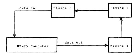
Figure 1. The HP-IL serial-loop system
