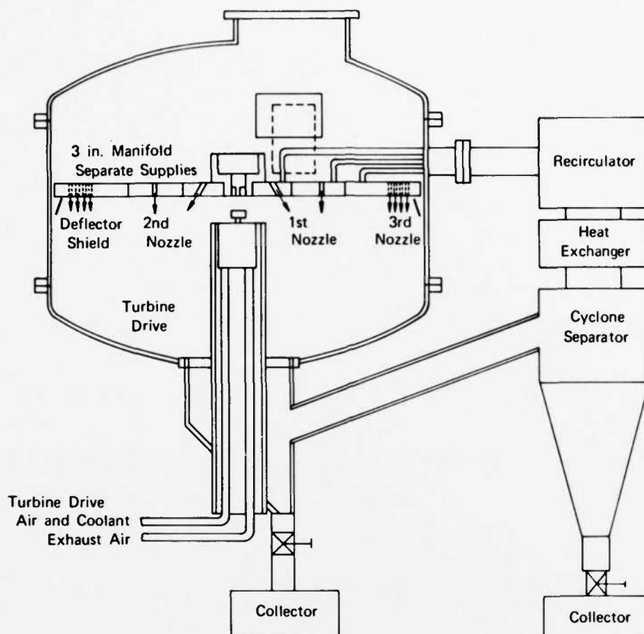
Figure 3. Experimental Powder Rig
