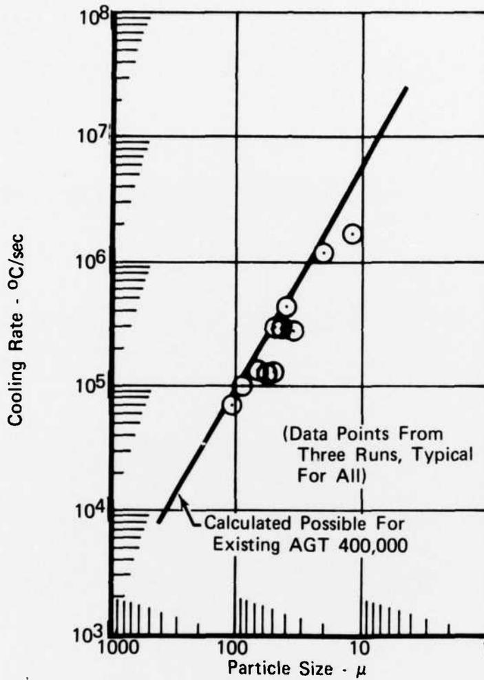
Figure 25. Experimentally Determined Cooling Rates
