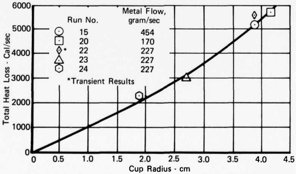
Figure 11. Liquid Metal Heat Losses to Skull-Forming Atomizers, 10,000-16,000 rpm FD 98338
