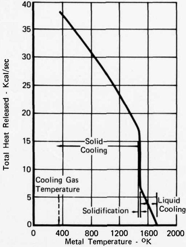
Figure 15. Total Heat Rejected to Helium Atmosphere at 350°K (151.2 grams/sec Superheated Liquid IN100)
