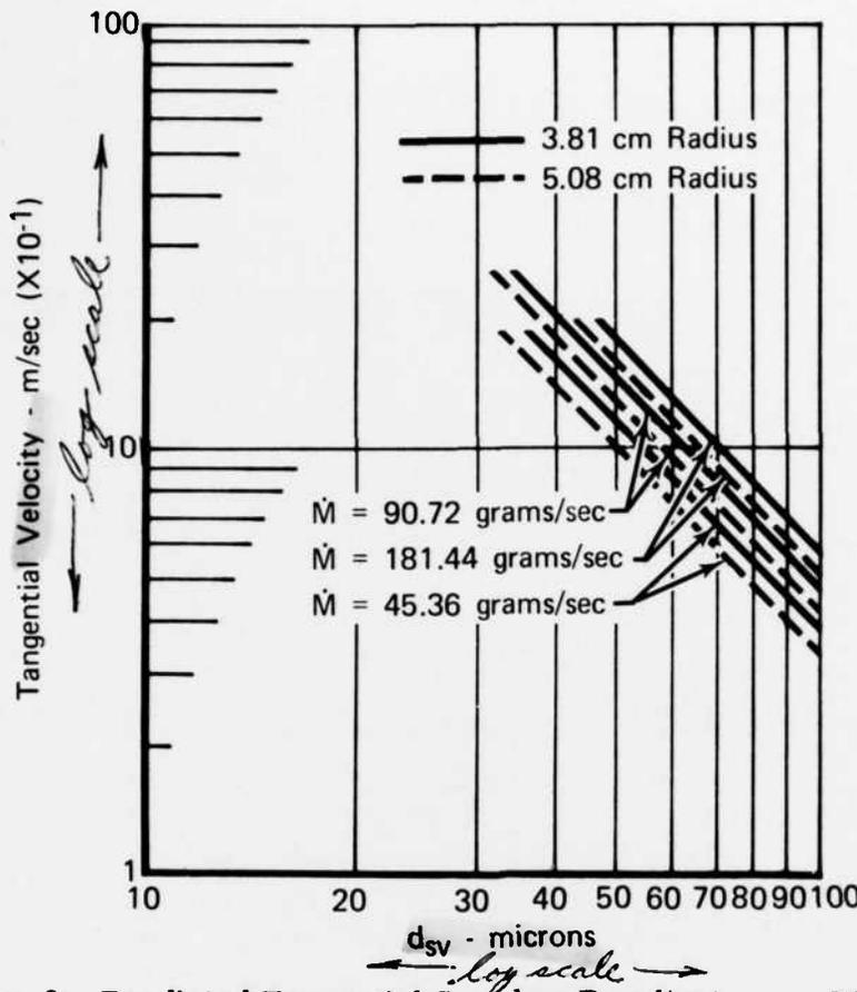
Figure 2. Predicted Tangential Speed vs Resultant Particle Size for IN100-Type Material FD 98316
