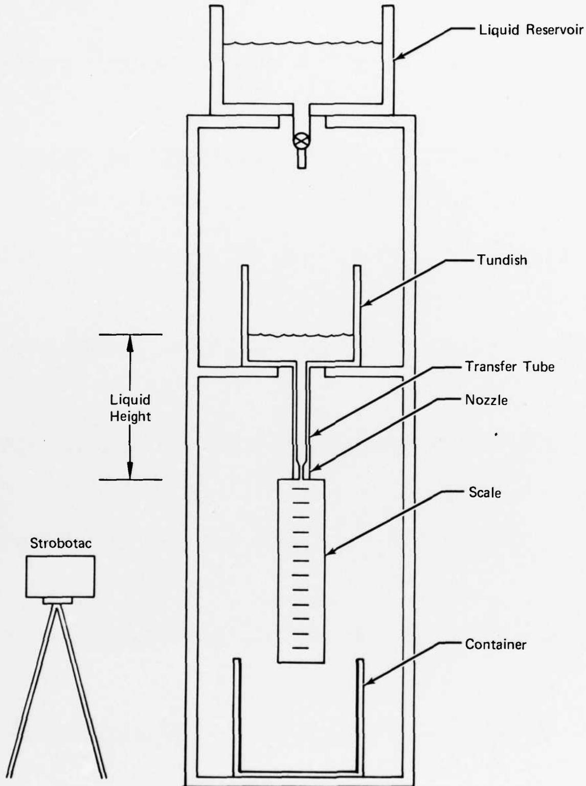
Figure 6. Schematic of Apparatus to Measure
