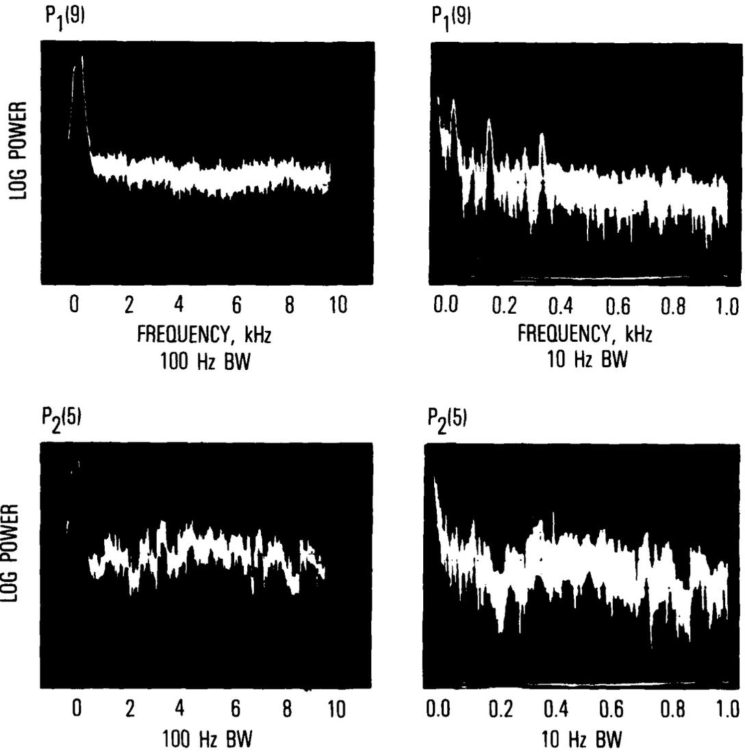
Fig. 4. Power Spectral Analysis of Two of the Signals Shown in Fig. 3. The scan rate was 5 sec/division and the measurement bandwidth is indicated.
