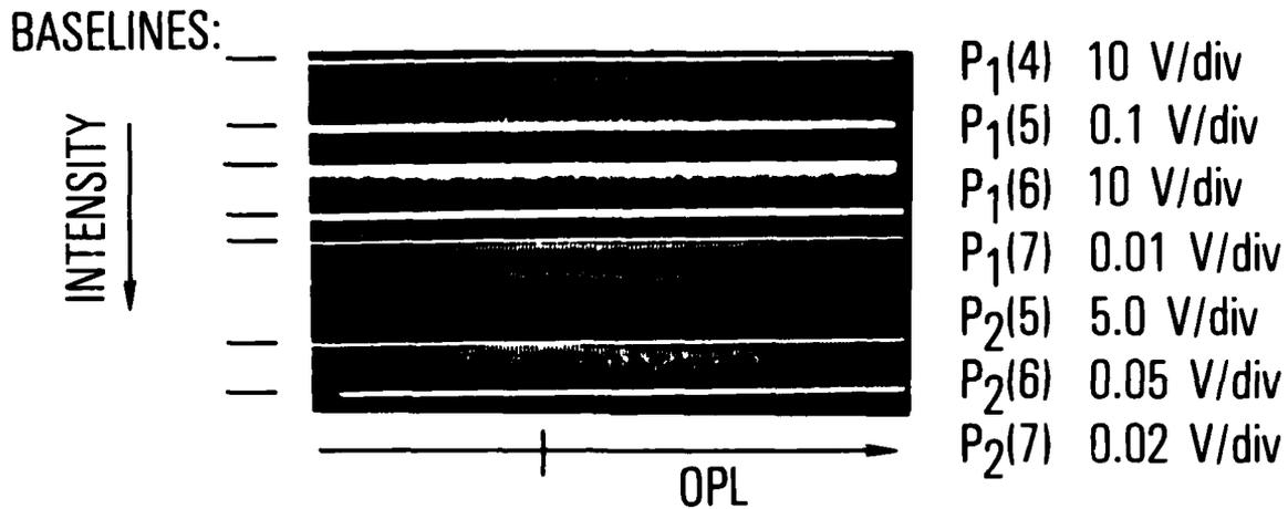
Fig. 6. Single-Line Fringe Scans of a Mach-Zehnder Interferometer without Gain in Either Arm.
