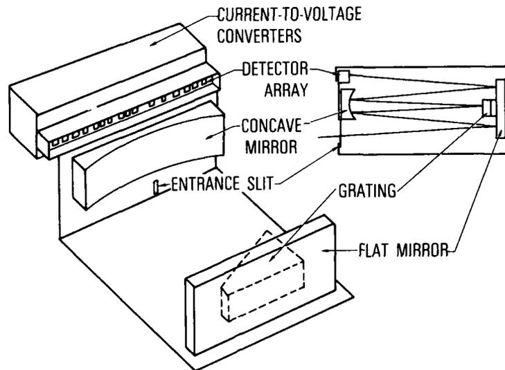
Fig. 1. Spectrometer Optical Layout
