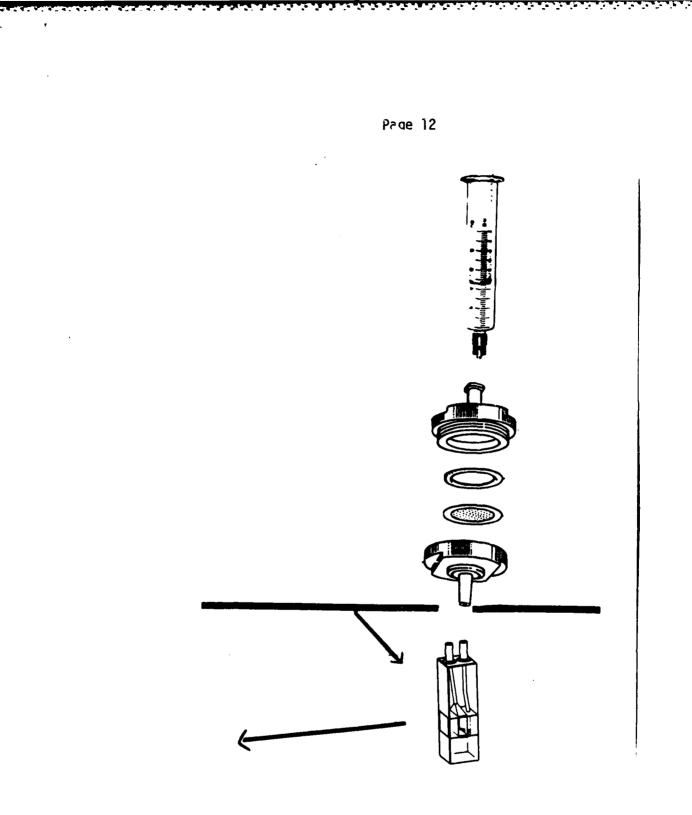
Fig. 2: A sketch of the flow-filtration apparatus for the rapid determination of the rate of 2-aminopurine efflux. The suspension of preloaded cells is placed in a syringe barrel connected to a holder for a 5.0 micron membrane filter. The efflux buffer is drained through a quartz flow cell with medical plastic tubing. The excitation light enters the cell from the rear and the emission light is detected at a right angle.
