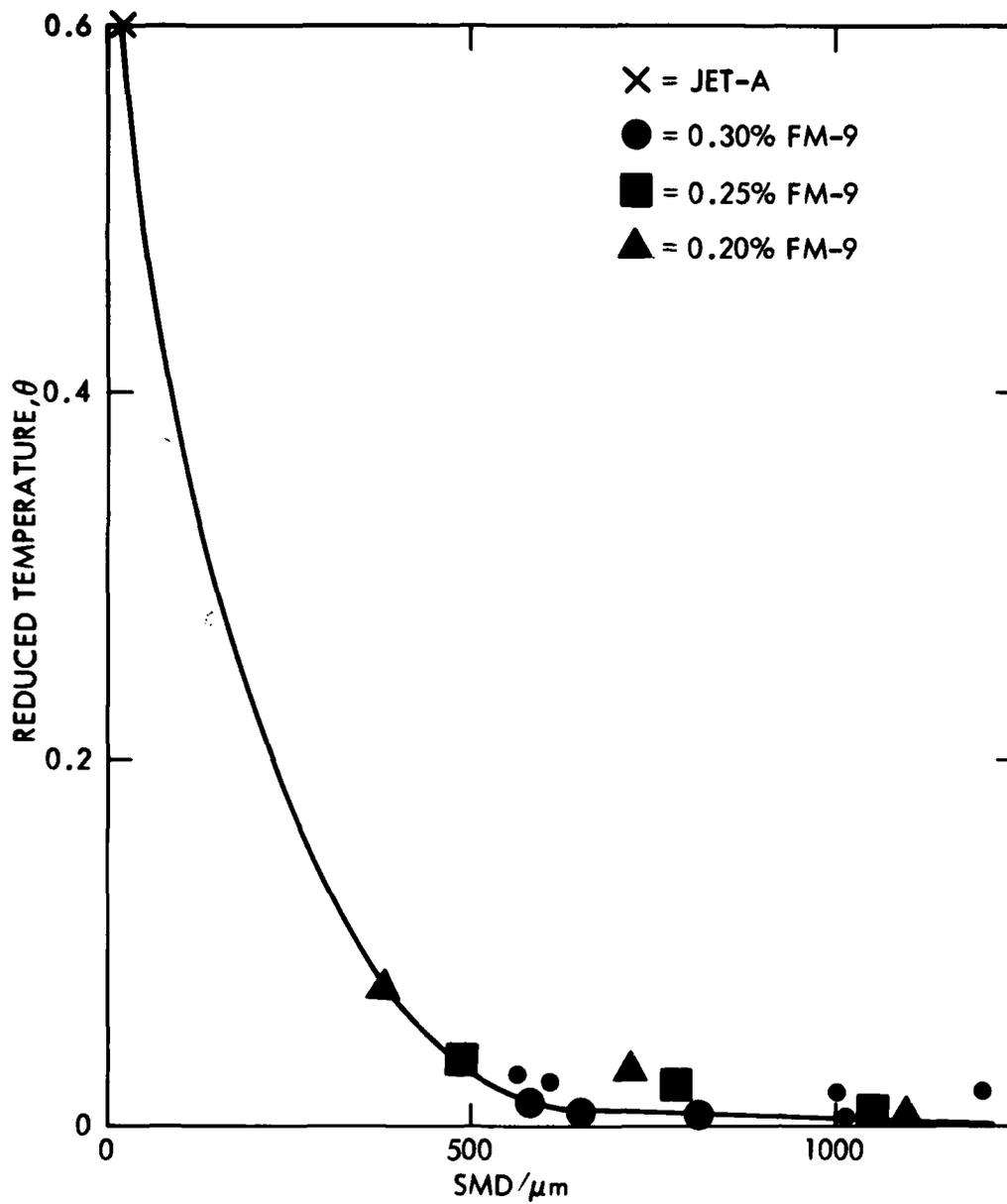
Figure 2-5. Flammability as a Function of Fuel Atomization. SMD values computed with a maximum diameter of 2000  $\mu\text{m}$
