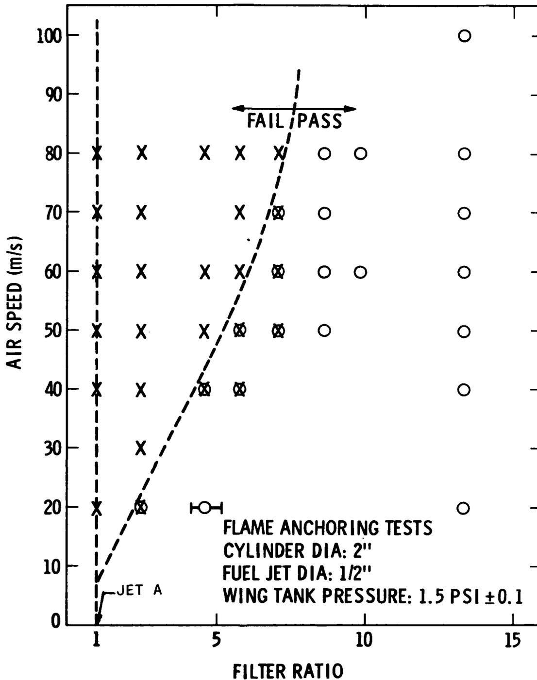
Figure 3-5 Pass/Fail Boundary for Degraded AMK(0.3 percent FM-9) in Cylinder Flame Anchoring Experiments. Ignition Source: Acetylene-Air Flame, 8.8 KW
