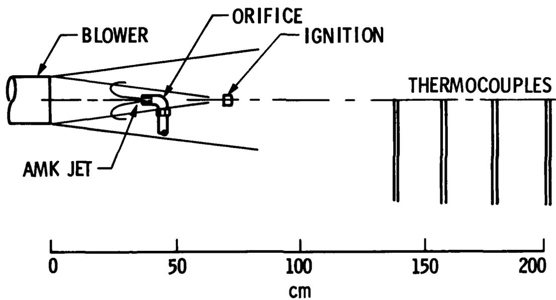
Figure 2-1. Mini Wing Shear Apparatus for Flammability Measurement
