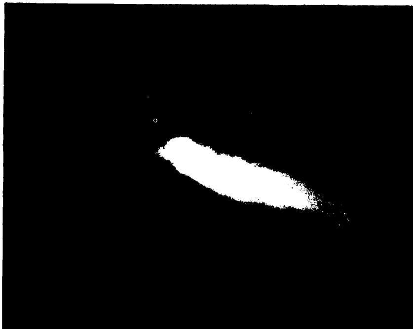
Figure 3-4. Flame Anchoring at  $U_{\infty} = 50$  m/s,  $FR = 4.65$
