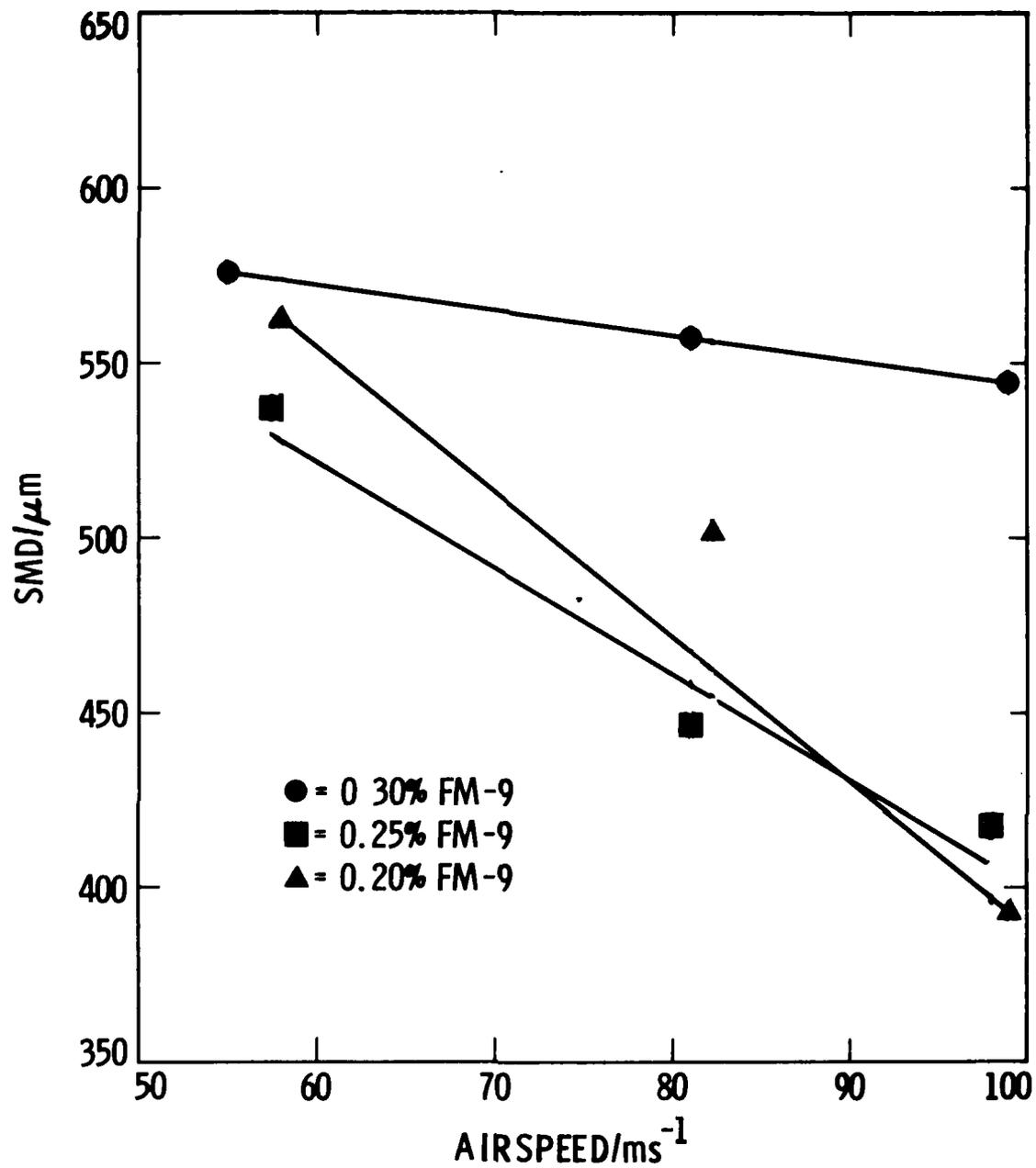
Figure 2-4. Fuel Atomization as a Function of Shearing Airspeed. SMD values computed with a maximum diameter of 1000 μm
