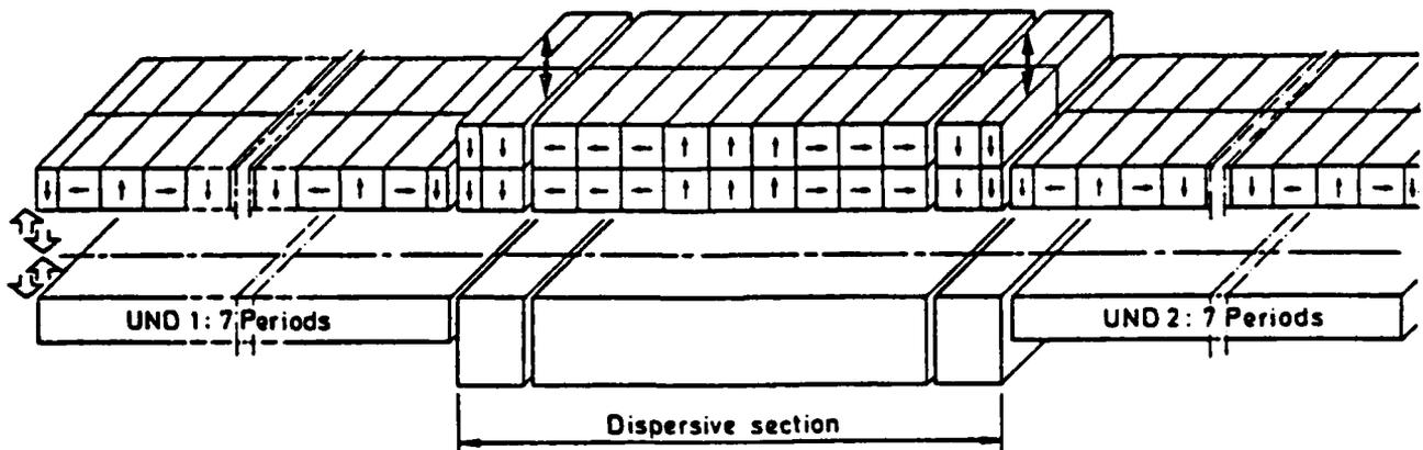
Figure 1 - Optical klystron magnet configuration.
