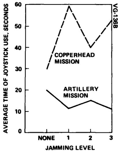
Figure 34. Jamming level effects on average joystick use time.
