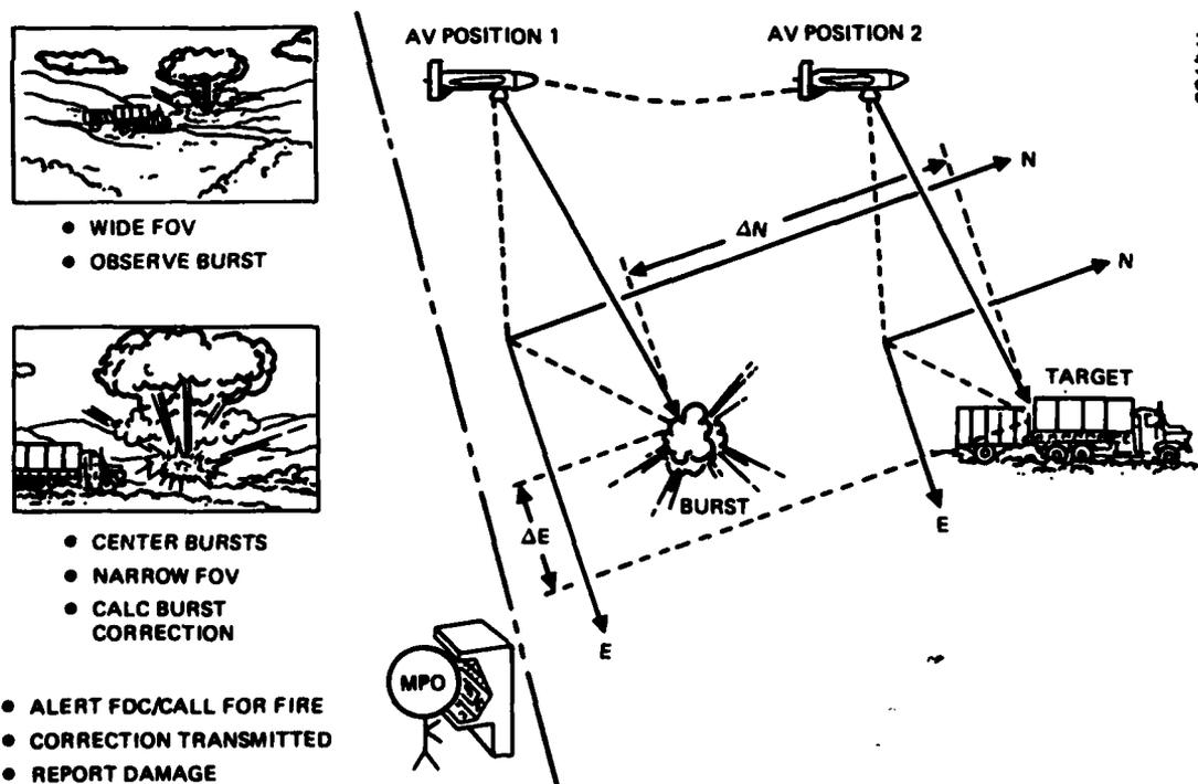
Figure 4. Artillery burst correction operation.
