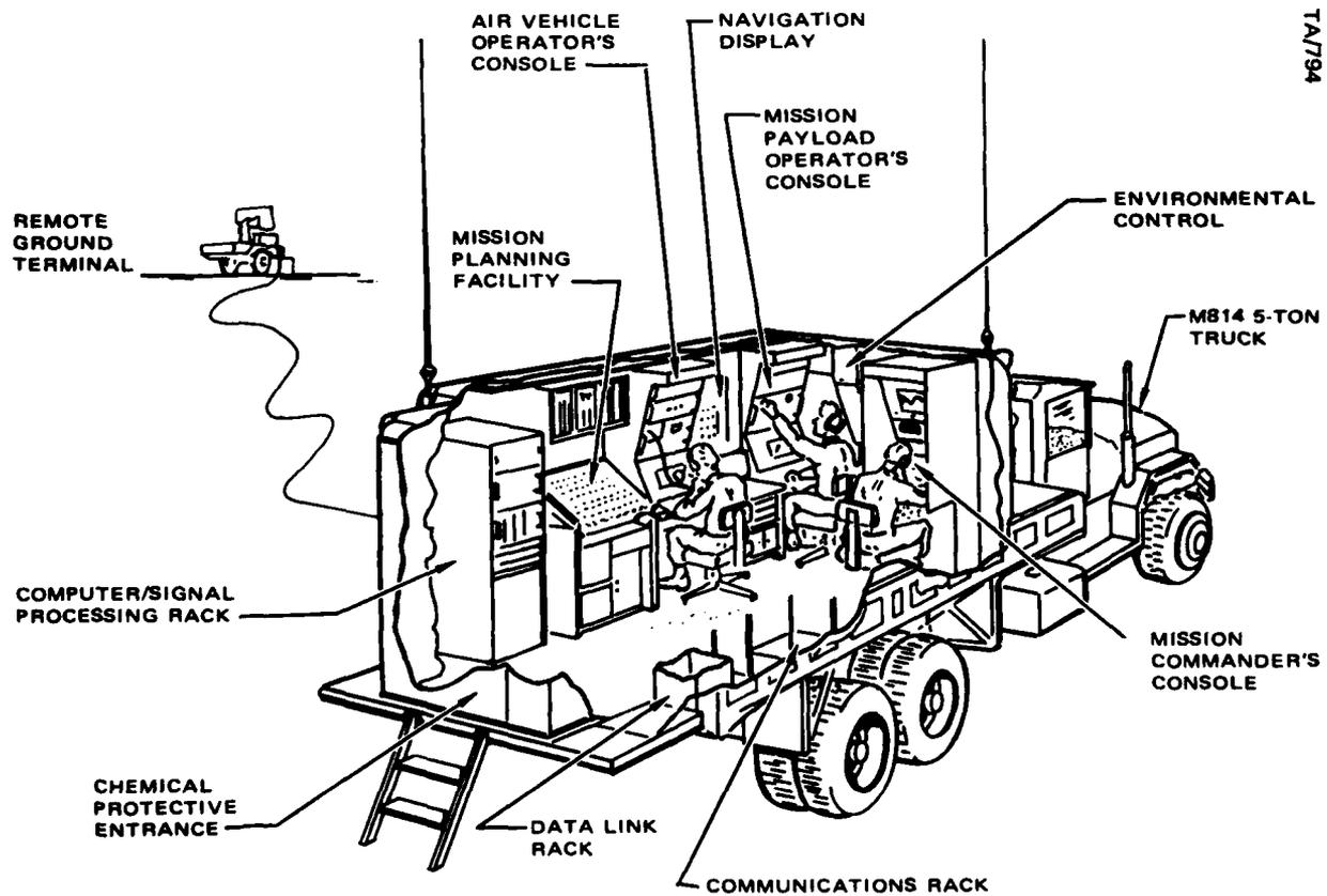
Figure 2. RPV ground control station.
