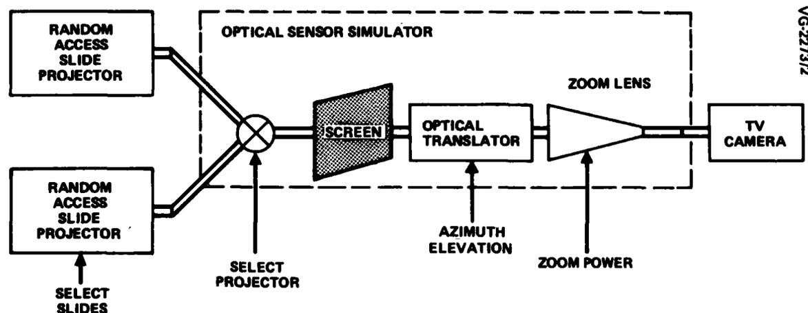
Figure 10. Sensor simulation equipment block diagram.
